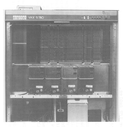
Figure 3-1 VAX-11/780 Standard Configuration (Front View)
