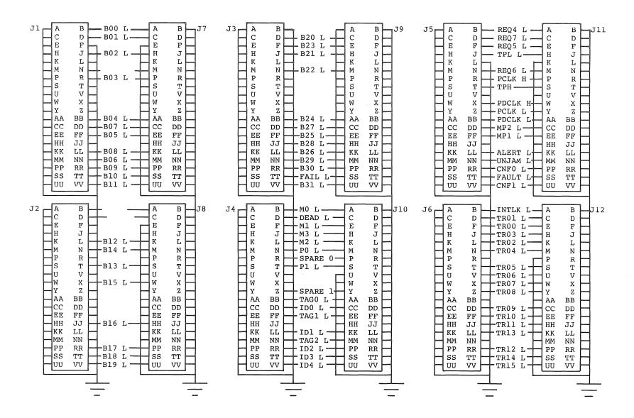
Figure 2-4. SBI Signal Names and Pin Assignments
