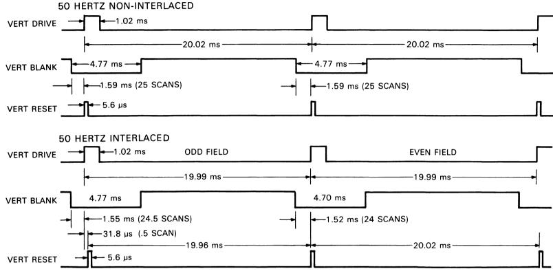
Figure 4-6-13 Vertical Signals - 50 Hz
