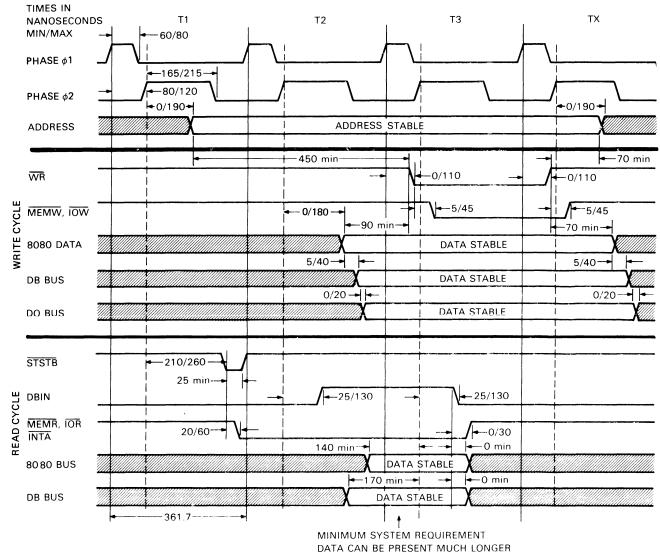
Figure 4-2-3 Microprocessor Bus Timing
