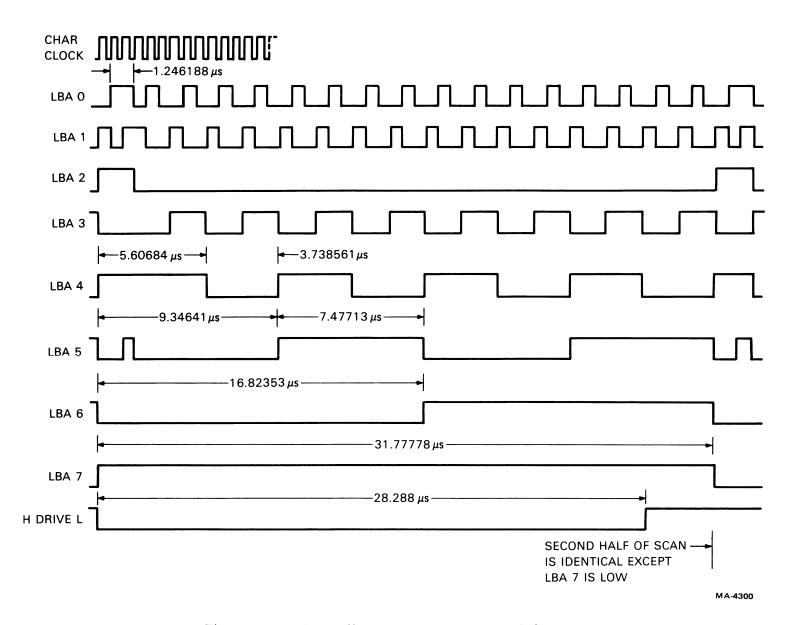
Figure 4-6-10 Line Buffer Address Outputs - 80 Column
