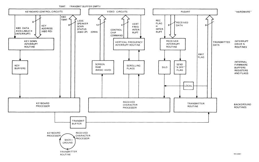
Figure 4-1-3 VT100 Firmware Block Diagram
