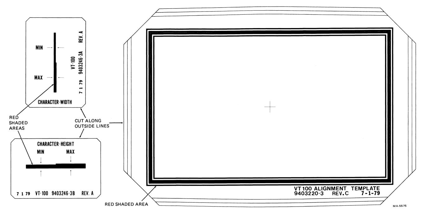
Figure 5-1 Video Alignment Templates
