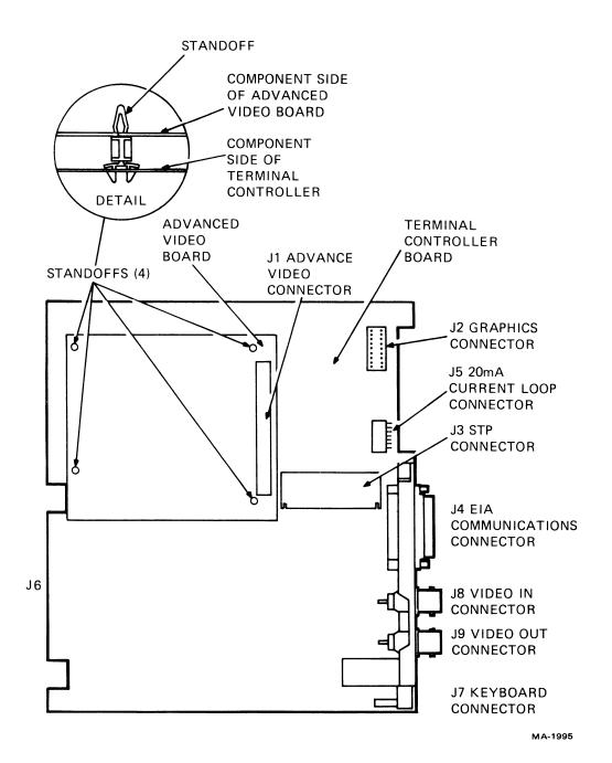
Figure 5-9 Terminal Controller with AVO
