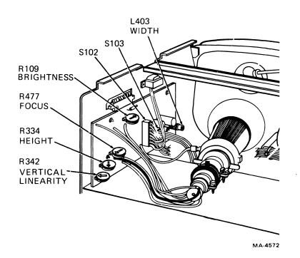
Figure 5-4 Elston Video Monitor Board Adjustments
