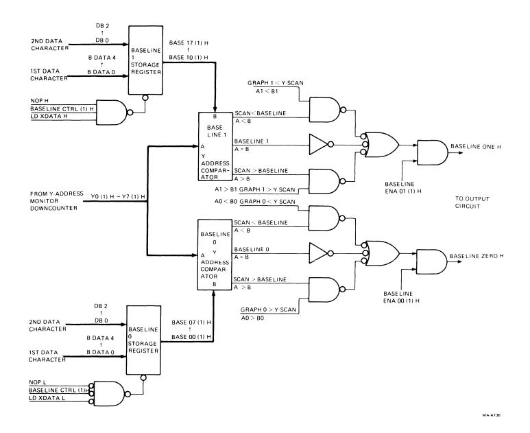
Figure 6-25 Baseline (Shade Line) Registers and Comparators
