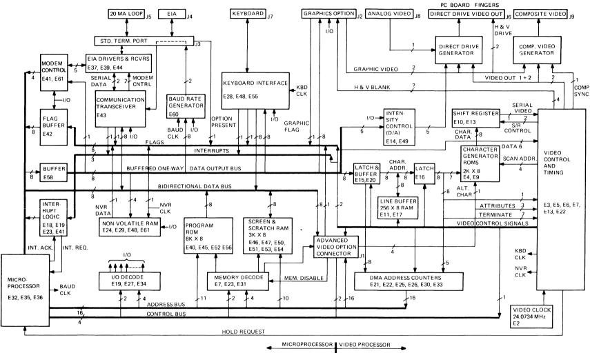
Figure 4-6-1 Video Processor Block Diagram
