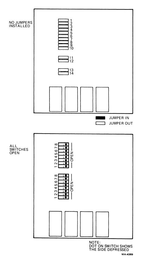
Figure 5-21 Advanced Video Board VT100 Configuration
