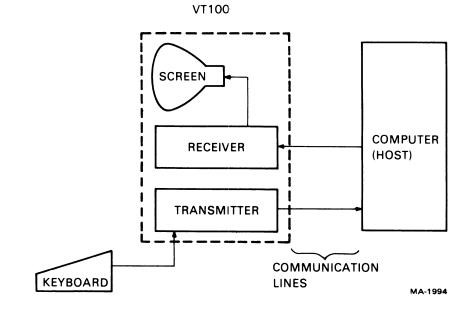
Figure A-1 Terminal Data Flow
