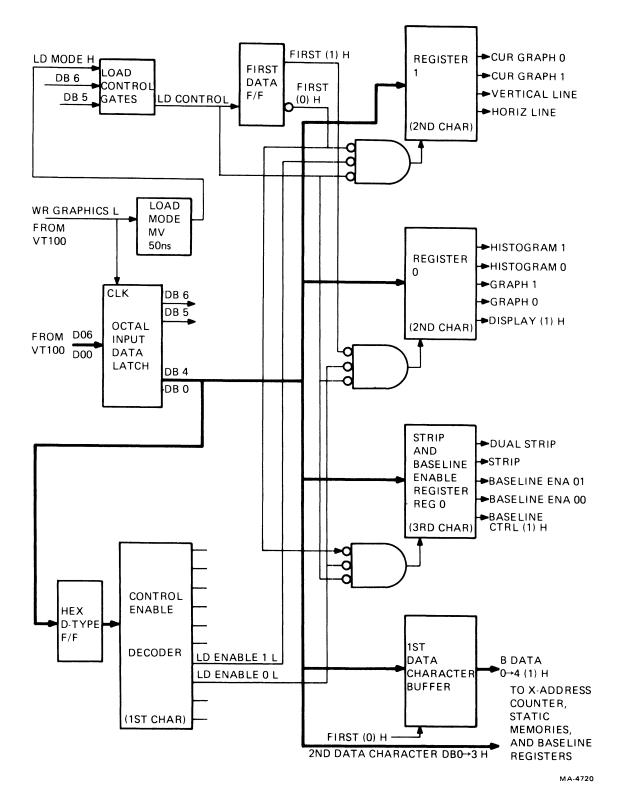
Figure 6-18 Loading the Registers
