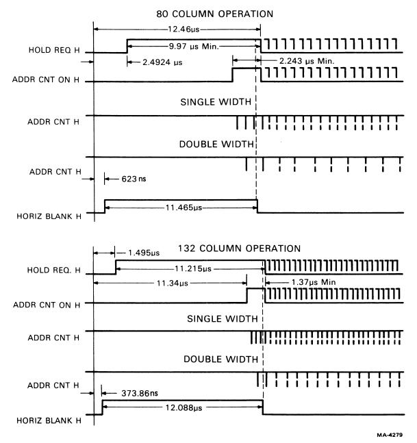
Figure 4-6-8 Address Count Timing
