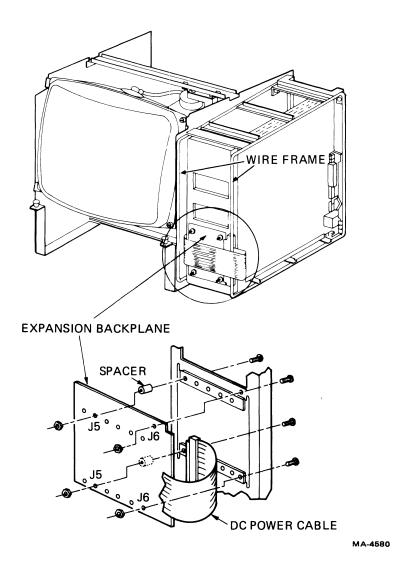
Figure 5-18 VT105 Expansion Backplane Removal
