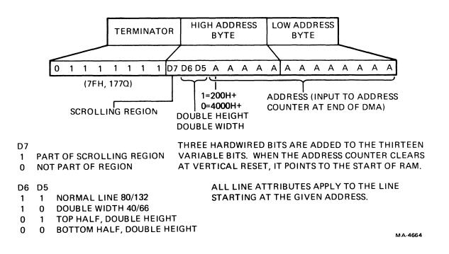
Figure 4-7-2 Terminator and Address Bytes
