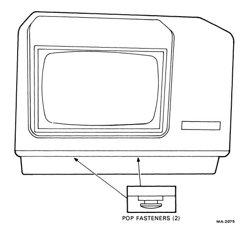
Figure 5-11a Top Cover Removal (Front View)
