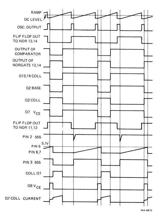
Figure 4-9-3 Power Supply Timing Diagram
