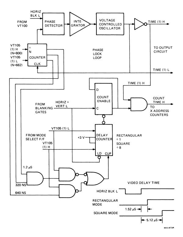
Figure 6-17 Phase Lock Loop Timing
