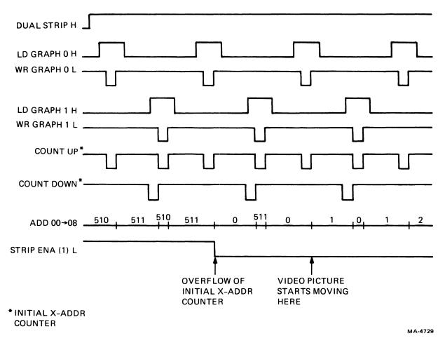
Figure 6-30 Dual Strip Chart Timing Diagram
