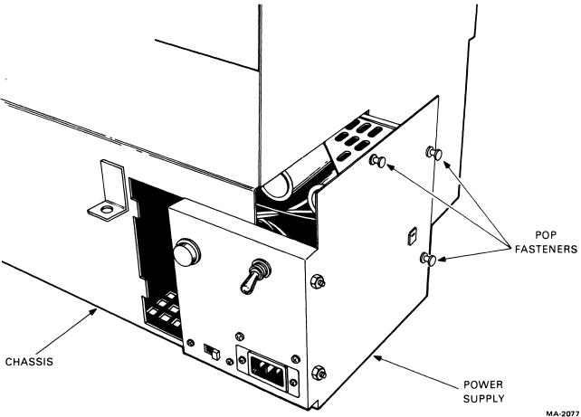
Figure 5-15 Power Supply Removal
