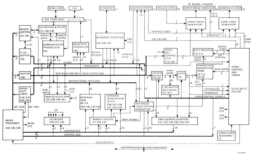
Figure 4-2-2 Microprocessor Block Diagram
