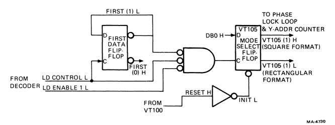
Figure 6-16 Selecting Mode of Operation
