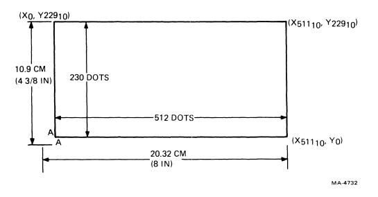
Figure 6-14 Rectangular Aspect Ratio Graph Drawing Field
