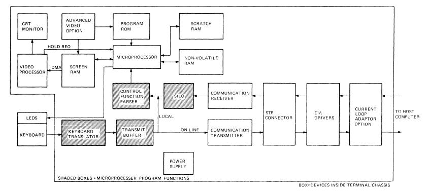
Figure 4-1-2 Functional Block Diagram
