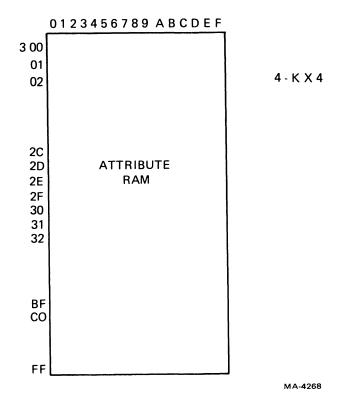
Figure 4-7-3 Screen RAM Organization – 80 Column, 60 Hz (Sheet 1 of 2)
