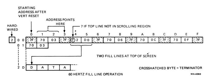
Figure 4-7-5 Fill Line Operation – 60 Hz
