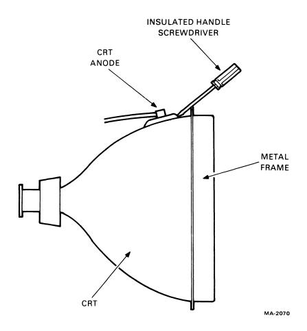
Figure 5-13 CRT Anode Discharging
