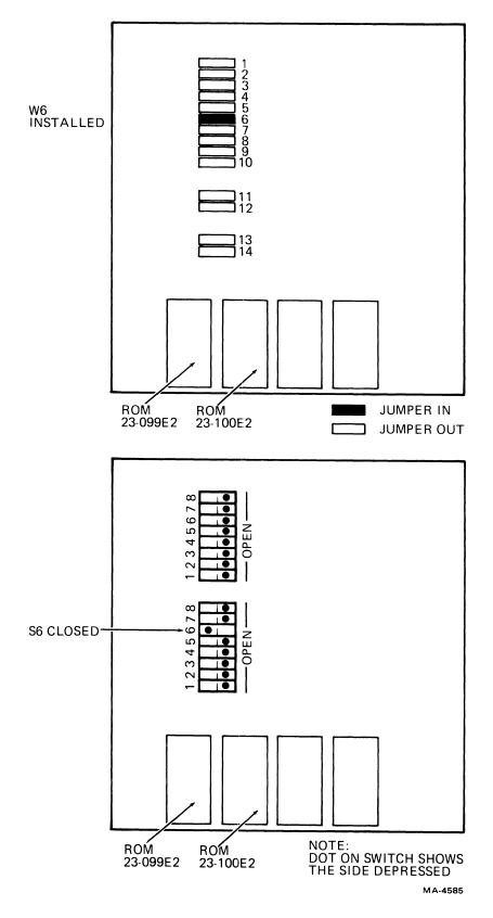
Figure 5-23 Advanced Video Board, VT132 Configuration
