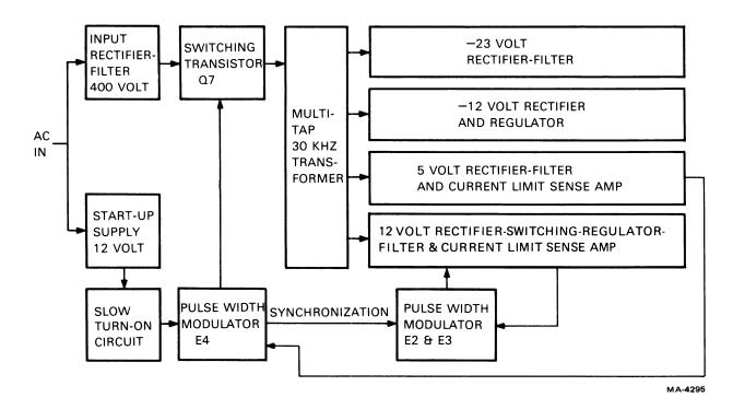
Figure 4-9-1 VT100 Power Supply Block Diagram
