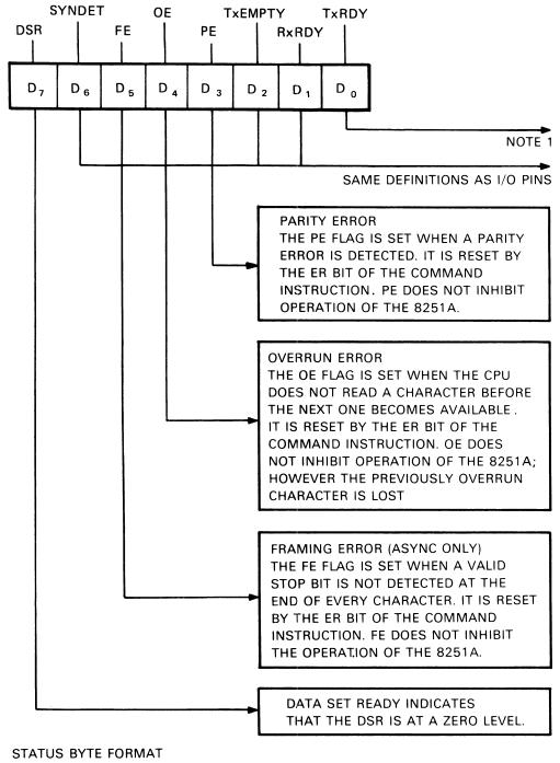
NOTE 1: TxRDY STATUS BIT HAS DIFFERENT MEANINGS FROM THE TxRDY OUTPUT PIN. THE FORMER IS NOT CONDITIONED BY CTS AND TxEN; THE LATTER IS CONDITIONED BY BOTH CTS AND TxEN. i.e. TxRDY STATUS BIT = DB BUFFER EMPTY TxRDY PIN OUT = DB BUFFER EMPTY • (CTS-0) • (TxEN-1) MA-4275
