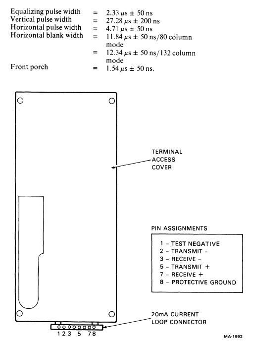
Figure 3-3 20 mA Current Loop Interface
