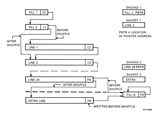
Figure 4-7-9 Full Screen Address Shuffling
