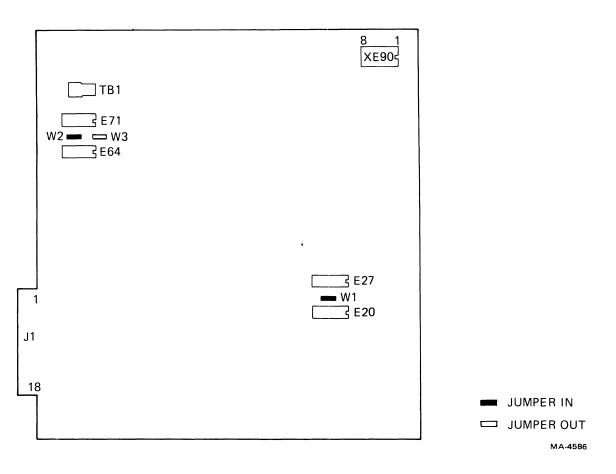
Figure 5-24 VT105 Waveform Generator Board Configuration
