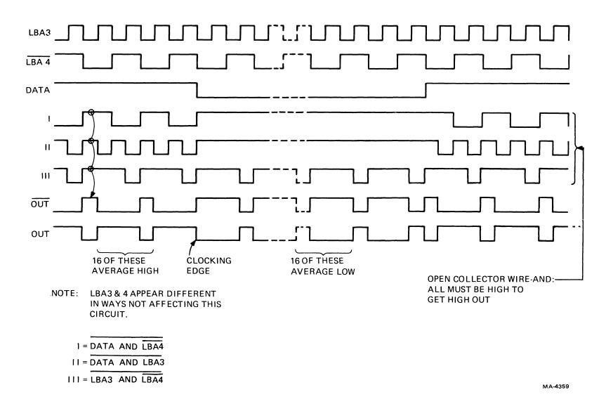
Figure 4-4-6 Encoding of Terminal Data and Clock
