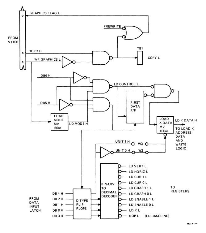
Figure 6-13 Decoding the Control Character
