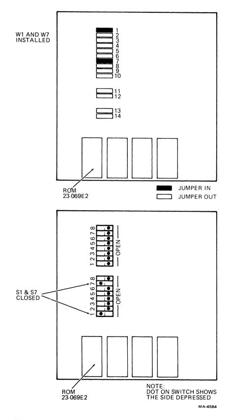
Figure 5-22 Advanced Video Board VT100-WA/WB Configuration
