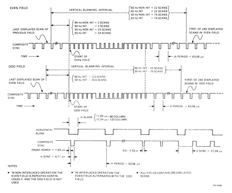
Figure 4-6-14 Composite Sync Output
