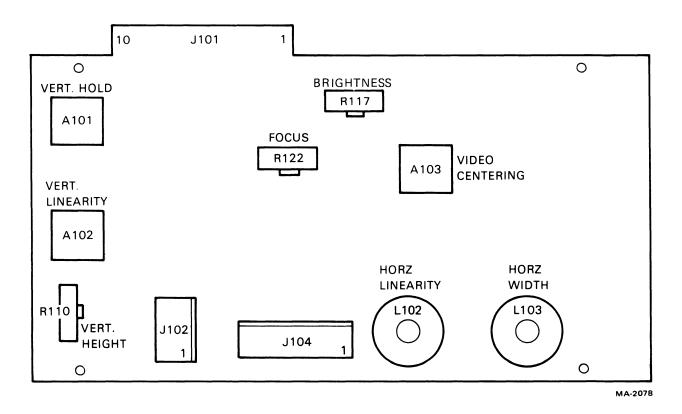
Figure 5-2 Ball Video Monitor Board Adjustments
