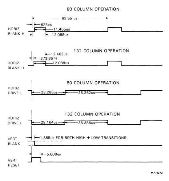
Figure 4-6-9 Horizontal Timing
