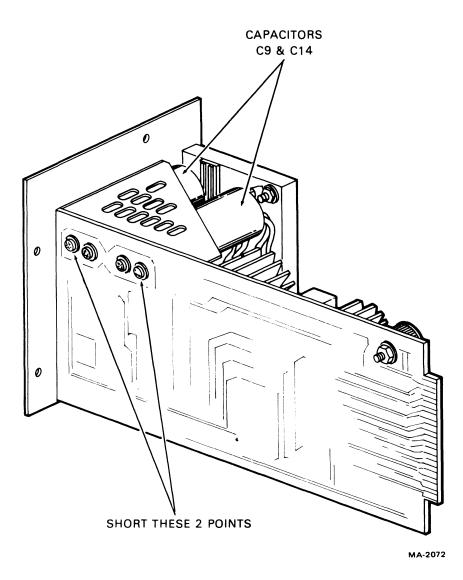
Figure 5-16 Power Supply Capacitor Discharging
