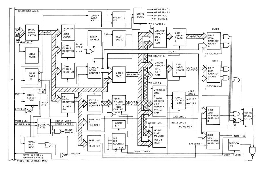
Figure 6-12 M7071 Waveform Generator Block Diagram
