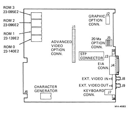
Figure 5-20 Terminal Controller Board, VT132 Configuration
