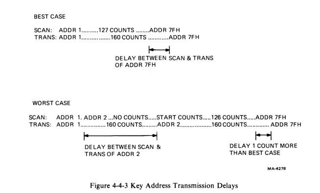
Here is a formula that estimates the delay between the time that the terminal asserts the start scan bit at its UART and the time that the terminal UART asserts data available upon receiving the final address 7FH. The clock driving the address counter and UART has a period of 7.945 microseconds, there is the number of addresses to the first closed key to be counted, and the serial transmission of an address takes 160 clock periods (16 clocks per bit, 8 data bits, 1 start and 1 stop bit).
