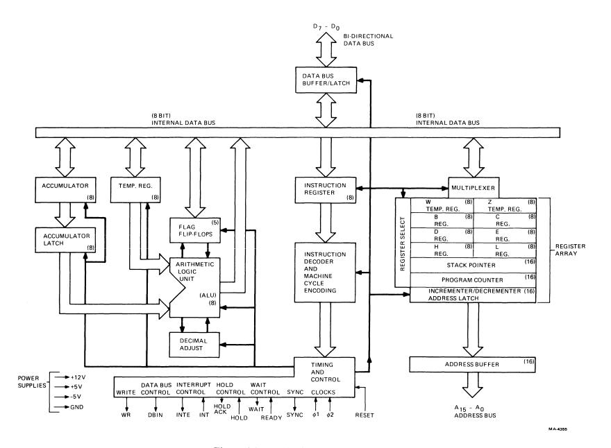
Figure 4-2-1 8080 Block Diagram
