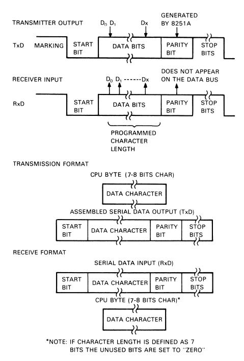
Figure 4-3-2 Asynchronous Data Format
