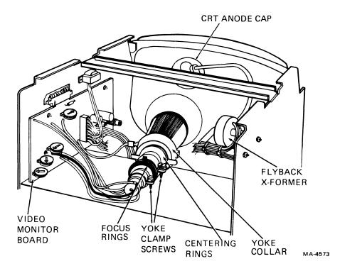
Figure 5-5 Elston Monitor CRT Adjustments
