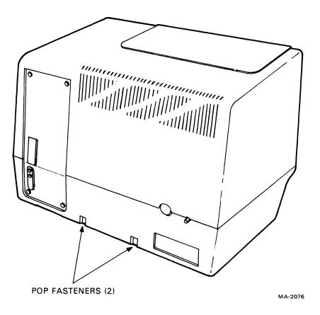
Figure 5-11b Top Cover Removal (Rear View)
