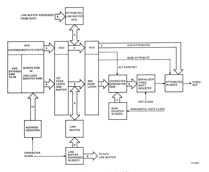
Figure 4-6-3 Video Processor Functional Diagram
