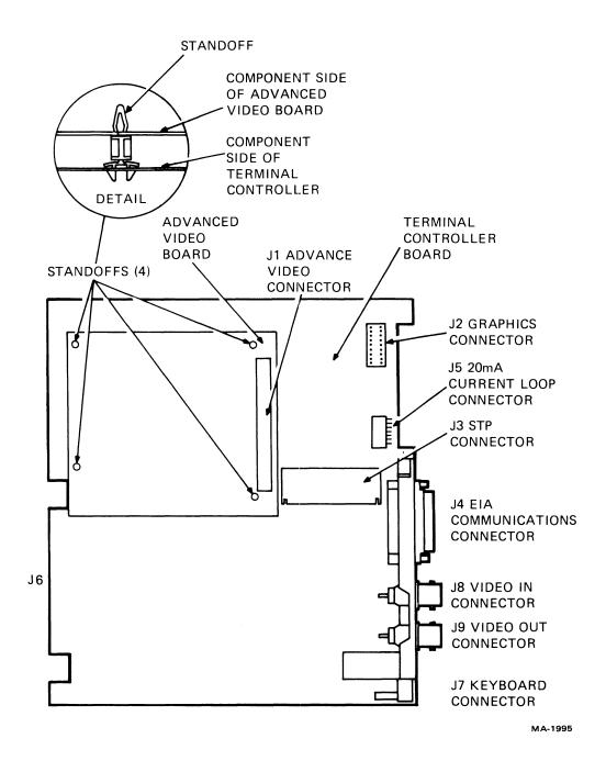
Figure 6-9 Advanced Video Option Installation
