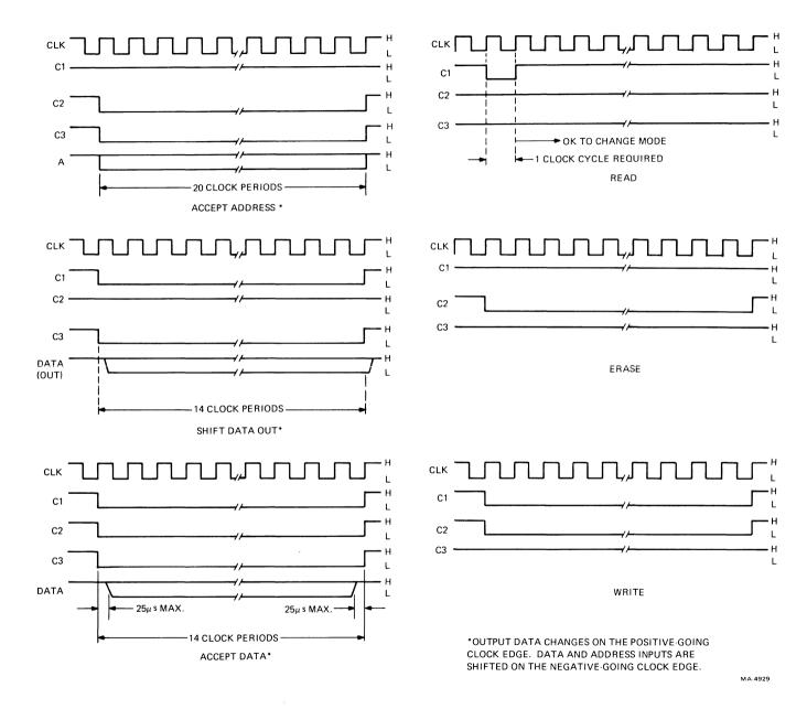
Figure 4-5-3 NVR Timing Diagrams
