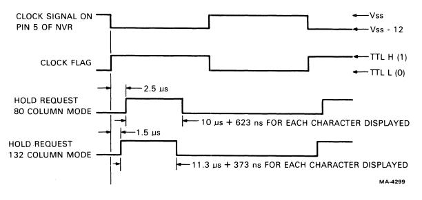
Figure 4-5-2 NVR Signals
