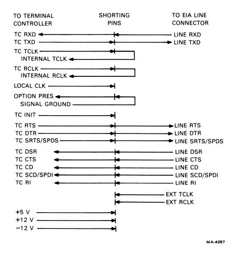
Figure 7-2 STP Signal Lines
