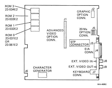
Figure 5-19 Terminal Controller Board VT100 Configuration
