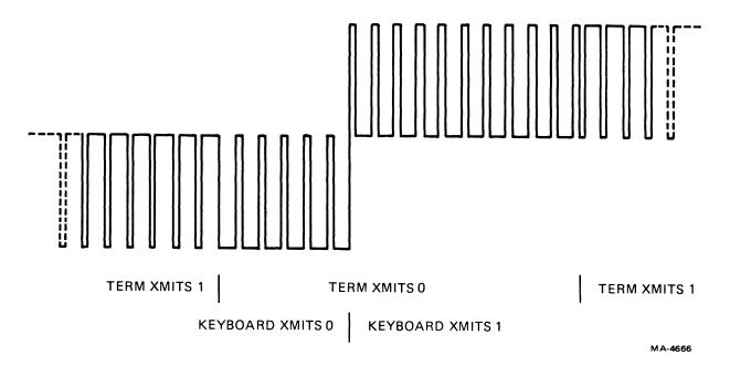
Figure 4-4-8 Keyboard Interface Signal
