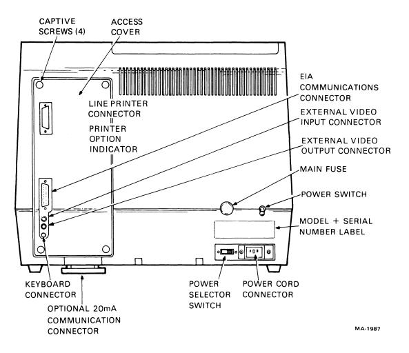
Figure 2-2 VT100 Terminal (Rear View)
