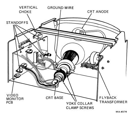
Figure 5-14 Elston Video Monitor Board Removal
