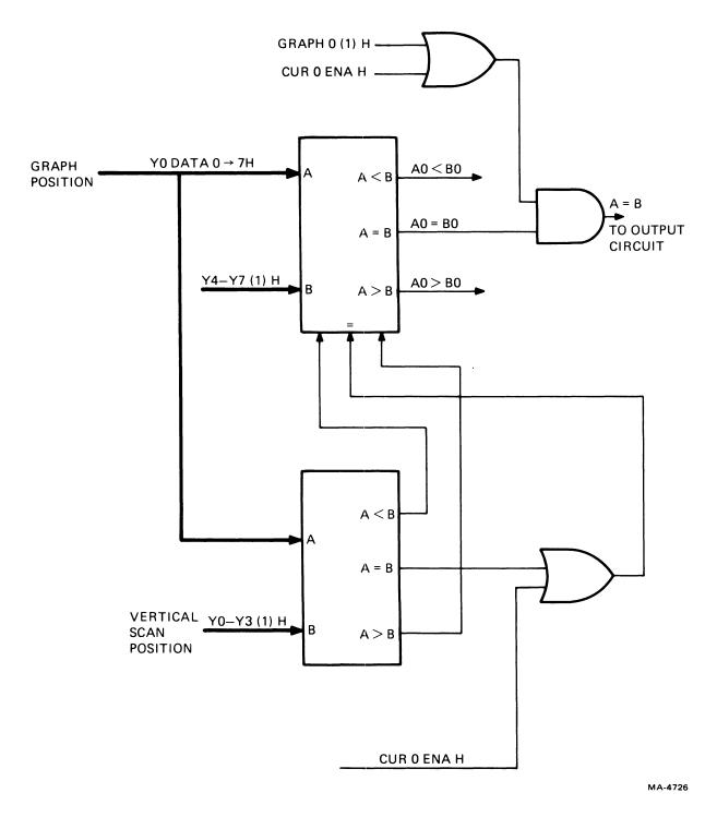
Figure 6-27 Graph Marker Y-Address Comparator
