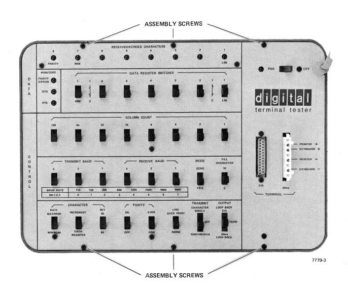
Figure 5-2 Assembly/Disassembly
