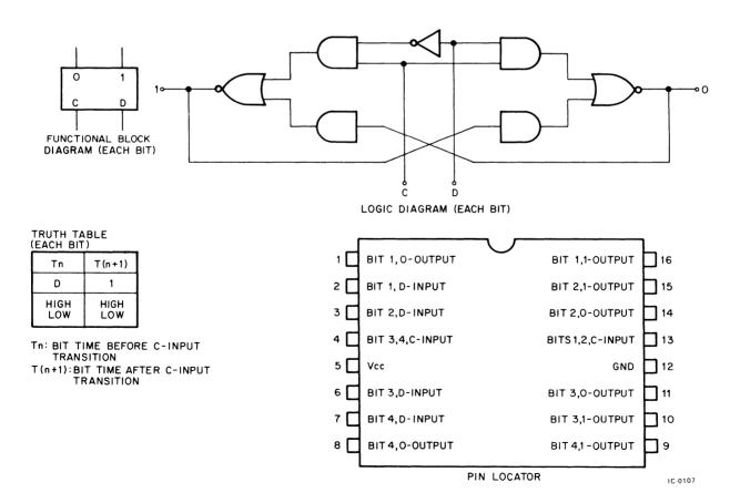
Figure B-1 7475 4-Bit Bistable Latch
