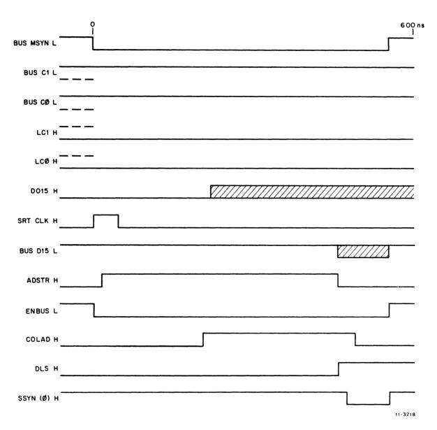
Figure 4-12 Data Read Timing (DATI)
