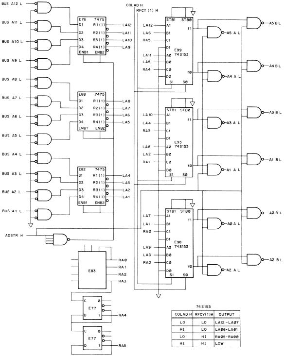
Figure 4-8 Address Path Logic
