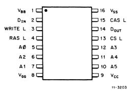
Figure 3-1 Chip Pin Connections
