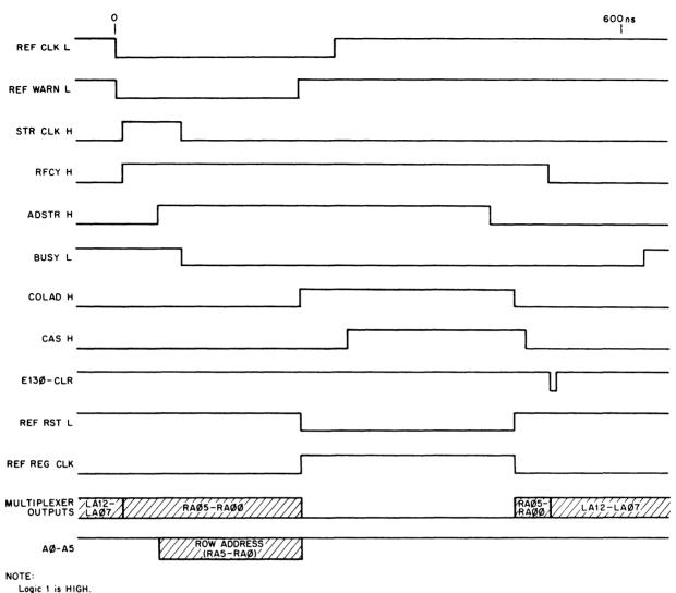
Figure 4-7 Refresh Cycle Timing Signals
