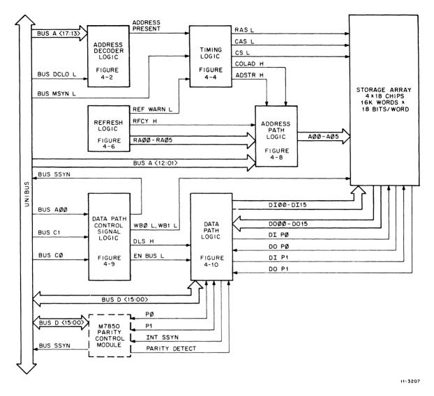
Figure 4-1 MS11 Block Diagram
