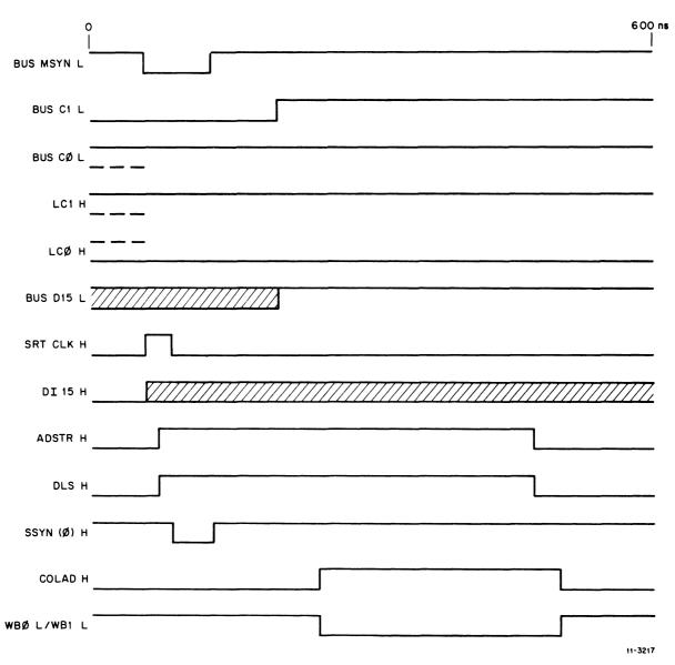
Figure 4-11 Data Write Timing (DATO
