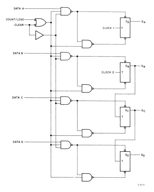
Figure B-4 74197 Logic Diagram (Sheet 1 of 2)
