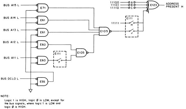
Figure 4-3 Address Decoding, I/O Address Space Logic
