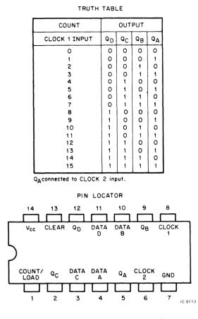
Figure B-4 74197 Truth Table and Pin Locator (Sheet 2 of 2)
