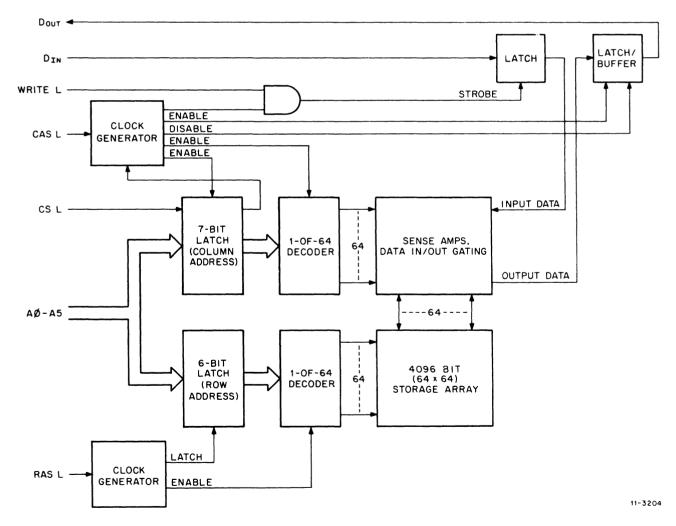
Figure 3-2 (4096  $\times$  1) Bit MOS Chip, Block Diagram
