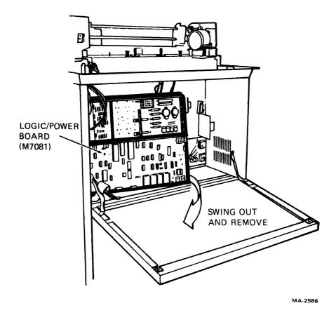
Figure 6-31 Logic/Power Board Removal and Installation
