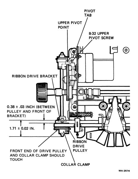
Figure 6-10 Ribbon Drive Pulley Removal and Installation
