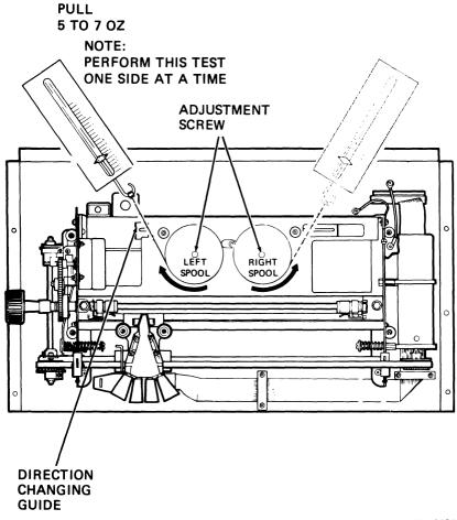
Figure 7-5 Ribbon Spool Tension Adjustment
