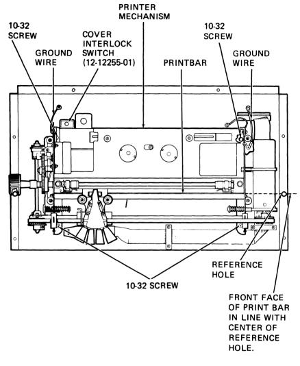
Figure 6-26 Printer Mechanism Assembly Removal and Installation
