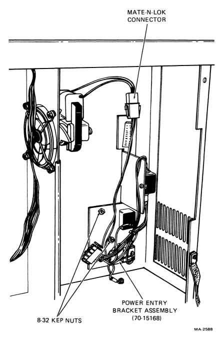
Figure 6-29 Power Entry Bracket Assembly Removal and Installation
