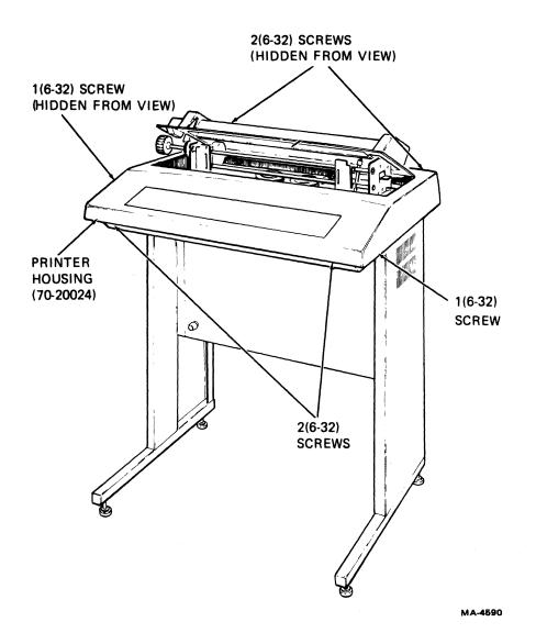
Figure 12-1 Printer Housing Removal and Installation
