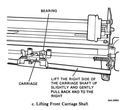
Figure 6-7 Carriage Assembly and Front Carriage Shaft Removal and Installation (Sheet 2 of 2)
