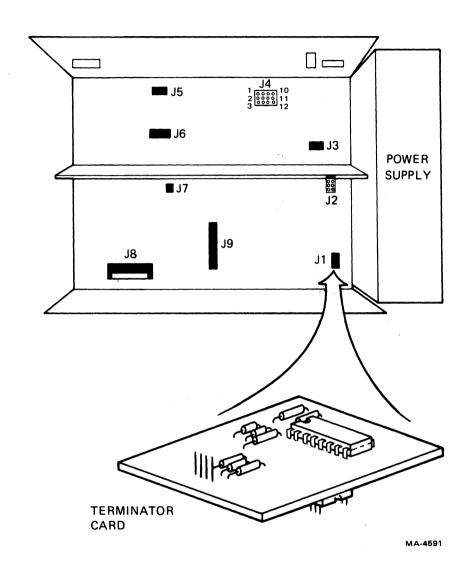
Figure 11-2 Terminator Card Removal
