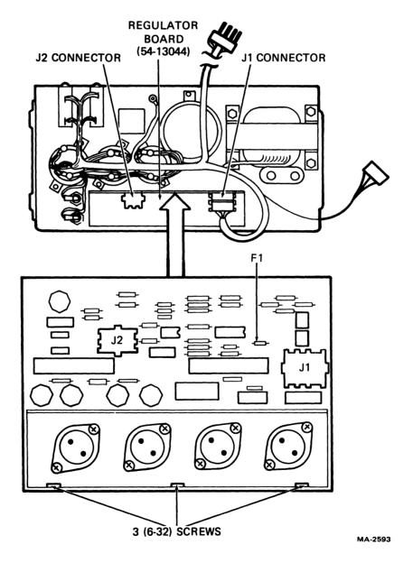
Figure 6-28 CVT Power Supply Module Removal and Installation
