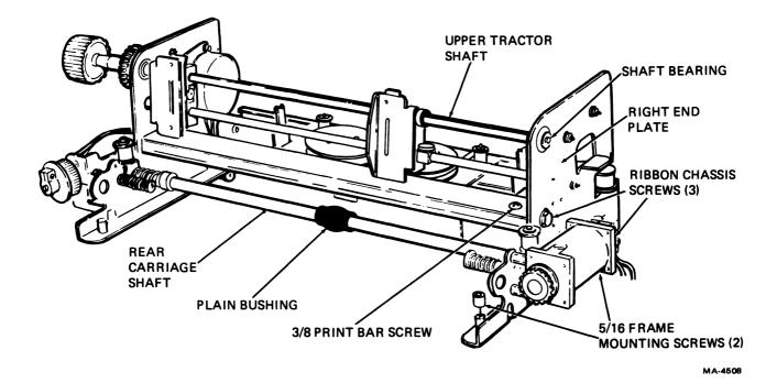
Figure 6-9 Rear Carriage Shaft and Plain Bushing Removal and Installation
