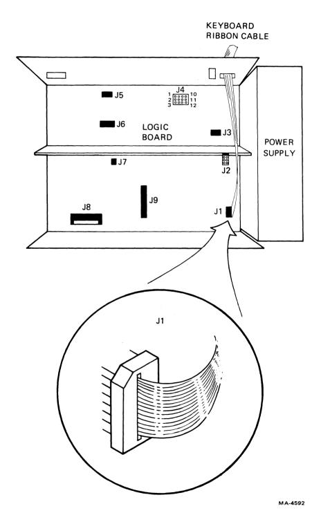
Figure 12-3 Keyboard Cable Installation
