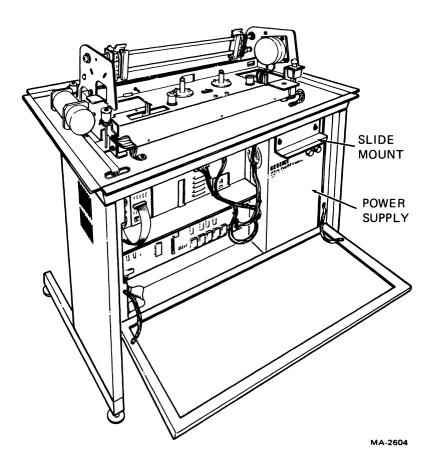
Figure 6-25 Power Supply Assembly in Position
