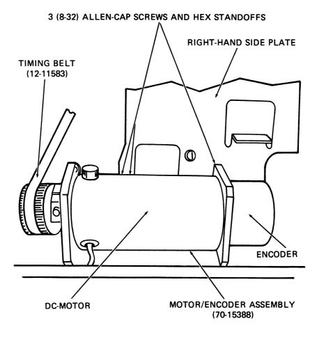
Figure 6-14 DC Motor/Encoder Assembly Removal and Installation
