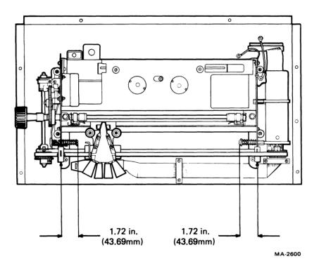
Figure 7-10 Bumper Assembly Adjustment
