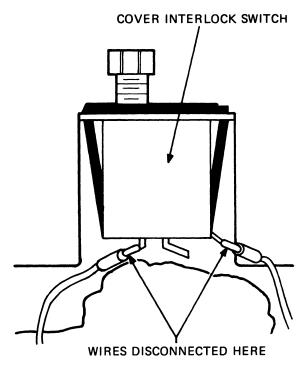
Figure 6-21 Cover Interlock Switch
