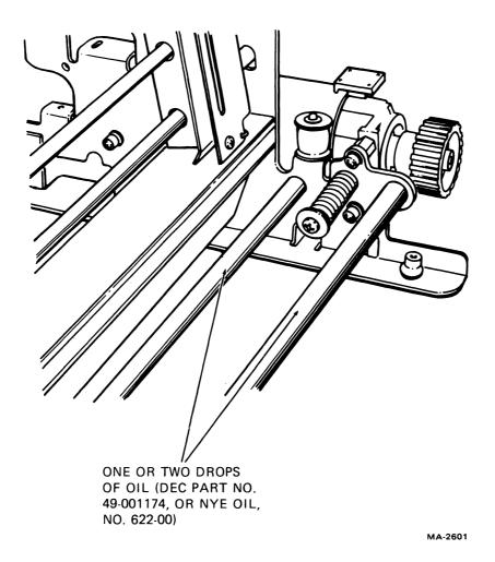
Figure 7-12 Carriage Shaft Lubrication
