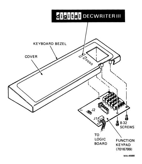
Figure 12-4 Keypad Installation
