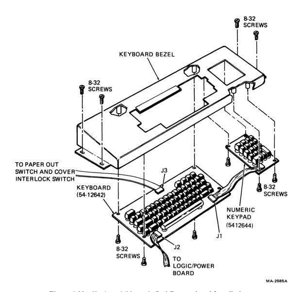
Figure 6-23 Keyboard/Numeric Pad Removal and Installation
