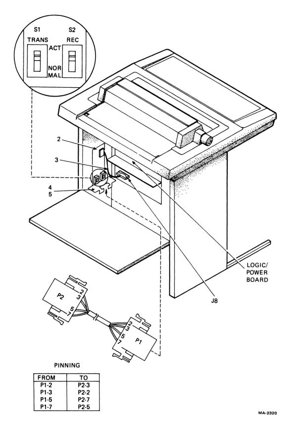
Figure 8-1 Installation of 20 mA LA12X-AL Option
