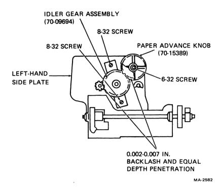
Figure 6-17 Idler Gear Assembly Removal and Installation
