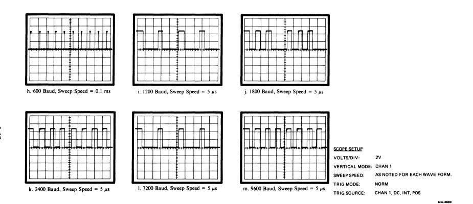
Figure 5-11 LA120 Baud Rate Clocks (Sheet 2 of 2)
