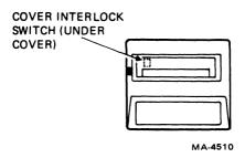
Figure 1-4 Location of Cover Interlock Switch
