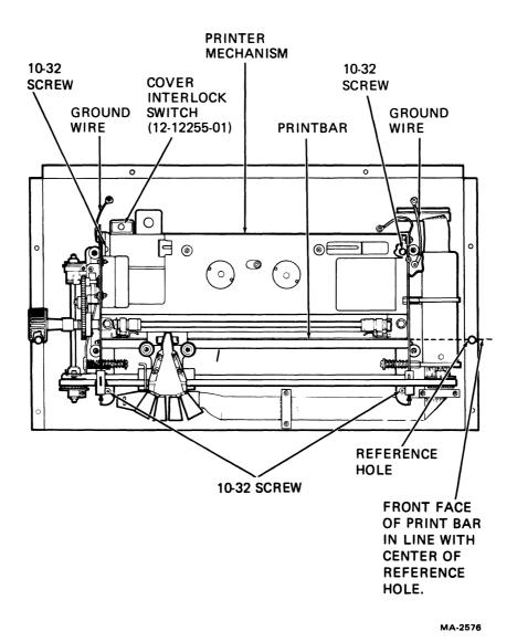
Figure 7-2 Printer Mechanism Alignment
