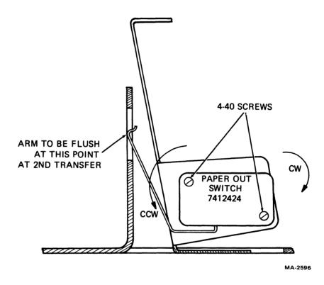
Figure 7-4 Paper Out Switch Adjustment
