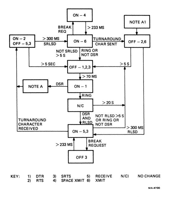
Figure 4-9 Coded Control with Reverse Channel
