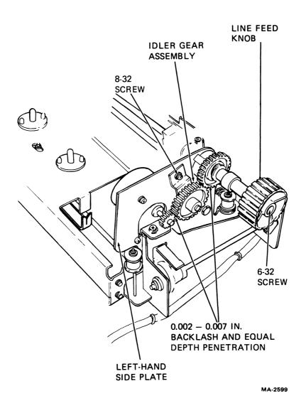
Figure 7-9 Idler Gear Assembly
