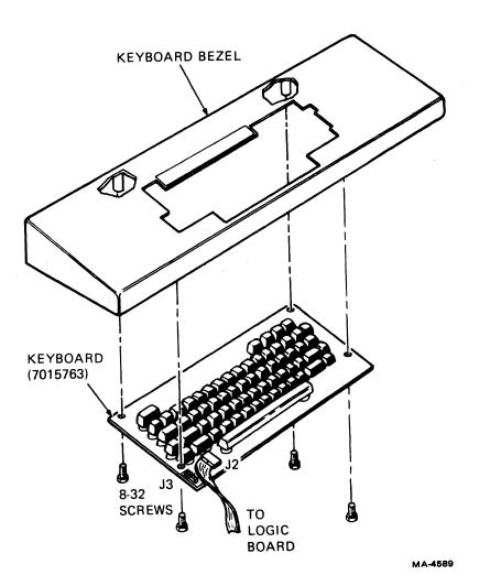
Figure 11-4 Keyboard Installation
