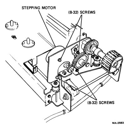
Figure 6-18 Stepping Motor Assembly Removal and Installation
