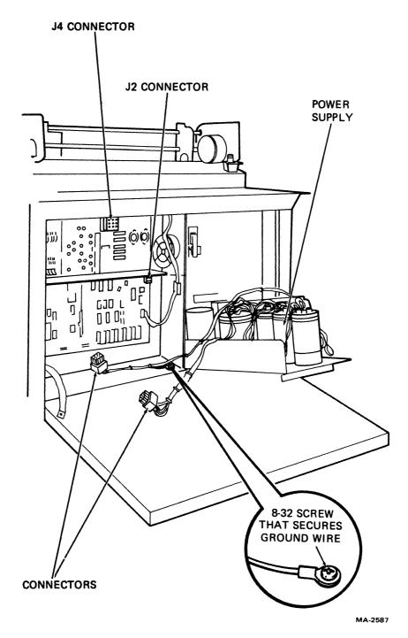
Figure 6-24 Power Supply Assembly Removal and Installation
