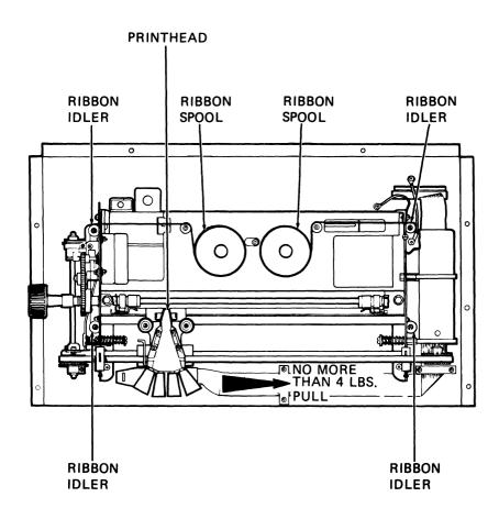
Figure 7-6 Ribbon Threading/Drag Test
