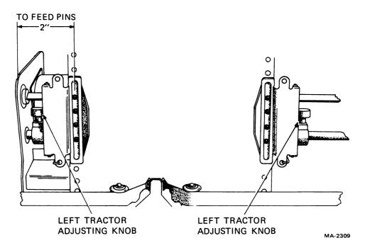
Figure 1-6 Tractor Adjust Knobs
