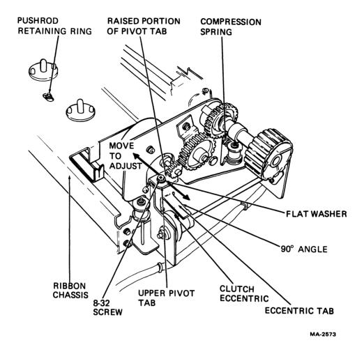
Figure 6-12 Ribbon Drive Assembly (Detailed View)
