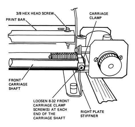
a. Carriage Shaft Clamp Screws
