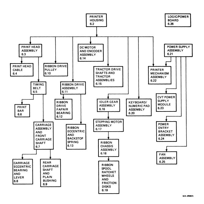
Figure 6-1 Assembly Removal Sequence
