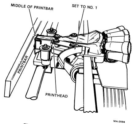
Figure 7-1 Print Head Adjustment
