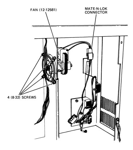
Figure 6-30 Fan Removal and Installation
