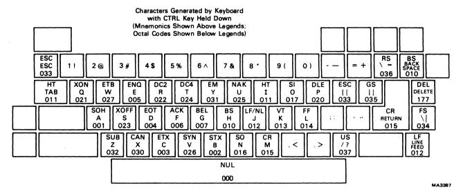
Figure 3-3 Characters Generated by Keyboard with CTRL Key Held Down
