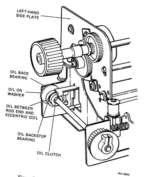
Figure 7-13 Ribbon Drive Assembly Lubrication
