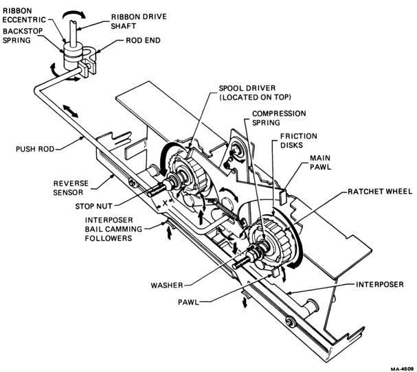
Figure 6-22 Ribbon Spool Ratchet Wheel and Friction
