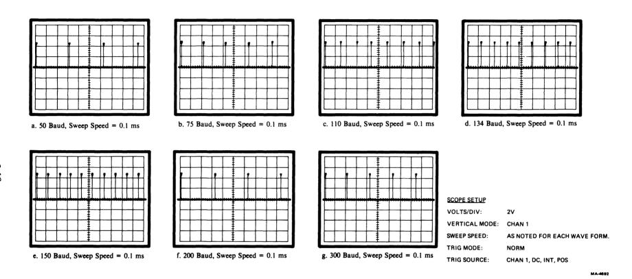
Figure 5-11 LA120 Baud Rate Clocks (Sheet 1 of 2)
