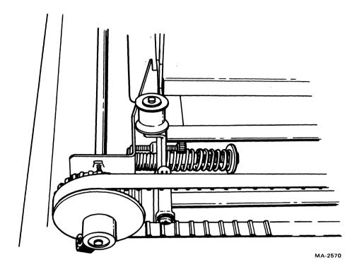
Figure 6-6 Belt Tension Spring (Detailed View)
