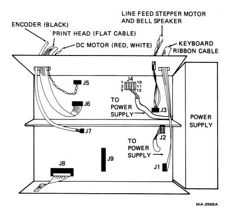
Figure 5-1 Logic/Power Board Connectors
