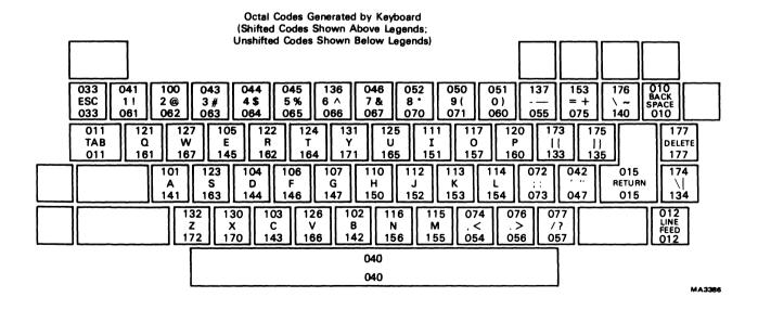
Figure 3-2 Octal Codes Generated by Keyboard
