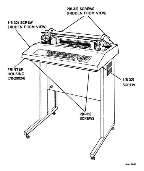
Figure 6-2 Printer Housing Removal and Installation
