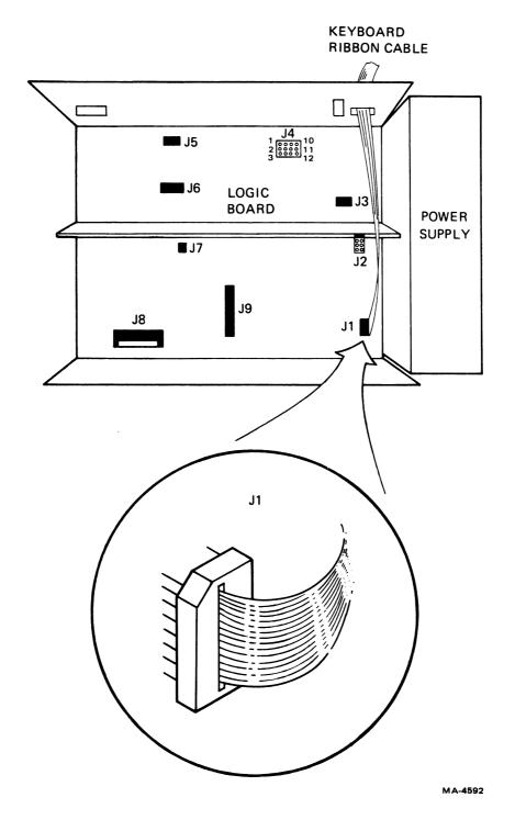
Figure 11-3 Keyboard Cable Installation
