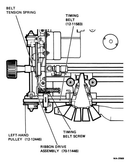
Figure 6-5 Belt Tension Spring Location
