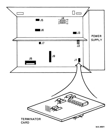
Figure 12-2 Terminator Card Removal
