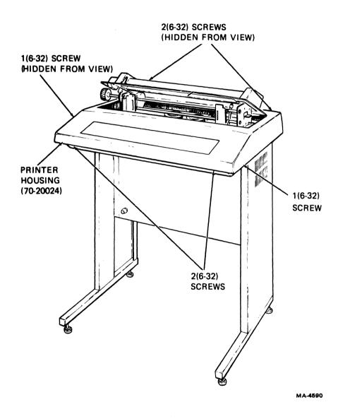
Figure 11-1 Printer Housing Removal and Installation
