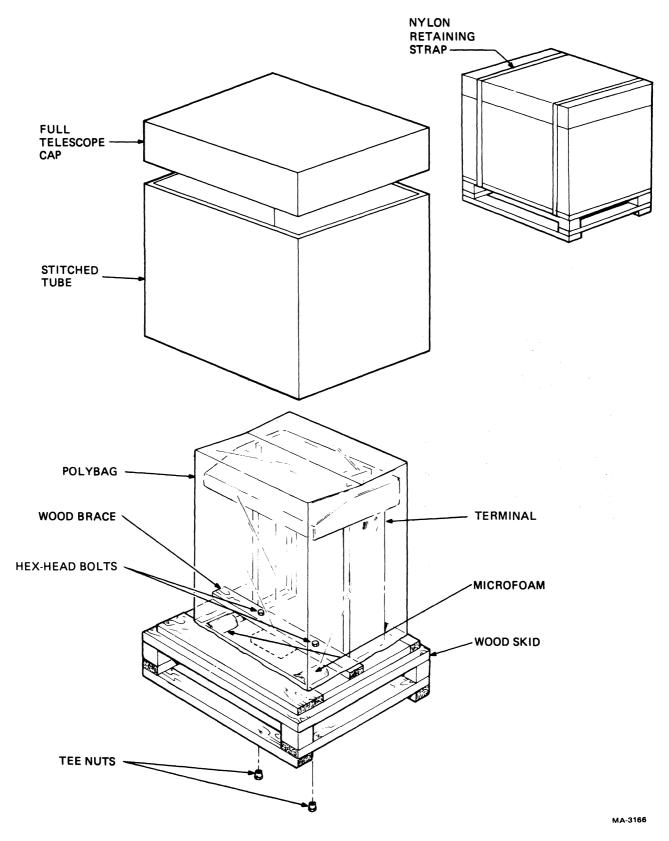
Figure 2-2 Unpacking/Packing
