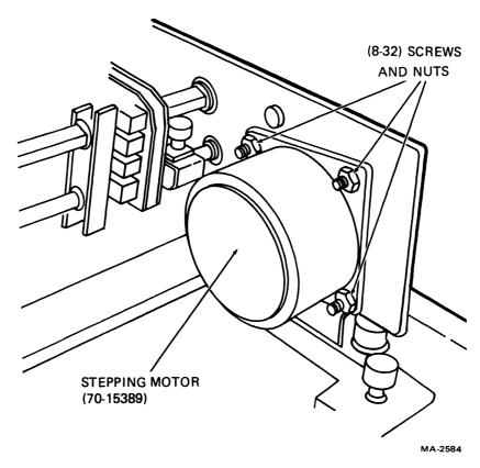
Figure 6-19 Stepping Motor Mounted on Side Plate
