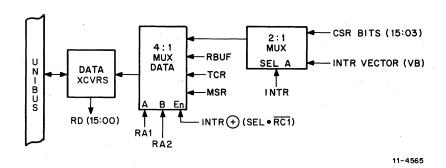
Figure 4-10 Output Data Multiplex Bit Correlation
