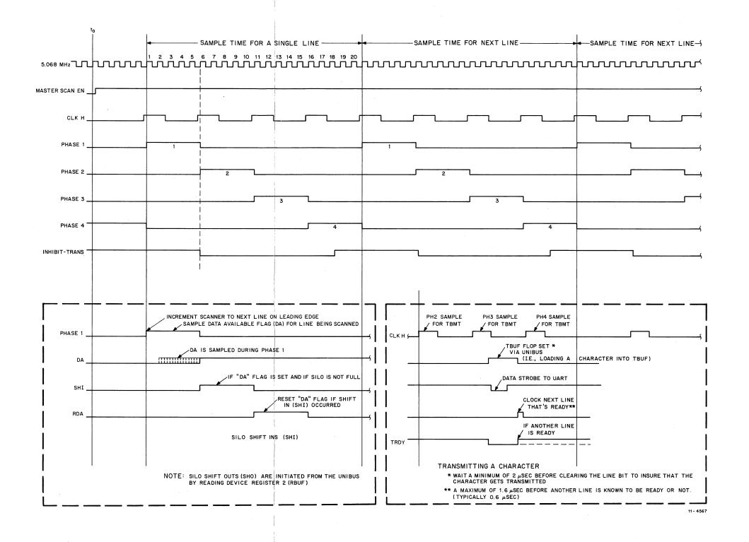
Figure 4-12 DZ11-A Scanner Timing
