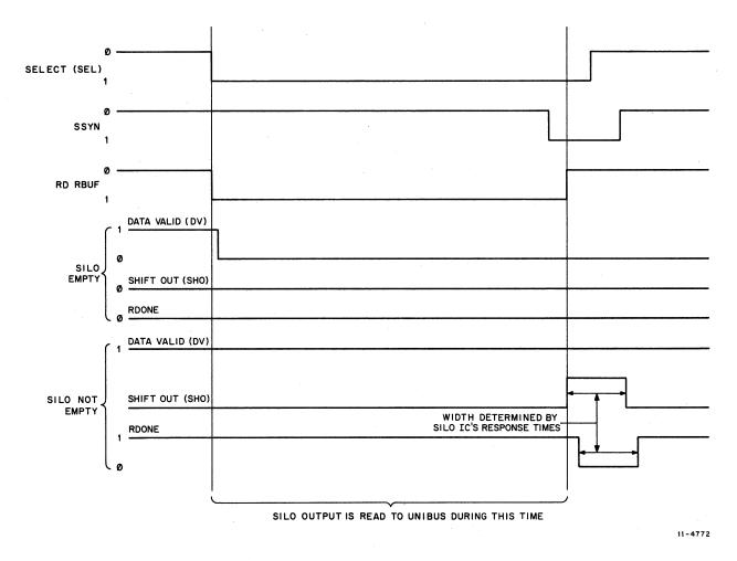
Figure 4-13 Silo Character Shift Out Timing Diagram
