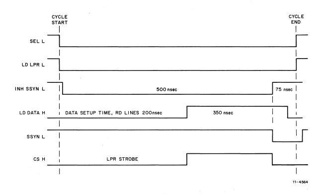
Figure 4-7 Line Parameter Loading
