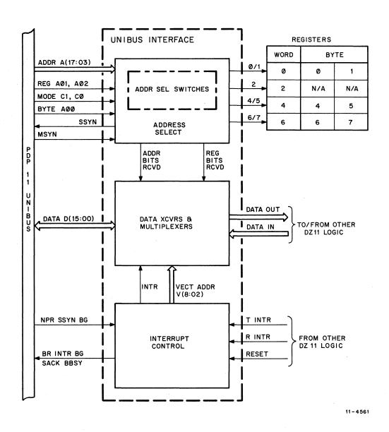
Figure 4-3 Unibus Interface Block Diagram
