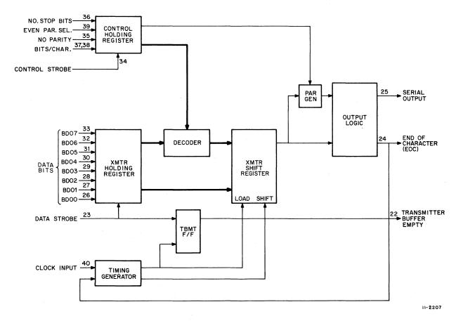
Figure C-2 UART Transmitter, Block Diagram and Simplified Timing Diagram
