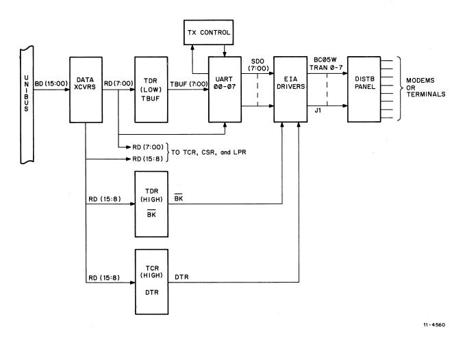
Figure 4-2 Unibus-to-Modem Data Flow (Transmit)
