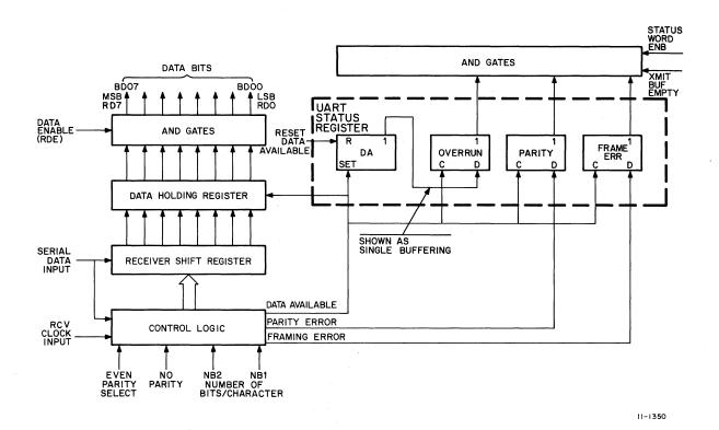
Figure 4-21 UART RCVR Block Diagram
