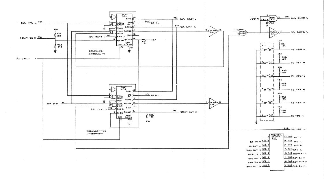
Figure 4-8 Interrupt Control Logic
