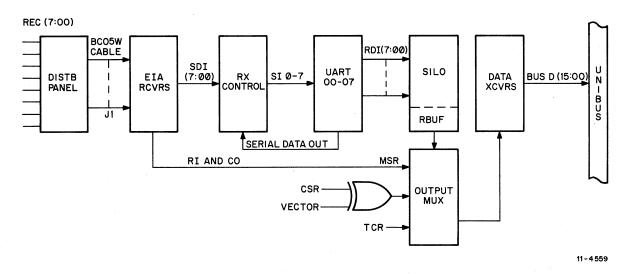
Figure 4-1 Modem-to-Unibus Data Flow (Receive)
