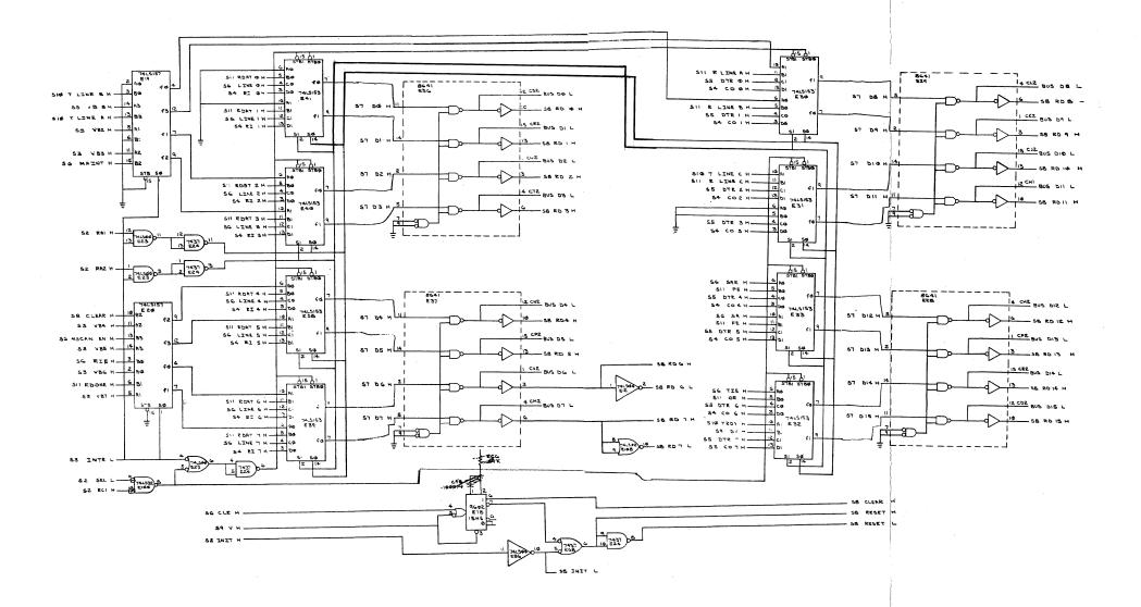
Figure 4-9 Unibus Data Flow
