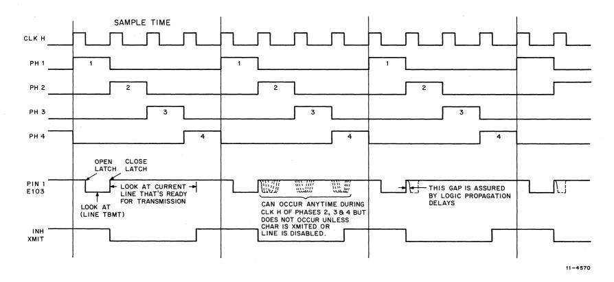
Figure 4-15 Transmit Control Timing
