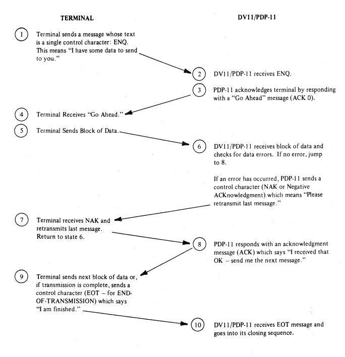
Figure B-3 Typical Data Exchange Using BSC (BISYNC)
