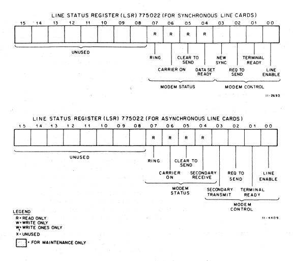
Figure 3-3 DV11 Primary Registers (Sheet 3 of 3)
