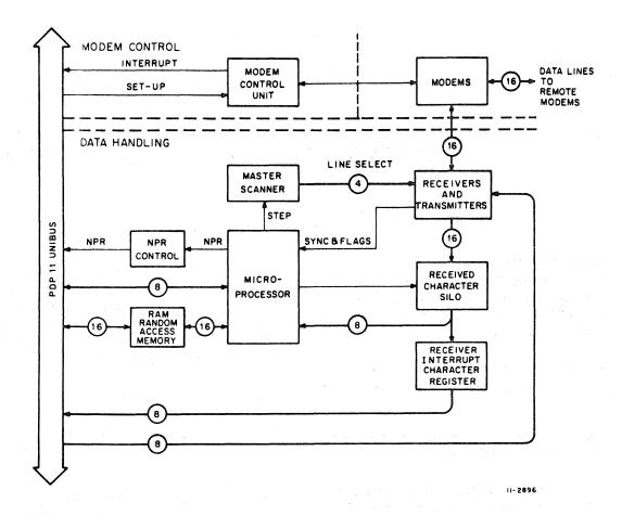
Figure 1-1 DV11 Overview Block Diagram
