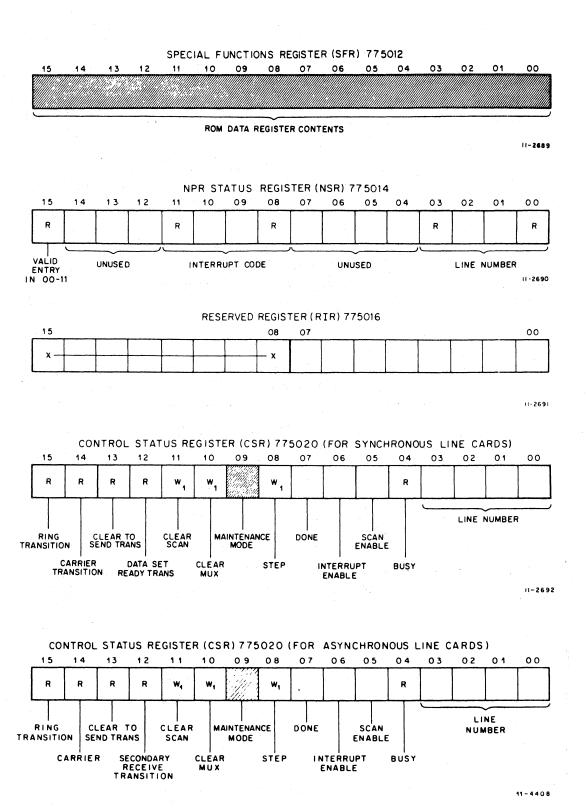
Figure 3-3 DV11 Primary Registers (Sheet 2 of 3)
