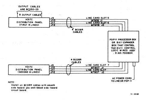
Figure 2-1 DV11 Interconnection Diagram
