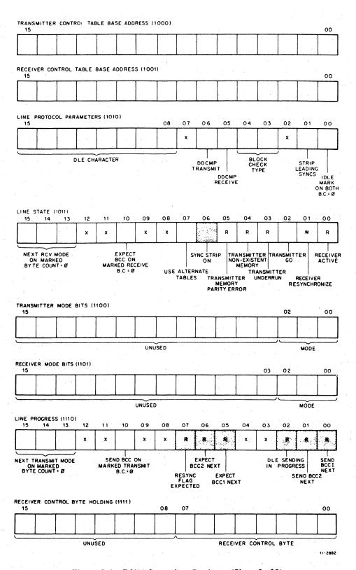
Figure 3-4 DV11 Secondary Registers (Sheet 2 of 2)
