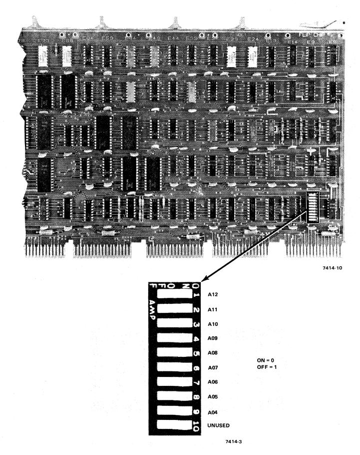
Figure 2-3 DV11 M7836 Module — Device Address Selection Switches
