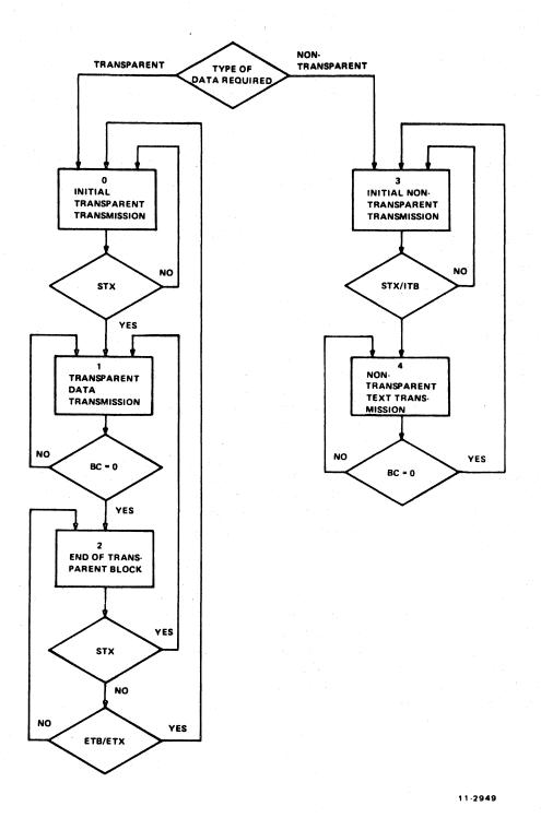
Figure 3-5 BISYNC Transmission Flow Diagram
