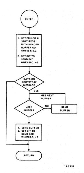
Figure 3-7 DDCMP Transmission Flow Diagram
