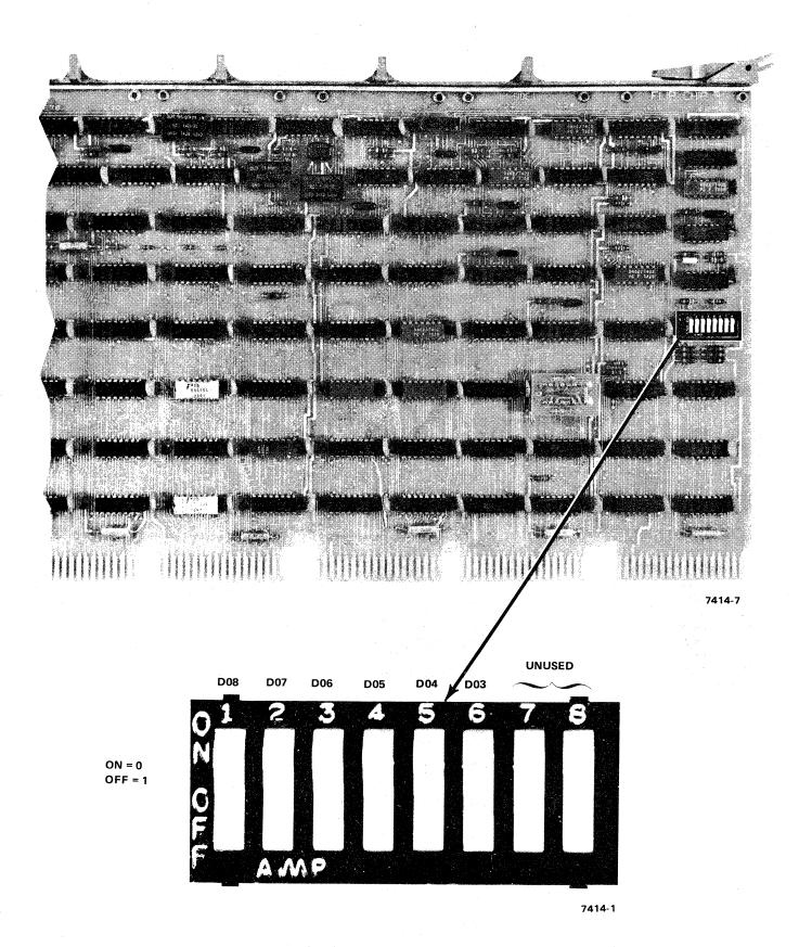
Figure 2-4 DV11 M7837 Module — Interrupt Vector Address Selection Switches for DV11 Data Handling Section
