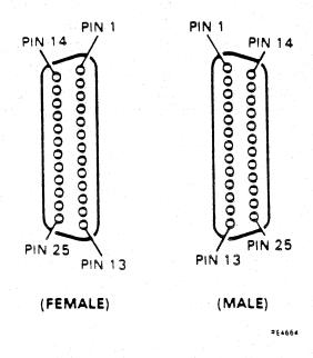
Figure C-5 25-Way D-Type Connector (Male and Female)
