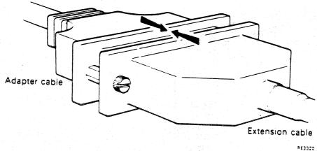
Step 3: Connect the Extension Cable to the Modem
