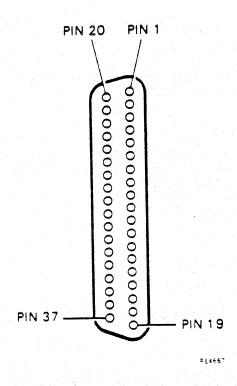
Figure C-1 37-Way D-Type Connector (Male)
