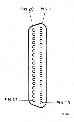
Figure C-2 37-Way D-Type Connector (Male)
