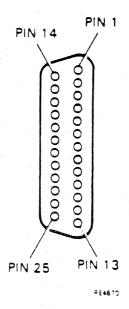
Figure C-4 25-Way D-Type Connector (Male)
