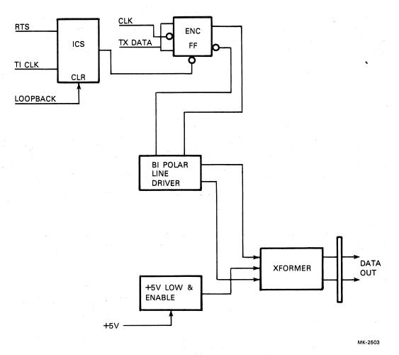
Figure 6-8 Integral Modem Transmit
