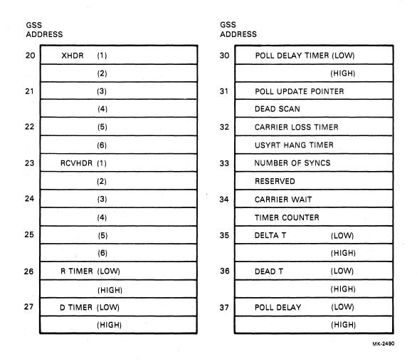
Figure 5-10 Global Status Slot (Sheet 2 of 2)
