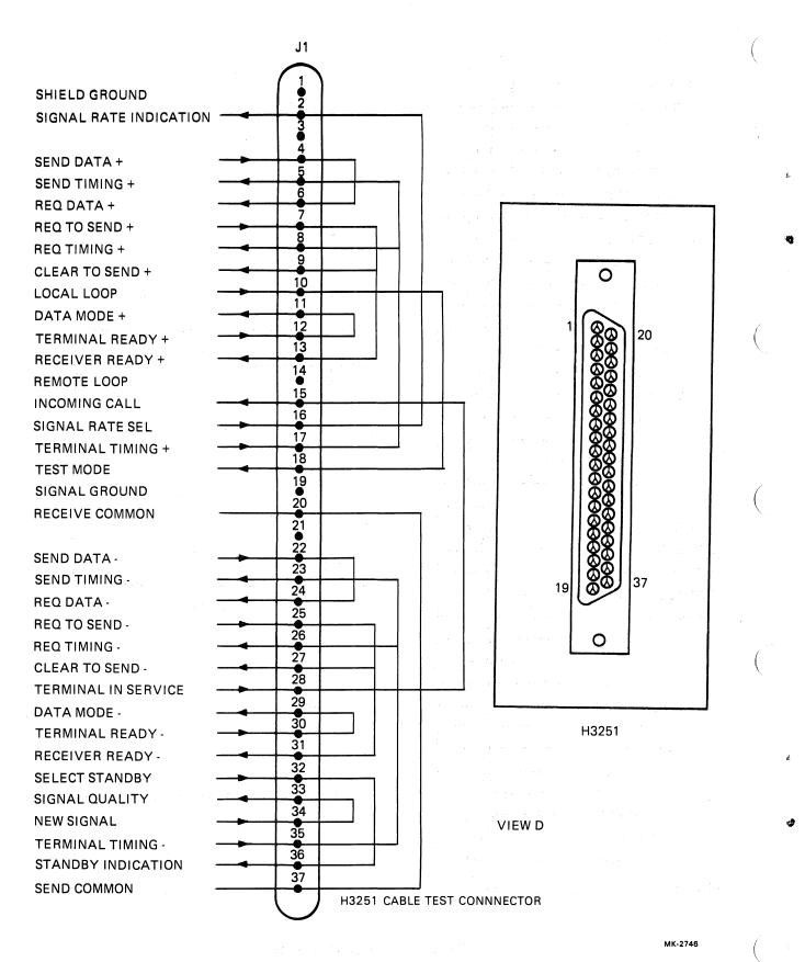
Figure 2-8 DMV11 Test Connectors (Sheet 3 of 4)
