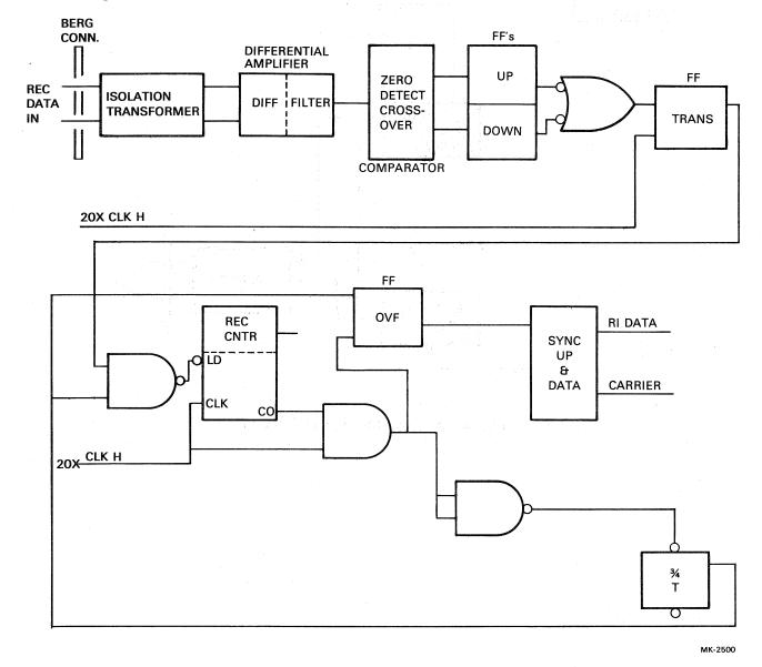
Figure 6-7 Integral Modem Receive
