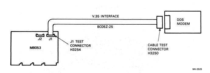
Figure 2-10 DMV11 Remote System Cabling Diagram
