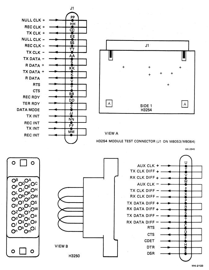
Figure 2-8 DMV11 Test Connectors (Sheet 1 of 4)
