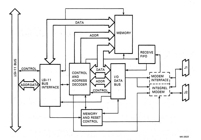
Figure 6-1 DMV11 Block Diagram
