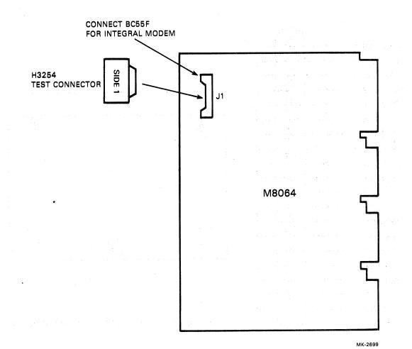
Figure 2-7 Test Connector Insertion for the M8064
