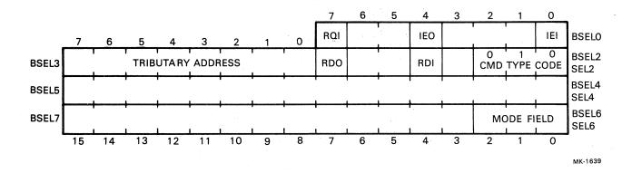
Figure 3-5 Mode Definition Command Format
