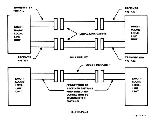
Figure 2-2 Full-Duplex/Half-Duplex Connections
