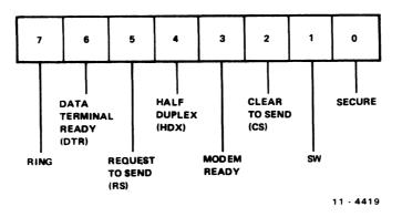
Figure 3-4 Modem Control Register Format
