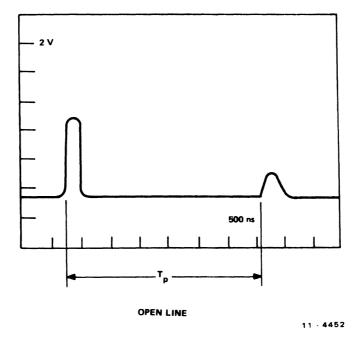
Figure 2-1 Signal Reflections from a Line Fault
