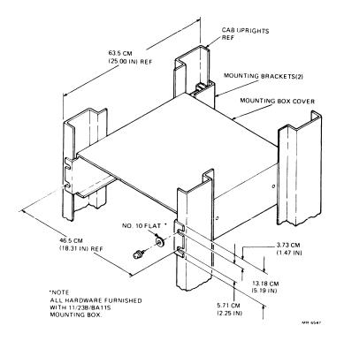
Figure 2-5 BA11-S Cover Mounting Dimensions
