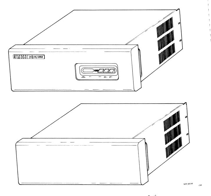
Figure 1-2 BA11-S with Control Panel and Blank Front Panel
