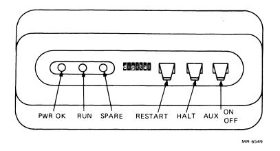
Figure 2-8 Front Panel Switches and Indicators
