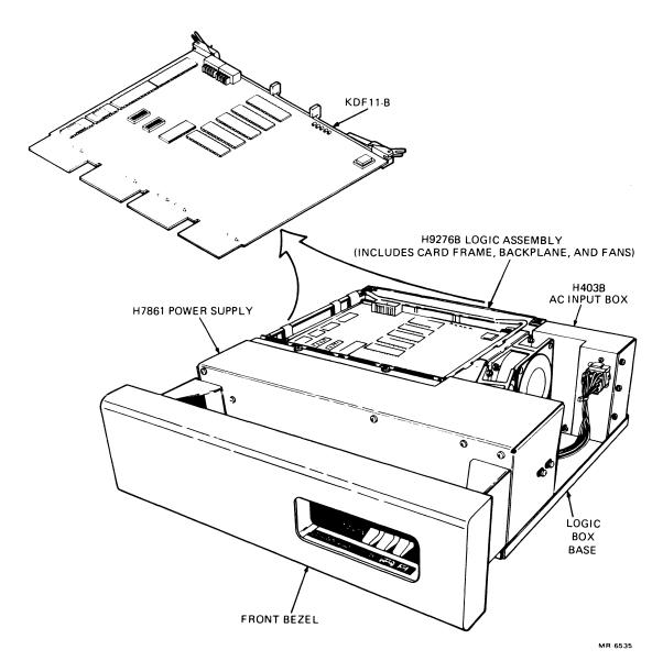
Figure 1-3 BA11-S Logic Box, Cover Removed
