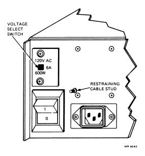
Figure 2-1 BA11-S Voltage Selection Switch
