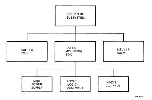
Figure 1-1 PDP-11/23B Subsystem
