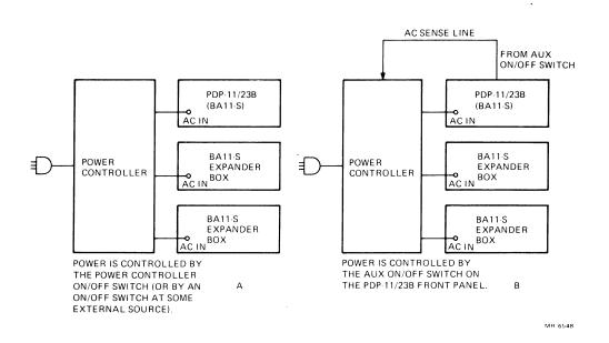
Figure 2-7 Power Connections, PDP-11/23B
