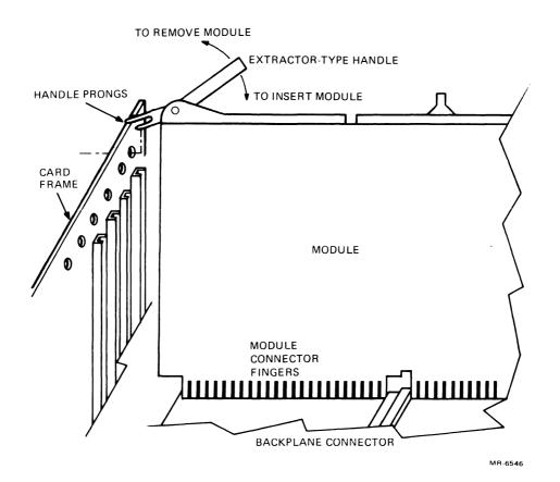
Figure 2-4 Insertion and Removal of Modules with Extractor-Type Handles
