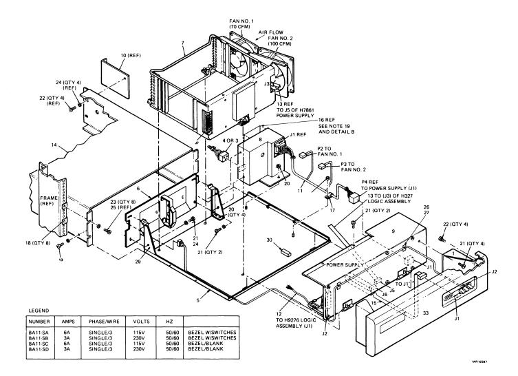
Figure 2-6 BA11-S Unit Assembly Drawing
