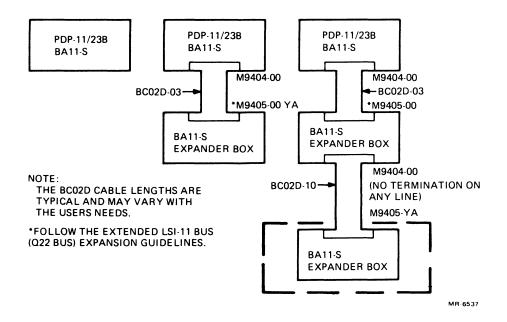
Figure 1-5 BA11-S Typical System Application (PDP-11/23B)
