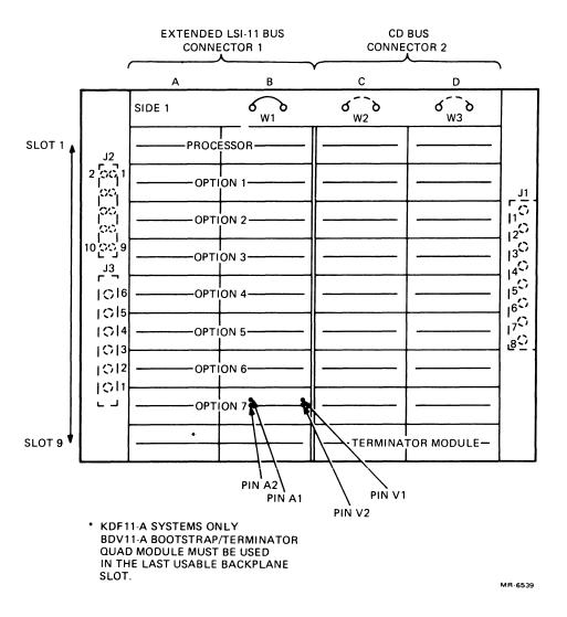
Figure 1-7 H9276 Backplane Connectors (Module Side)
