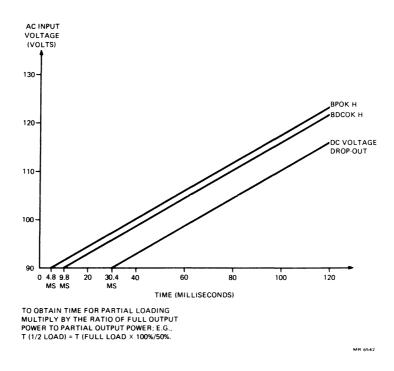
Figure 1-10 H7861 Power Supply Minimum Ride-Through After Power Interruption
