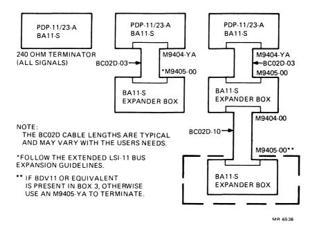
Figure 1-6 BA11-S System Application (PDP-11/23A)
