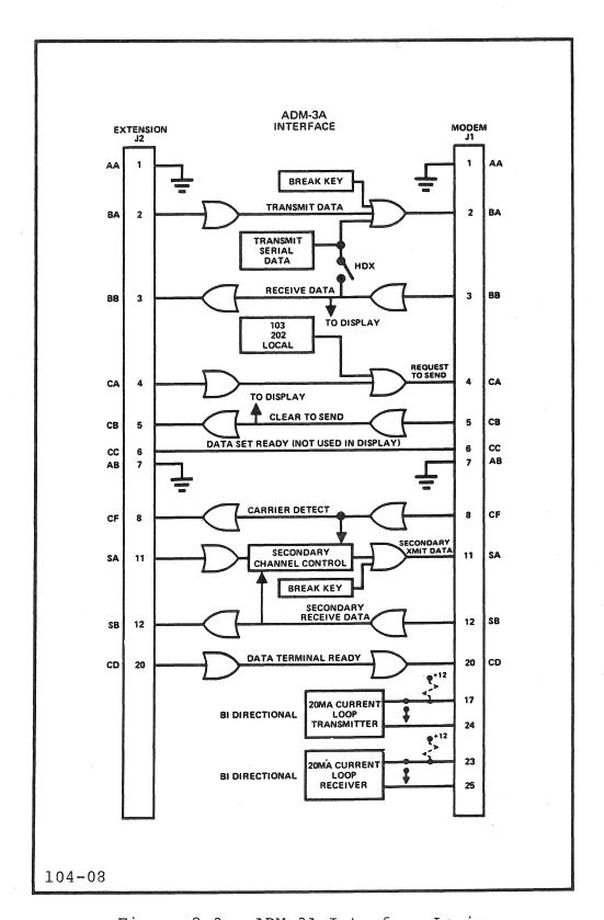
Figure 2-3. ADM-3A Interface Logic
