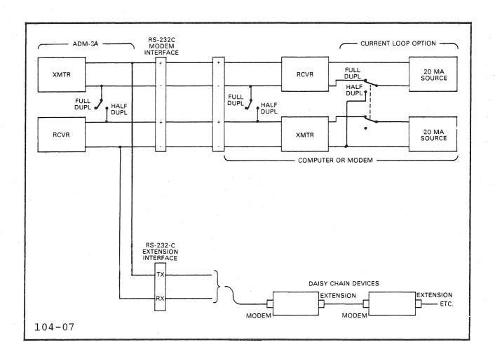
Figure 2-2. Typical ADM-3A Interfaces
