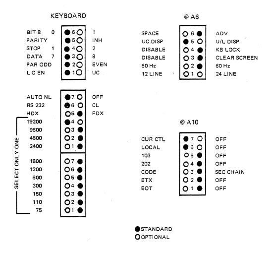
Note: To operate in the off-line or Local Mode, the HDX/FDX Switch should be in the HDX position.
