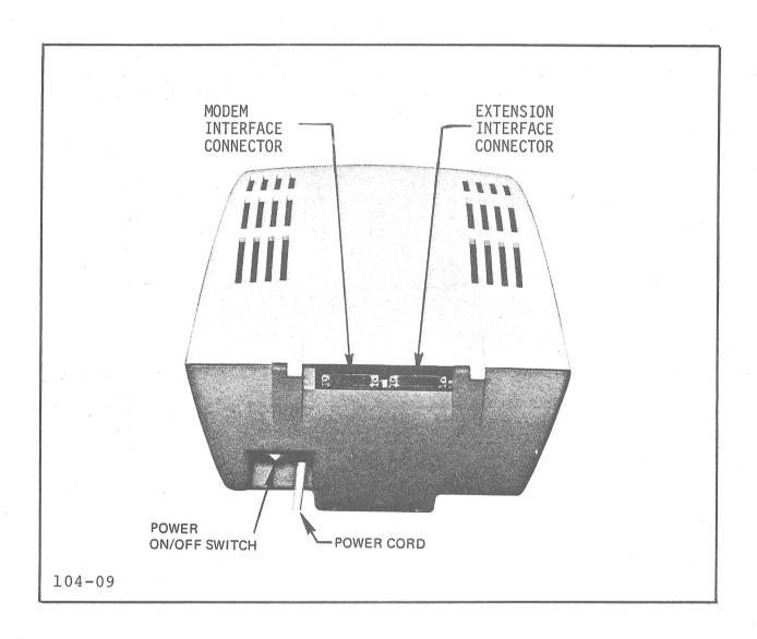
Figure 2-4. ADM-3A Rear Panel Controls
