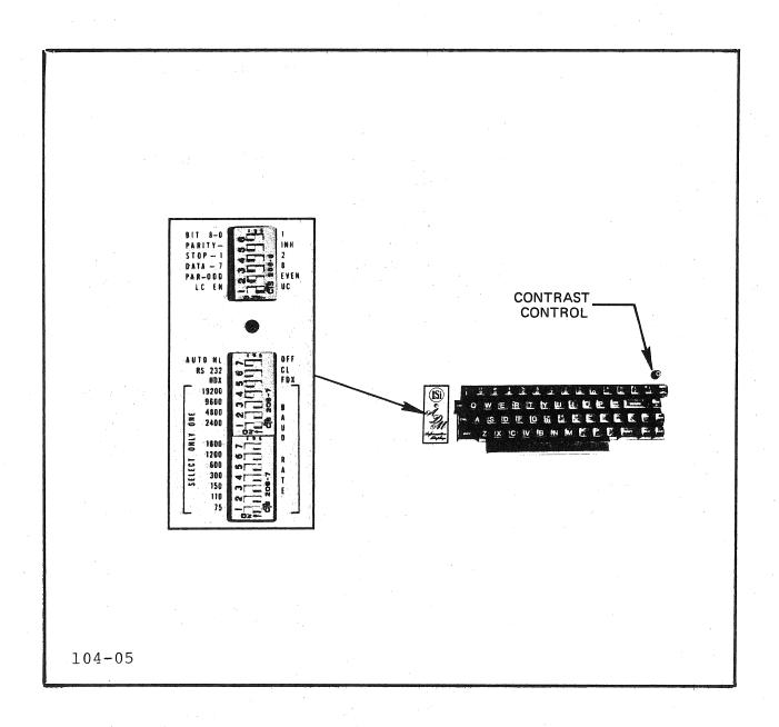
Figure 1-5. Front Panel Switch Locations
