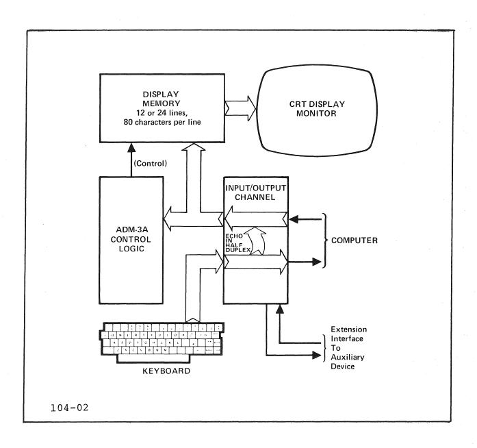
Figure 1-2. ADM-3A Data Flow Block Diagram
