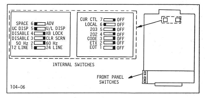
Figure 2-1. ADM-3A Configuration Control Switch Locations
