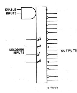
Figure 1-14 Binary to Decimal Decoder
