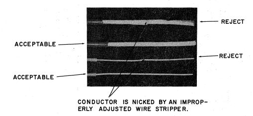
Figure 5-8 Stripping Damage
