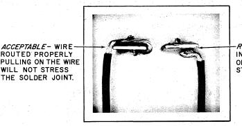
REJECT- WIRE ROUTED INCORRECTLY, PULLING ON THE WIRE WILL STRESS THE JOINT.
