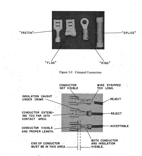
Figure 5-10 Acceptable and Unacceptable Crimped Connections
