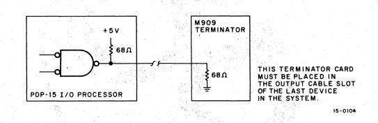
Figure 6-7 The PDP-15 I/O Bus Drive/Termination Scheme
