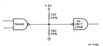
Figure 5-1 Terminating Long Wires
