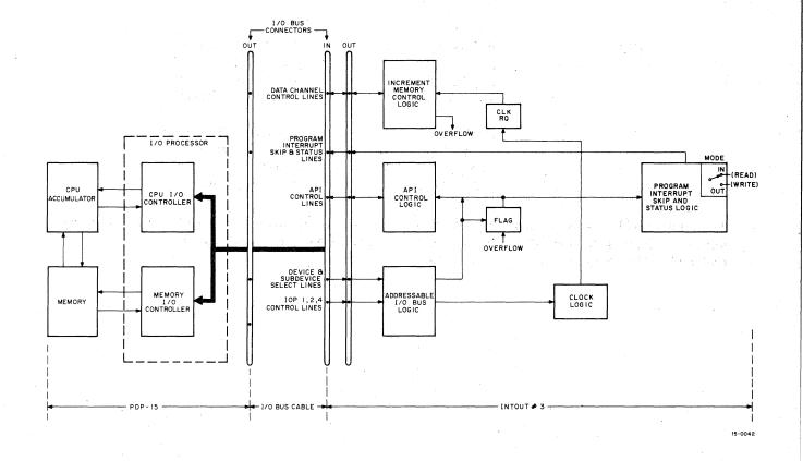
Figure 4-8 Block Diagram for Increment Memory
