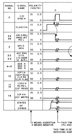
Figure 4-4 Timing Diagram of the CPU Device with API
