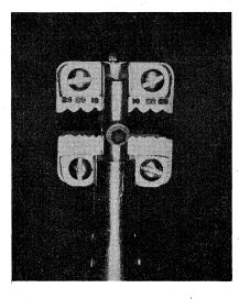
Figure 5-6 Non Adjustable Wire Stripper
