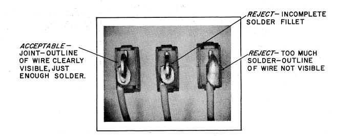
REJECT-INSUFFIENT SOLDER-CAUSED BY USING TOO SMALL A SOLDERING IRON ON A LARGE (#10) WIRE.
