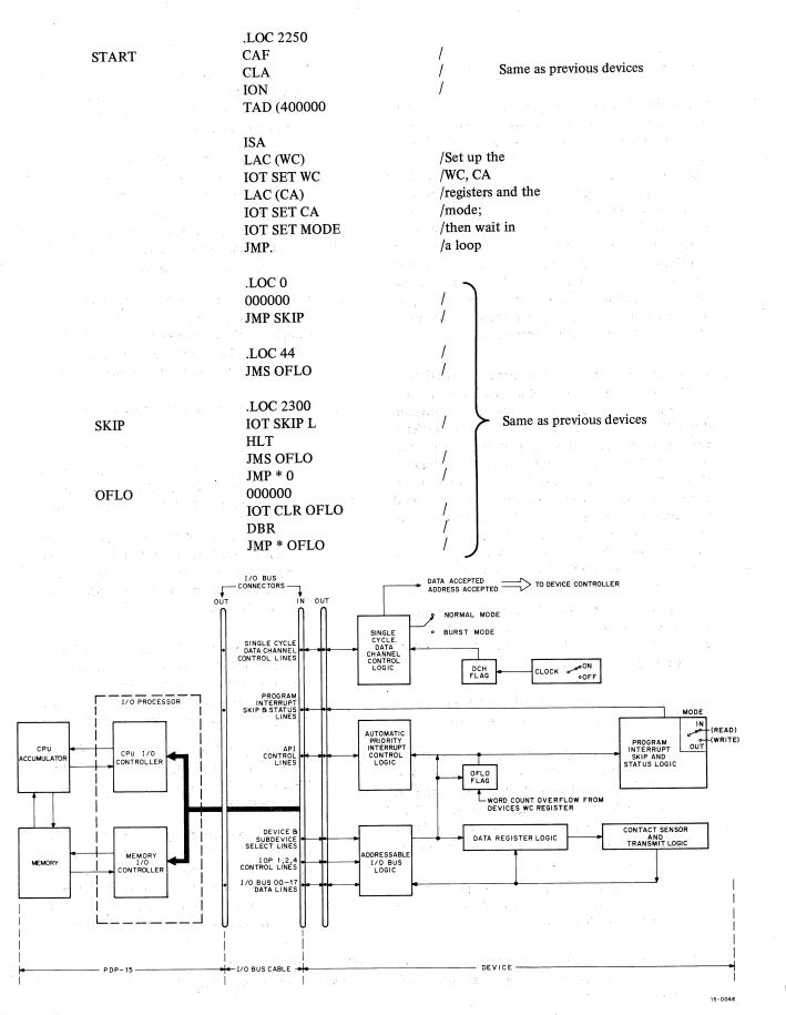
Figure 4-11 Block Diagram of Single-Cycle Data Channel Device
