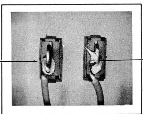
ACCEPTABLE-SOLDER-SMOOTH AND SHINY. *REJECT*-SOLDER PEAK, IRON REMOVED TOO SOON
