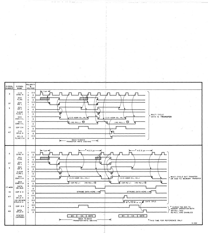
Figure 4-6 Multi-Cycle Data Channel Device Logic
