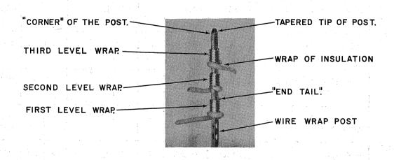
THE CONNECTOR BLOCK AND OTHER POSTS HAVE BEEN ELIMINATED FROM THE PICTURE FOR CLARITY.
