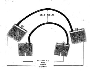
Figure 6-2 BC09A Cable Assembly
