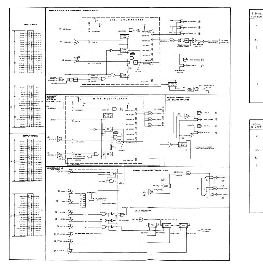
Figure 4-12 Logic Diagram of Single-Cycle Data Channel
