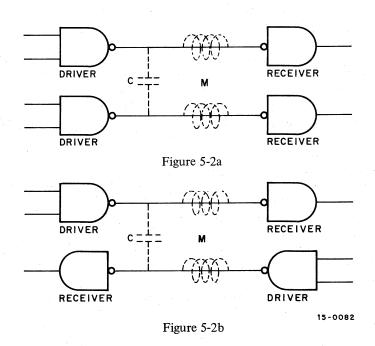
Figure 5-2 Capacitance and Inductive Crosstalk Components
