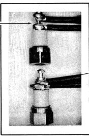
REJECT- BOTTOM WIRE OVERWRAPPED, OTHER WIRE NOT IN CONTACT WITH POST.
