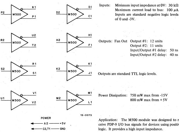
Figure 2-8 M500 Receiver Module
