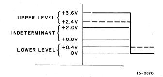
Figure 2-2 Voltage Spectrum of TTL Logic
