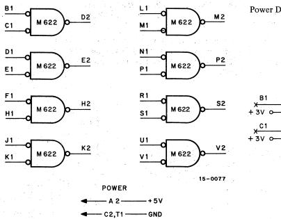
Outputs: Outputs are standard PDP-15 positive I/O bus signals.
