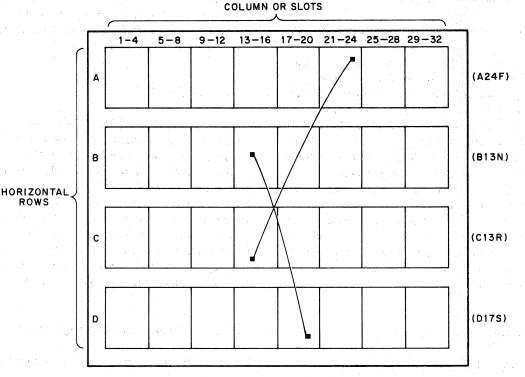
Figure 5-13 Wire Wrap Post Location Standard
