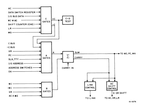
Figure 3-1 CPU Bus Structure
