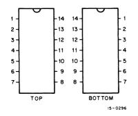
Figure 7-2 Integrated Circuit Pin Location
