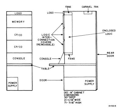
Figure 1-3 PDP-15/10 System Configuration Diagram
