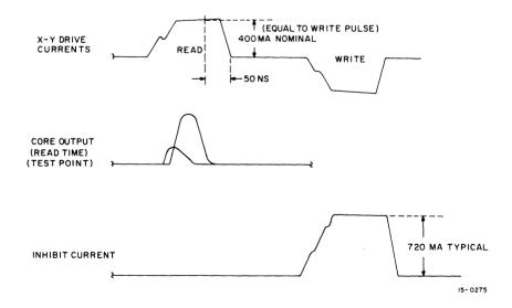
Figure 2-3 Typical Inhibit Current Waveforms
