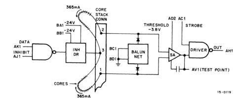
Figure 2-2 Sense Amplifier/Inhibit Driver, Simplified Diagram
