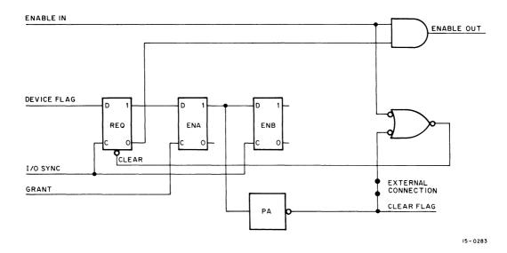
Figure 4-7 Simplified M104 Module Diagram
