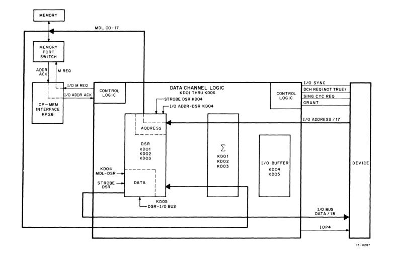
Figure 4-12 Single Cycle Data Out Transfer, Block Diagram
