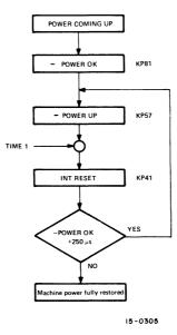
Figure 6-6 Power Restore Sequence With Power Fail Option Disabled, Flow Diagram
