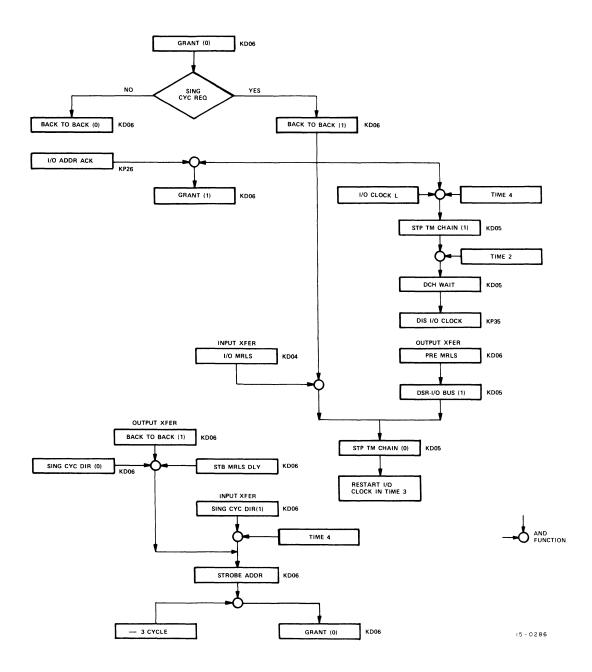
Figure 4-11 Single Cycle Back-To-Back Transfer, Detailed Flow Chart
