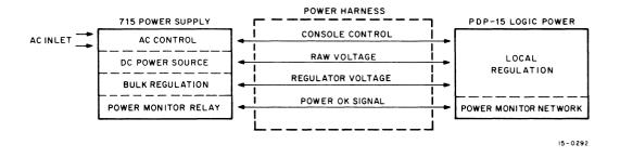
Figure 5-1 Power Distribution Block Diagram
