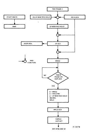
Figure 2-7 Central Processor Write Cycle
