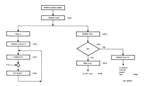
Figure 6-7 Power Fail Sequence With Power Fail Option Enabled, Flow Diagram
