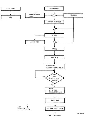
Figure 2-6 Central Processor Read Cycle
