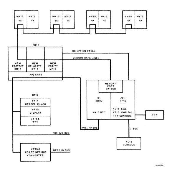
Figure 1-2 PDP-15 System Block Diagram
