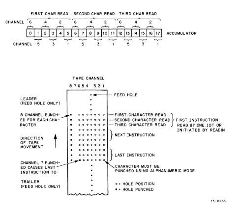
Figure 6–14 HRI Tape Format and Accumulator Bits (Binary Mode)
