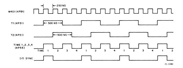
Figure 4-1 Basic I/O Timing
