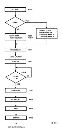
Figure 6–16 High–Speed Punch Operation, Flow Diagram
