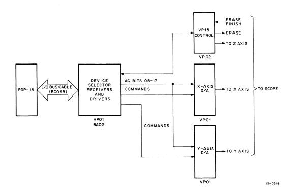
Figure 6-19 VP15 Controller, Simplified Block Diagram
