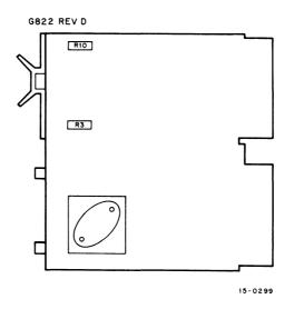
Figure 7-4 G822 Module Adjustment Locations
