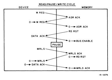
Figure 2-4 Basic Device-Memory Control Signal Flow
