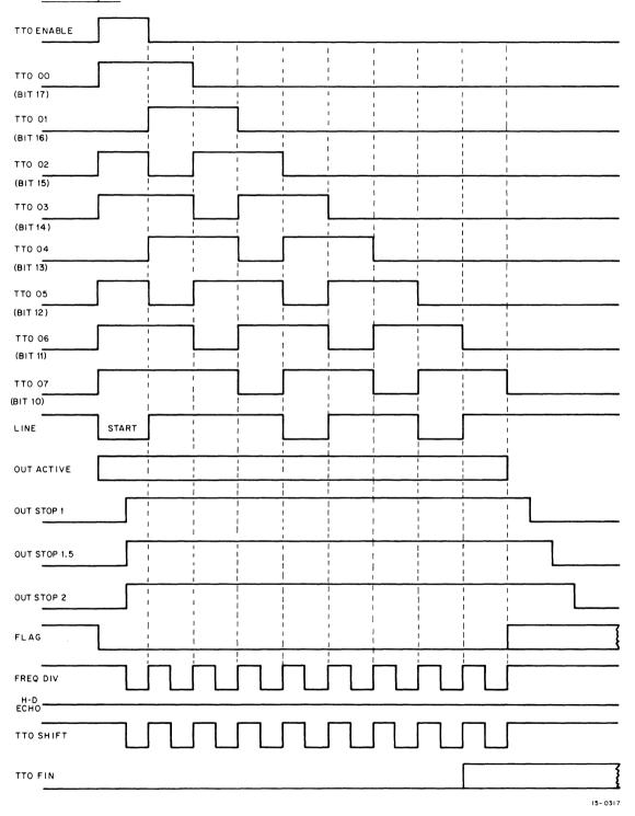
Figure 6-18 Teletype Transmitter (Printer) Timing
