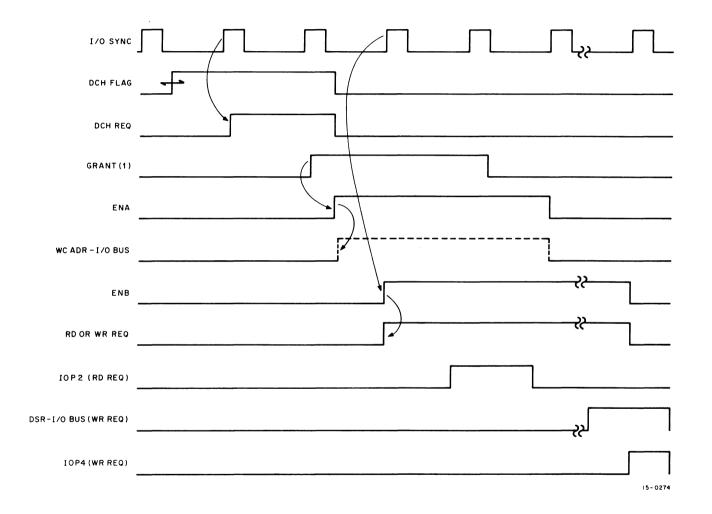
Figure 4–15 Multicycle Timing Diagram
