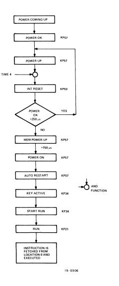
Figure 6–8 Power Restore Sequence With Power Fail Option Enabled, Flow Diagram
