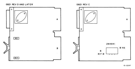
Figure 7-3 G821 Module Adjustment
