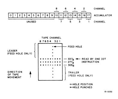
Figure 6-13 Tape Format and Accumulator Bits (Alphanumeric Mode)
