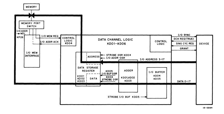
Figure 4-9 Single Cycle Data In Transfer, Block Diagram
