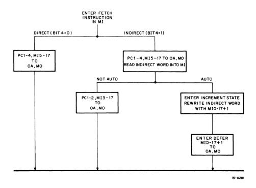
Figure 3-3 Bank (PDP-9) Mode Address Formation
