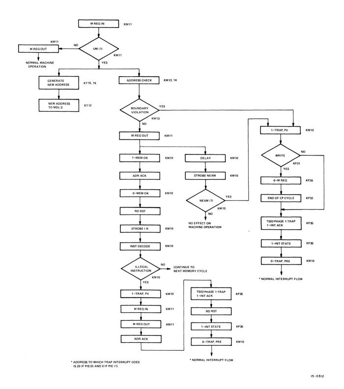
Figure 6–12 KT15 Memory Protect/Relocate Flow Diagram
