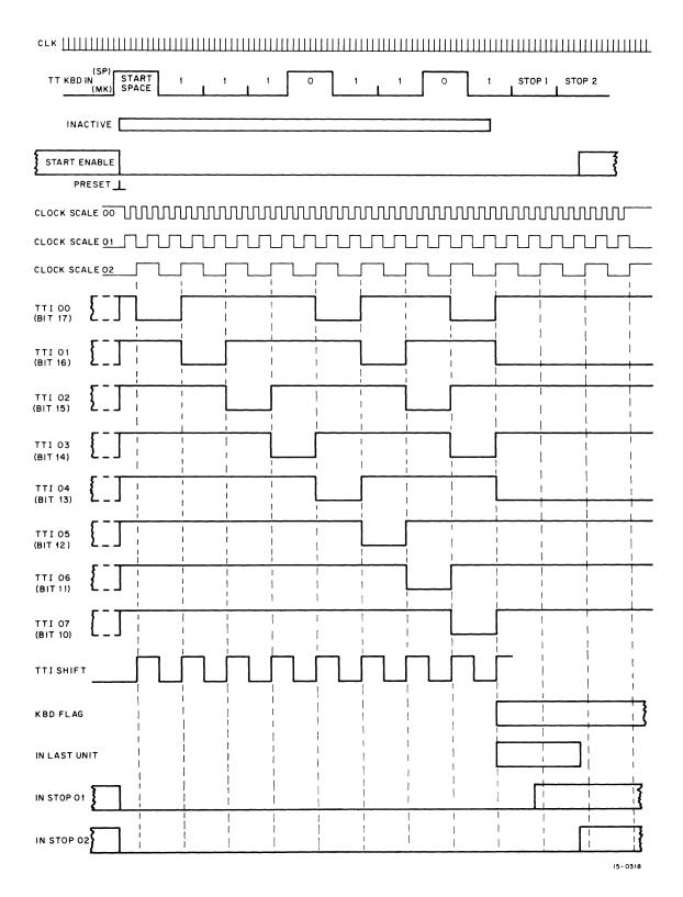
Figure 6-17 Teletype Receiver (Keyboard) Timing
