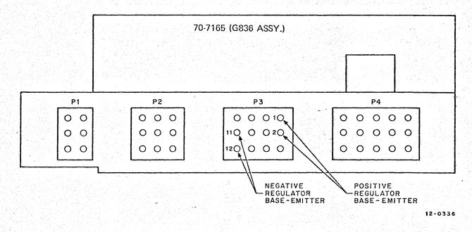
Figure 4 Base-Emitter Voltage Drop, Test Point Location
