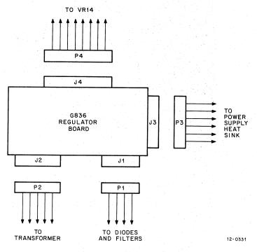
Figure 4-3 7007165 Power Regulator Assembly
