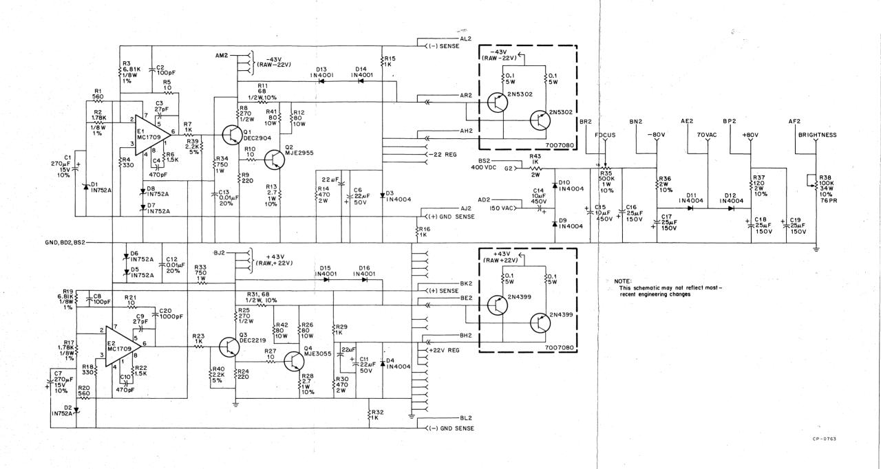
Figure 3-2 G836 Circuit Board, Part of the 7007165 Power Regulator Assembly
