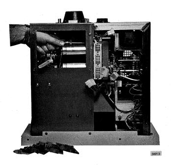
a. Remove power cord and all connectors to the 7007165. Unscrew mounting screws from the opposite side of the vertical chassis wall.
