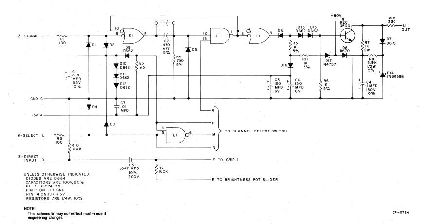
Figure 3-3 Intensity Amplifier W682, Circuit Schematic
