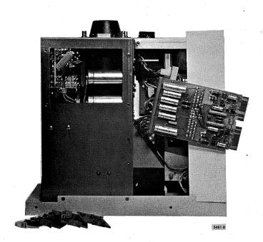
b. Reconnect connectors and place a cardboard under the 7007165 to prevent shorting out the circuit against the chassis when troubleshooting the board outside the unit.
