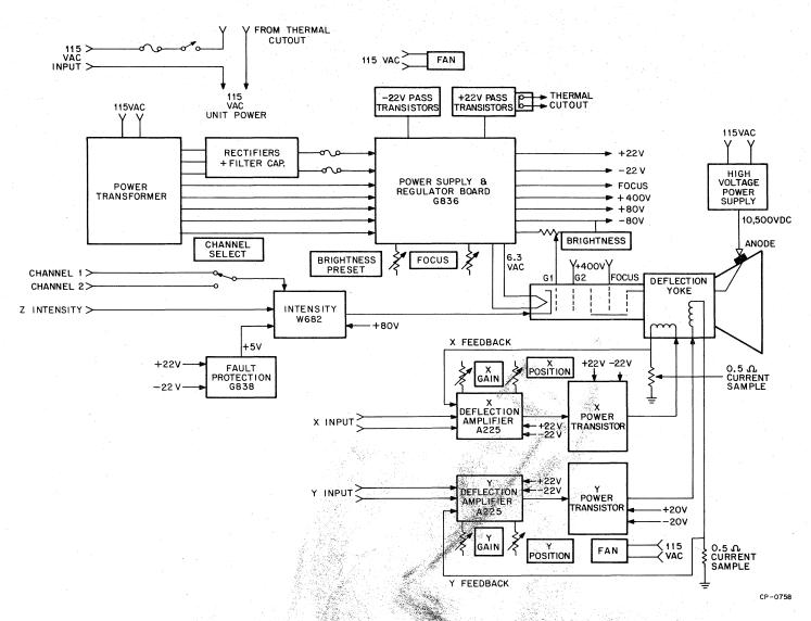
Figure 1-1 Block Diagram of VR14 Without Light Pen Option
