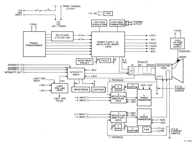
Figure 1-2 VR14L/VR17L Block Diagram
