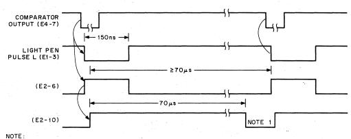
1. This output must be low before a second LIGHT PEN PULSE L signal can be asserted.
