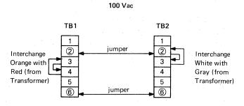
Figure 2-1 Input Power Jumper
