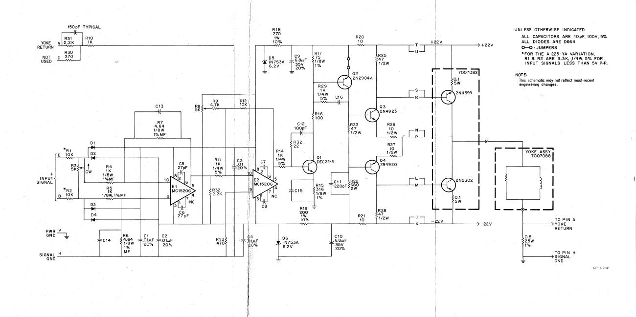
Figure 3-1 X and Y Deflection Circuit
