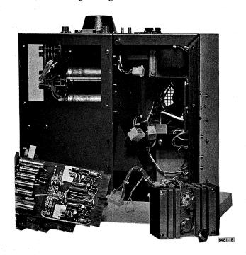
b. Lift heat sink straight out and repair faulty transistor.
