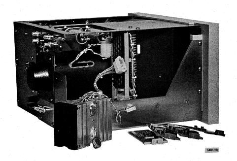
b. Remove heat sink assembly (and its connectors if necessary) and remove faulty power transistor.
