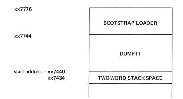
The DUMPAB program (for systems with a switch register) is 65(10) words long. When used in absolute format the storage map is:
