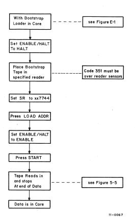
Figure F-2 Loading Bootstrap Tapes into Core
