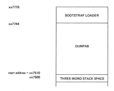
The DUMPAB program (for systems without a switch register) is 82(10) words long. When used in absolute format the storage map is:
