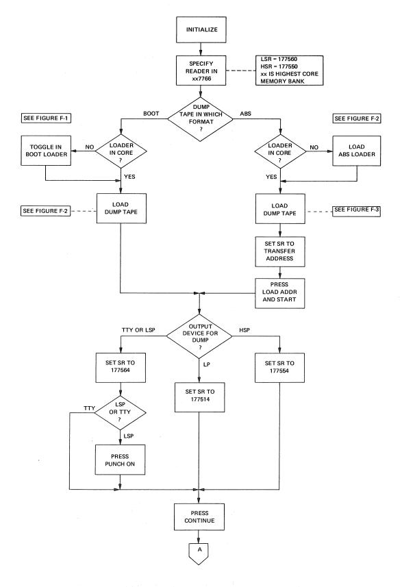
Figure F-4 Dumping Using DUMPAB or DUMPTT
