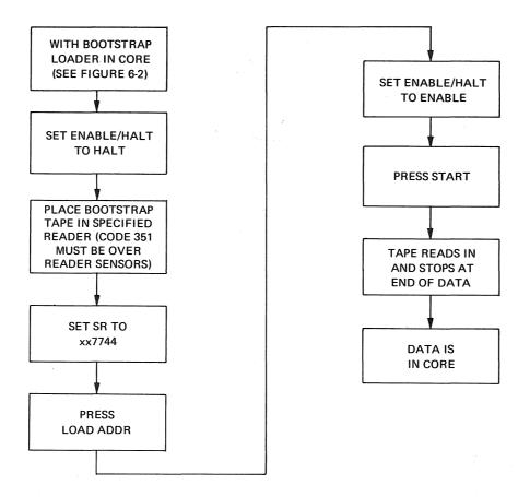
Figure 6-3 Loading Bootstrap Tapes Into Core
