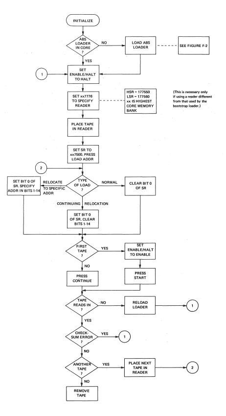
Figure F-3 Loading with the Absolute Loader
