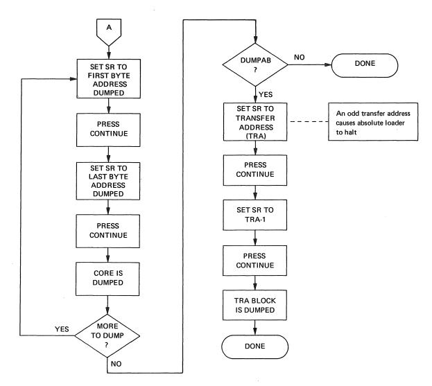
Figure F-4 (continued). Dumping Using DUMPAB or DUMPTT
