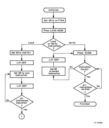
Figure F-l Loading and Verifying the Bootstrap Loader
