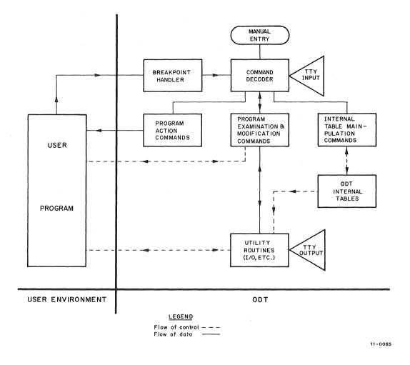
Figure 5-1 Communication and Data Flow
