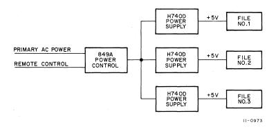
Figure 4-2 UDC11 Logic Cabinet Power Distribution Block Diagram
