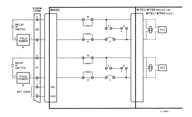
Figure 4-32 Isolated Power for Contact Sensing, Wiring Diagram
