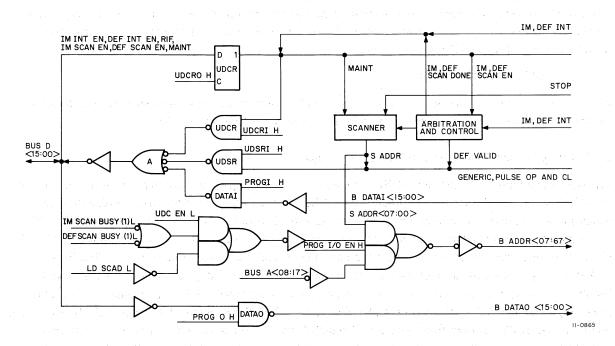
Figure 3-3 Address and Data Gating Logic
