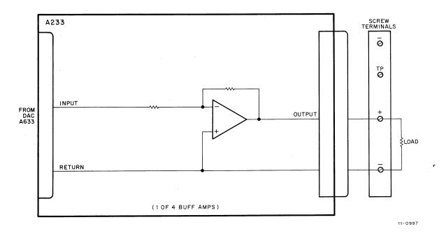
Figure 4-56 Simplified Schematic Diagram (A233)
