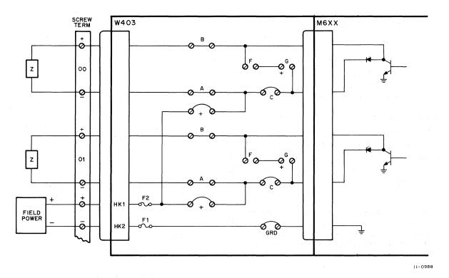
Figure 4-41 Common Power for Driver Output Wiring Diagram
