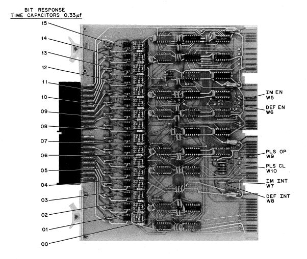
Figure 4-15 Location of Jumpers and Bit Response Time Capacitors (W743)
