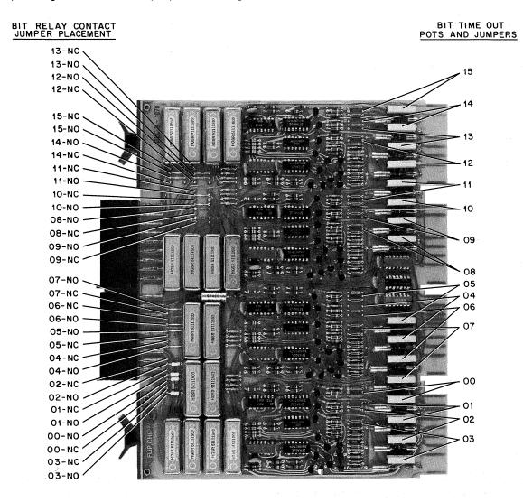
Figure 4-24 Location of Bit Time-out Pots and Jumpers and Relay Contact Jumpers (M807)
