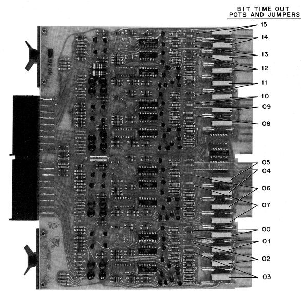
Figure 4-18 Location of Bit Timeout Pots and Jumpers (M687)
