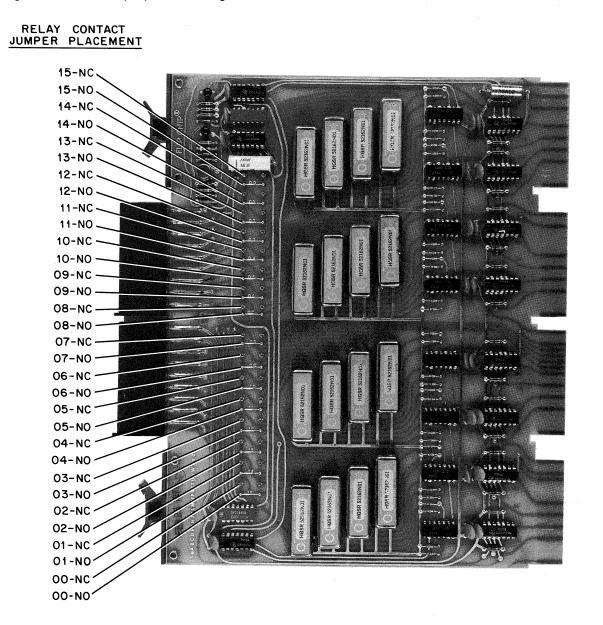
Figure 4-20 Location of Bit Relay Contact Jumpers (M803)
