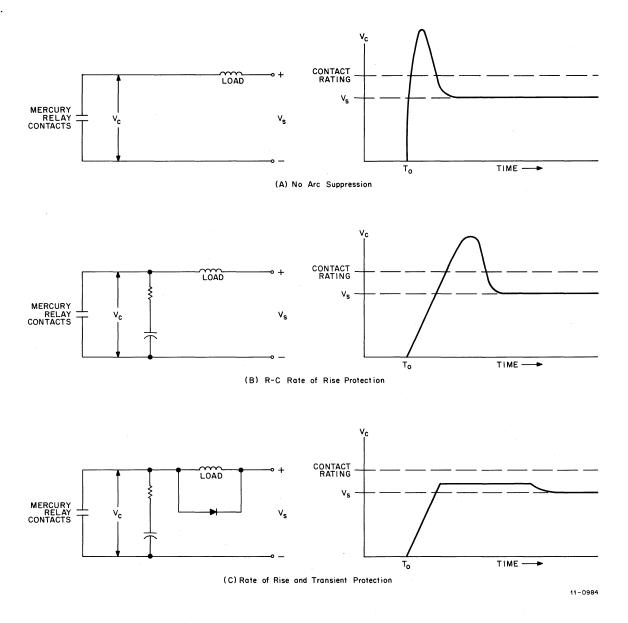
Figure 4-37 Arc Suppression Circuit Characteristics
