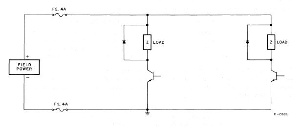
Figure 4-42 Common Power for Driver Output, Schematic Diagram
