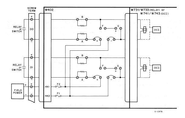
Figure 4-30 Common Power for Contact Sensing, Wiring Diagram
