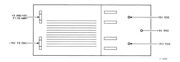
Figure 5-1 H740 Power Supply Fuses and Adjustment Controls
