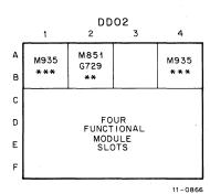
Figure 1-3 DD01-D and DD02 Configuration Diagram
