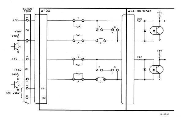
Figure 4-34 Logic Level (RTL) Input, Wiring Diagram
