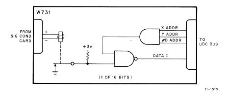
Figure 4-9 Simplified Schematic Diagram (W731)
