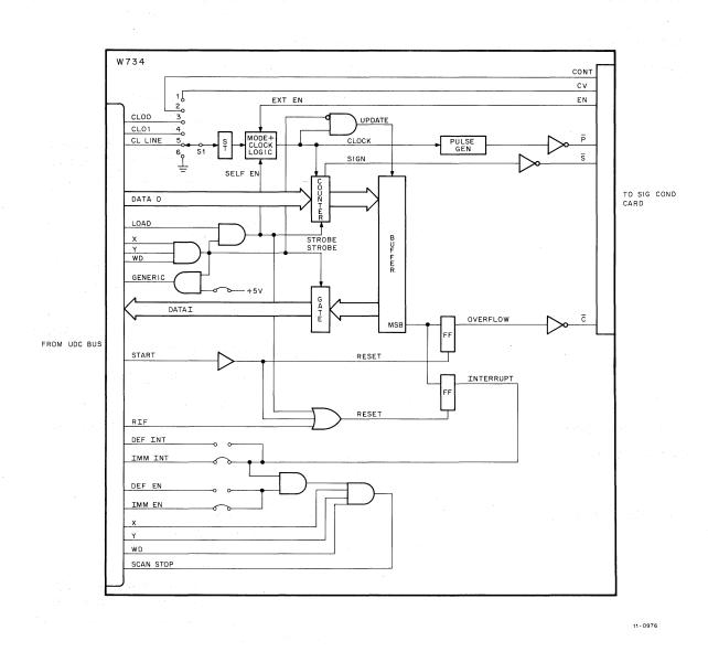
Figure 4-27 Simplified Schematic Diagram (W734)
