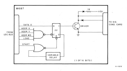
Figure 4-17 Simplified Schematic Diagram (M687)
