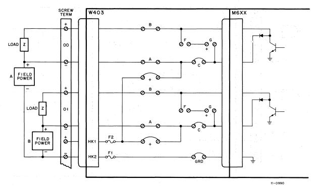
Figure 4-43 Isolated Power for Driver Output Wiring Diagram
