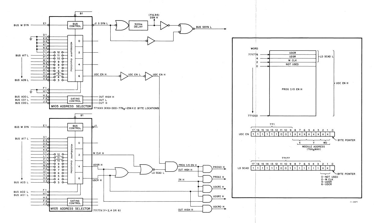
Figure 3-2 Address Selector Logic
