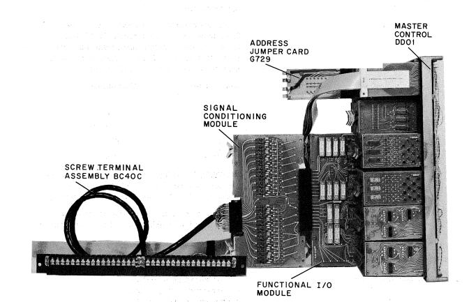
Figure 1-4 UDC11 Assembly Details
