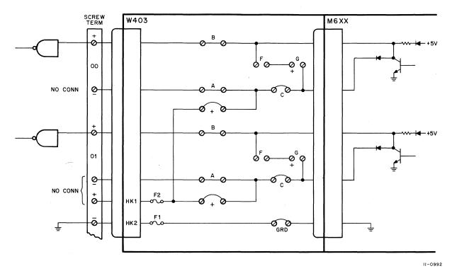
Figure 4-45 Logic Level Output, Wiring Diagram
