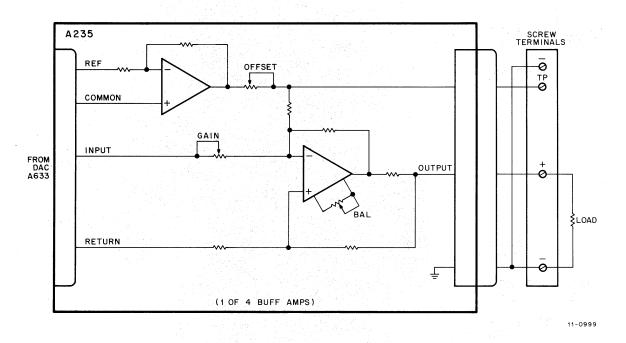
Figure 4-59 Simplified Schematic Diagram (A235)
