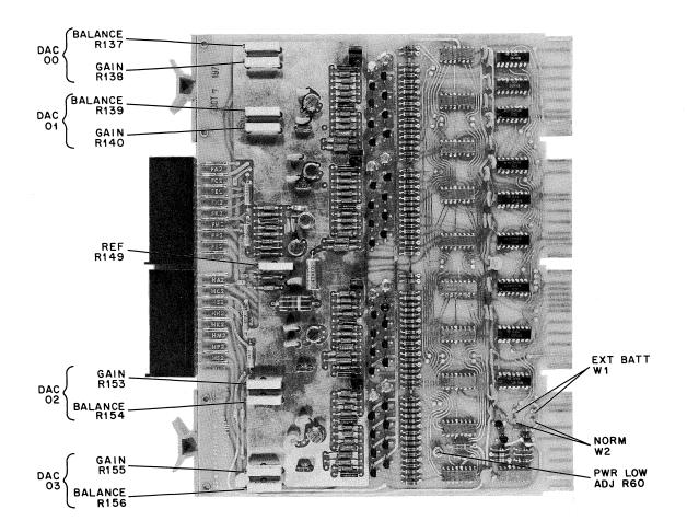
Figure 4-26 Location of Adjustments and Jumpers (A633)
