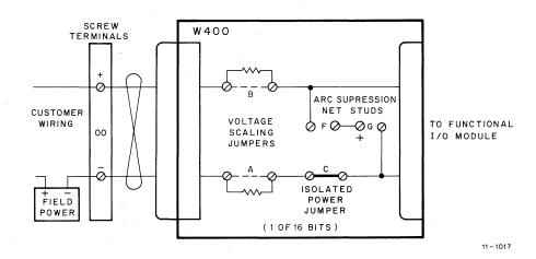
Figure 4-50 Simplified Schematic Diagram (W400)
