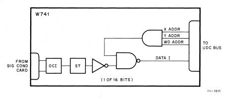
Figure 4-12 Simplified Schematic Diagram (W741)
