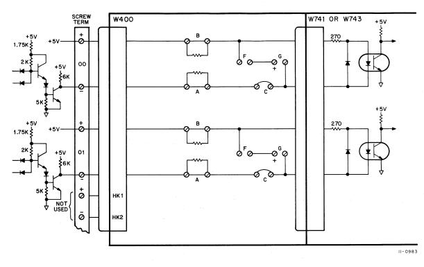
Figure 4-35 Logic Level (DTL) Input, Wiring Diagram
