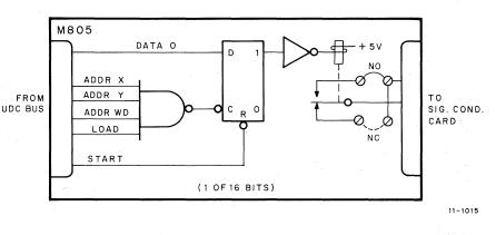
Figure 4-21 Simplified Schematic Diagram (M805)
