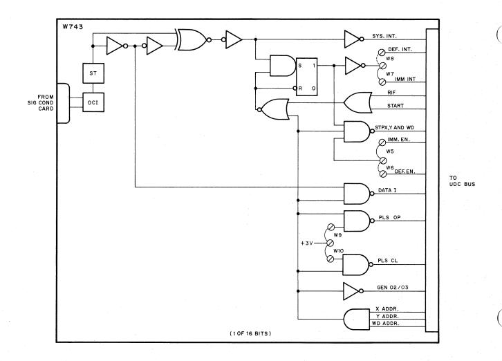
Figure 4-14 Simplified Schematic Diagram (W743)
