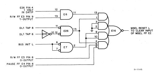
Figure 3-26 Generation of MSEL RESET L
