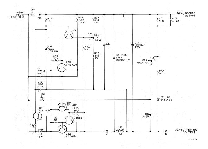
Figure 2-11 –15V Regulator Circuit
