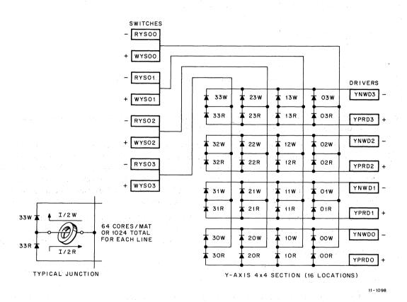
Figure 3-16 Y-Line Selection Stack Diode Matrix
