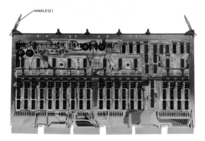
Figure 3-2 Component Side of Drive Module G231
