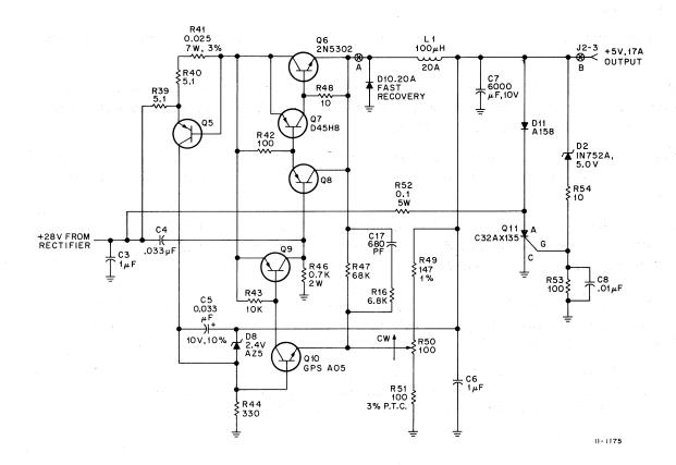
Figure 2-10 +5V Regulator Circuit
