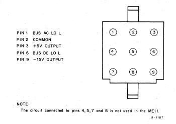
Figure 2-3 H740 Output Connector (5409728 Regulator Module)
