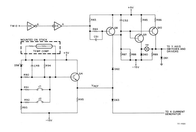
Figure 3-19 Y-Current Generator and Reference Voltage Supply
