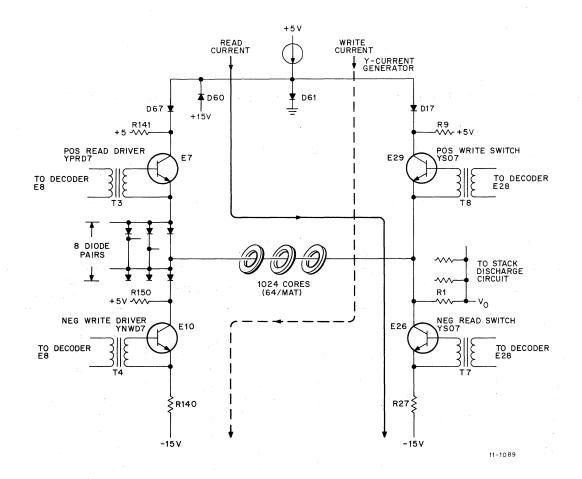
Figure 3-17 Typical Y-Line Read/Write Switches and Drivers
