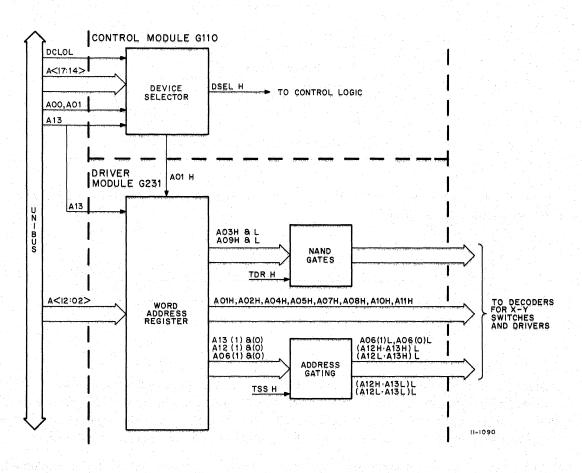
Figure 3-8 Device and Word Address Selection Logic, Block Diagram
