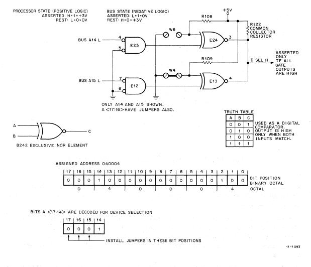
Figure 3-11 Jumper Configuration for a Specific Memory Address
