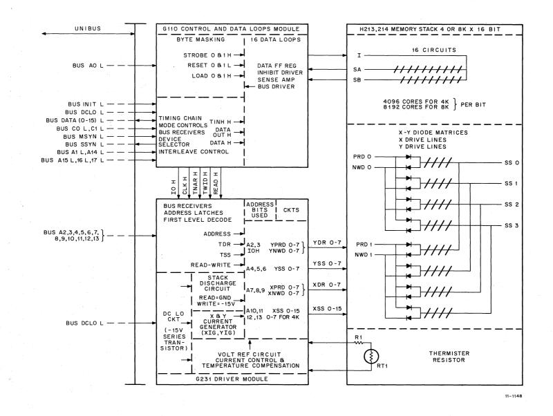
Figure 3-4 MM11-L Memory Block Diagram
