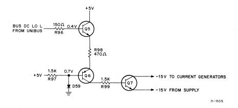
Figure 3-23 DC LO Circuit, Schematic Diagram
