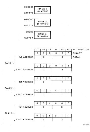
Figure 3-10 Address Assignments for Three Banks of 8K Words Each
