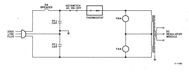
Figure 2-6 230V Connection, Simplified Schematic Diagram
