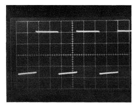
c) Point C, 5A load, 50 μs/div, and 10V/div.
