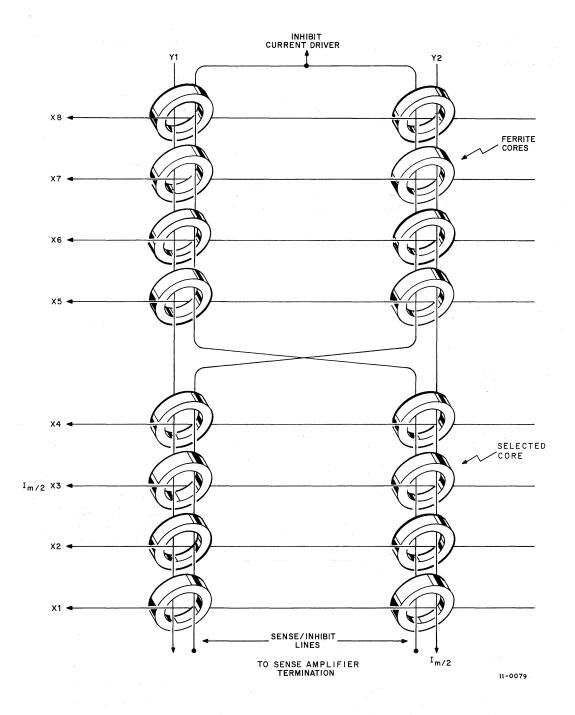
Figure 3-5 Three-Wire Memory Configuration
