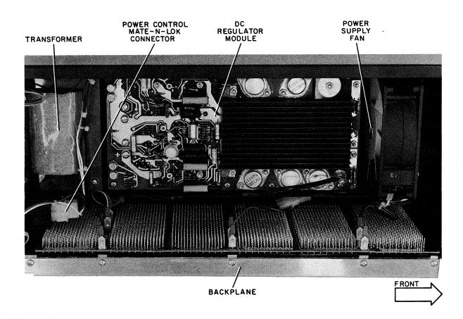
Figure 1-6 Power Supply Section of ME11-L
