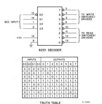
Figure 3-13 Type 8251 Decoder, Pin Designation and Truth Table
