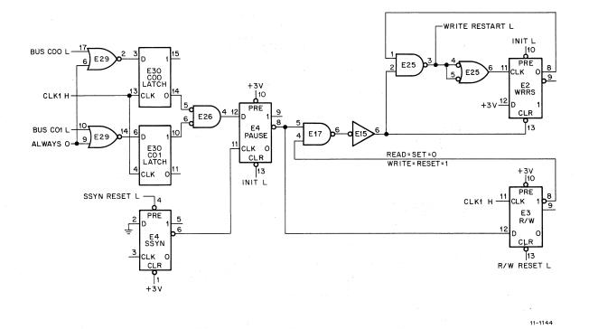
Figure 3-28 Pause/Write Restart Circuit
