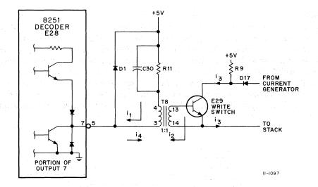
Figure 3-15 Switch or Driver Base Drive Circuit
