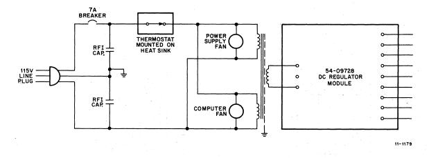
Figure 2-5 115V Connections, Simplified Schematic Diagram
