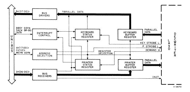
Figure 2-1 LC11 Controller - Simplified Block Diagram
