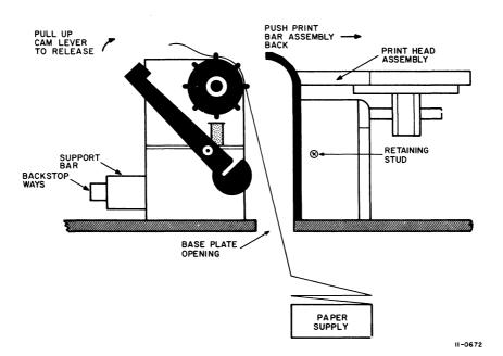
Figure 3-2 Loading Paper into LA30 DECwriter
