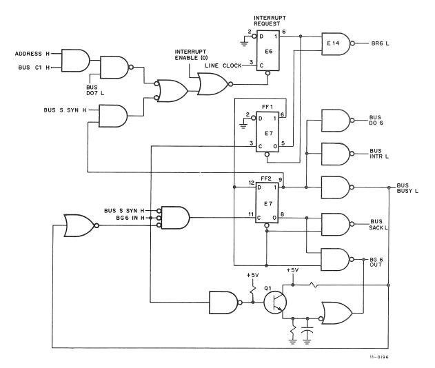
Figure 3-2 Interrupt Request Section, Simplified Logic Diagram
