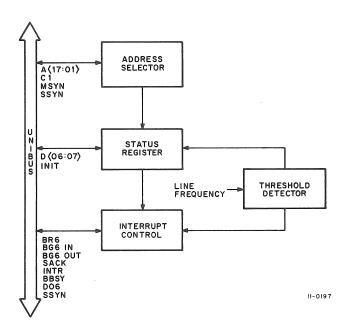
Figure 2-1 KW11-L Block Diagram
