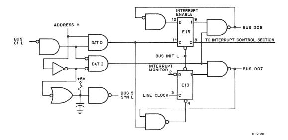
Figure 3-3 Status Register, Simplified Logic Diagram
