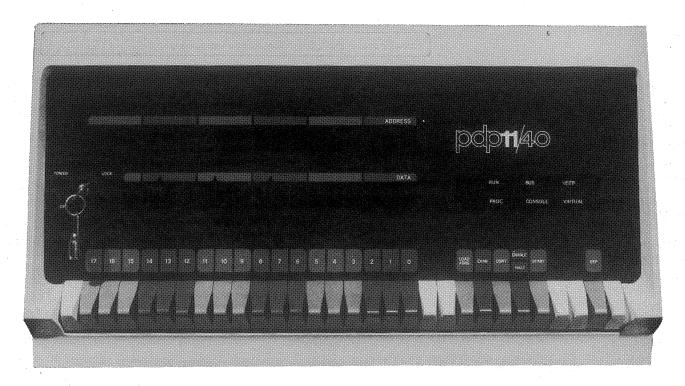
Figure 2 PDP-11/40 Programmer's Console
