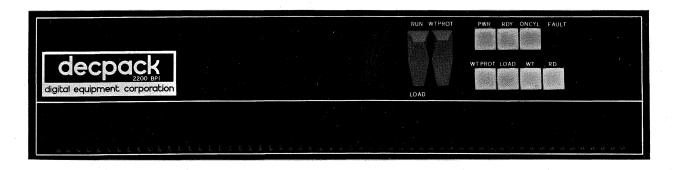
Figure 4 RK05 Controls and Indicators
