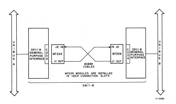
Figure C-1 Block Diagram of PDP-11 DMA Interprocessor Channel
