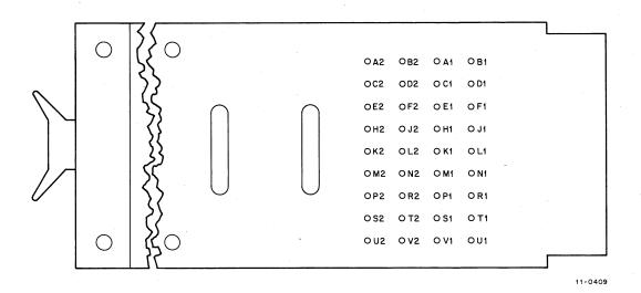
Figure B-1 M957 Cable Connector Pinning Detail
