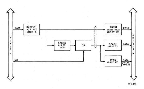
Figure C-3 Cross-Interrupt Block Diagram
