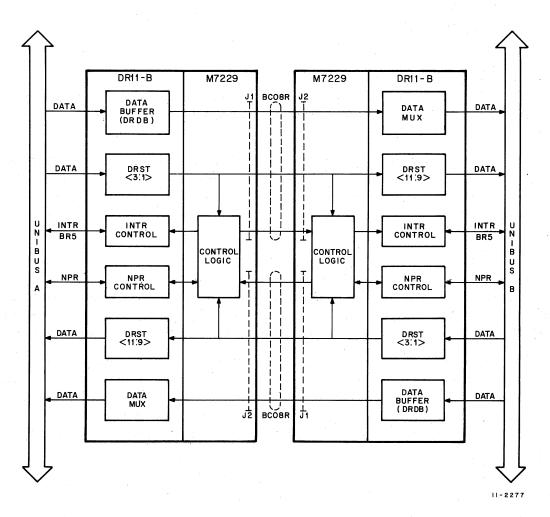
Figure C-2 DMA Interprocessor Channel Functional Block Diagram
