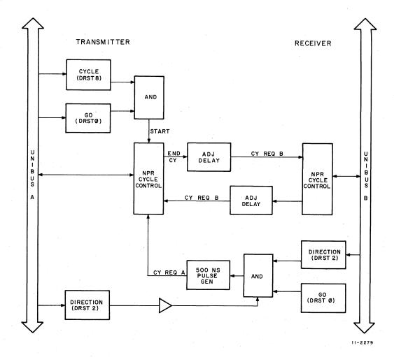
Figure C-4 NPR Interlocking Control Block Diagram
