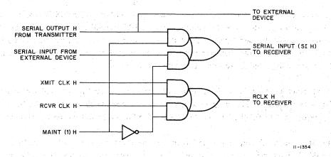
Figure 5-9 Maintenance Logic – Simplified Diagram
