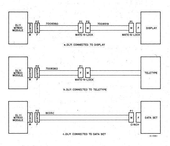
Figure 3-3 DL11 Cable Connections
