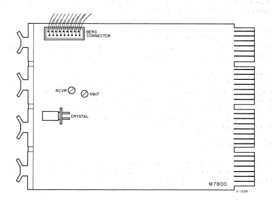
Figure 2-4 Crystal and Switch Location
