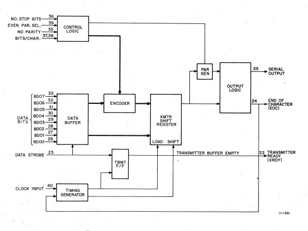
Figure 5-6 UART Transmitter – Block Diagram
