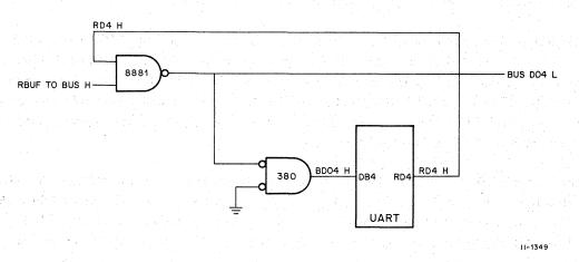
Figure 5-4 RBUF and XBUF Gating Logic – Simplified Diagram (one bit position)
