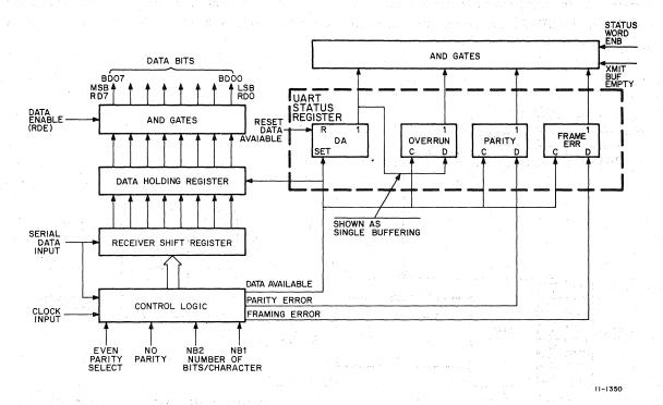
Figure 5-5 UART Receiver – Block Diagram
