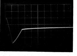
e) Point D, No load, 50 μs/div, and 50 mV/div.
