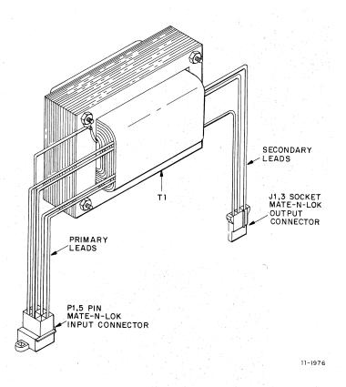
Figure 1-3 Transformer Assembly
