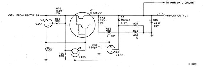
Figure 3-9 +15 V Regulator Circuit
