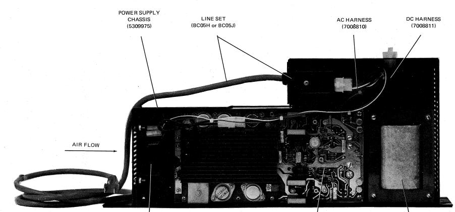
COOLING FAN (1210719) DC REGULATOR MODULE (5409728) TRANSFORMER (7008726)
