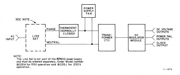
Figure 3-1 Power Supply Block Diagram
