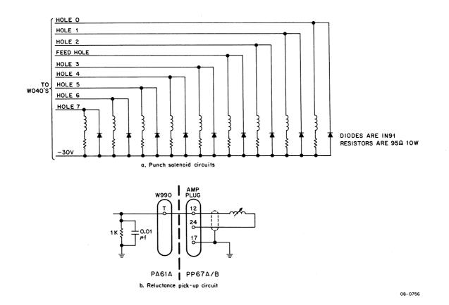
Figure 4-5 Punch Solenoid and Reluctance Pick-up Circuits, Simplified Diagram
