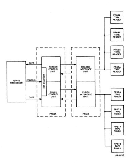
Figure 3-1 Configuration of Typeset-8 System
