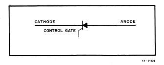
In the OFF condition, an SCR has a high resistance in both directions (for example, 100,000 ohm), the gate to cathode being equivalent to a small diode. Providing the anode voltage is positive with respect to the cathode, if a small positive voltage is applied to the gate, the forward resistance of the SCR will be greatly reduced and current will flow
