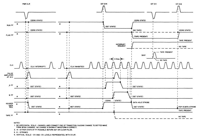
Figure 4-8 Tape Reader Timing Sequence, PA68A Reader/Punch Control Unit
