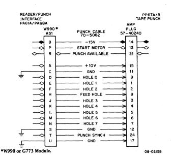
Figure 5-3 Interface, PR68A/B Paper-Tape Reader to PA61A Reader/Punch Interface Unit
