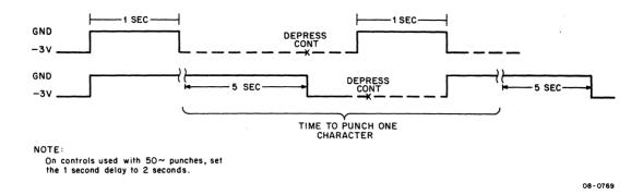
Figure 6-4 1 Second and 5 Second Delay Waveform Relationship
