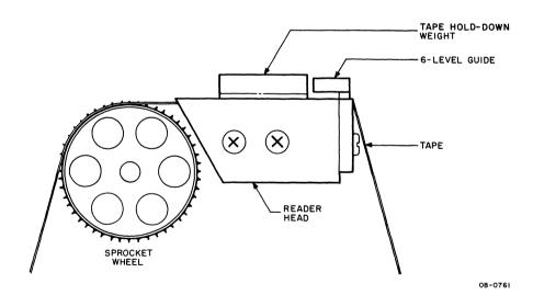
Figure 6-6 6-Level Guide and Reader Head Adjustment
