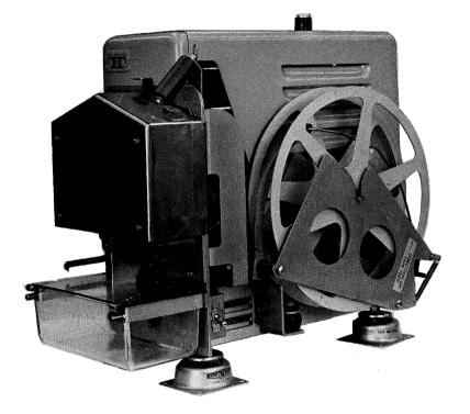
Figure 1-2 PP67A/B High-Speed Paper-Tape Punch
