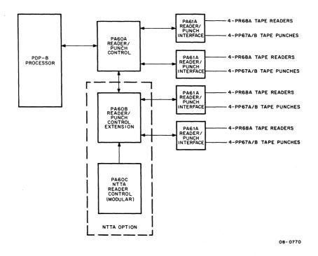
Figure 3-2 Multi-Reader/Punch Configuration with NTTA Option
