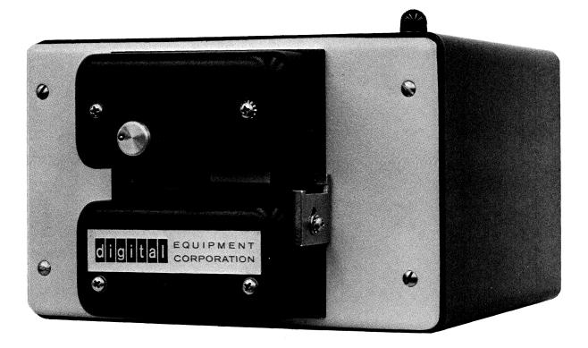
Figure 1-1 PR68A High-Speed Paper-Tape Reader
