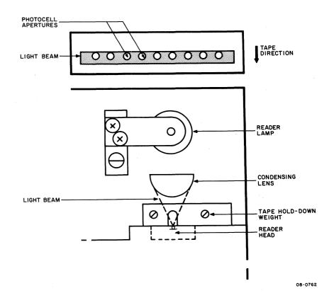
Figure 6-7 Reader Lamp and Condensing Lens Adjustment
