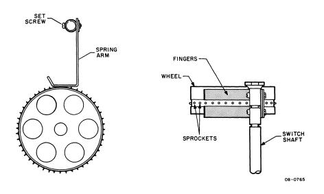
Figure 6-10 Spring Arm Adjustment
