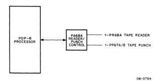
Figure 3-3 Single Reader/Punch Configuration
