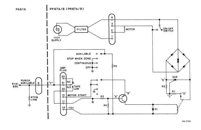
Figure 4-3 PR67A Paper-Tape Punch Control, Simplified Functional Diagram
