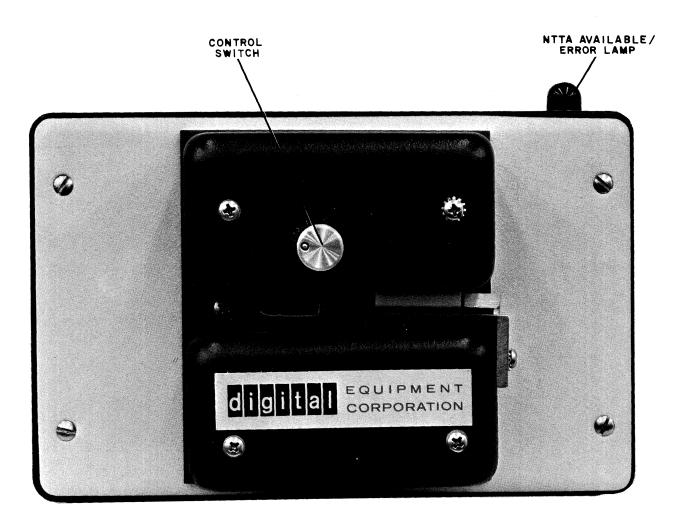
Figure 4-6 PR68A Paper-Tape Reader, Control Switch and Indicator
