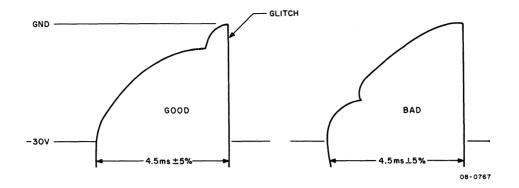
Figure 6-12 Punch Solenoid Waveform
