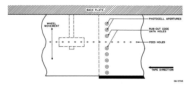
Figure 6-8 Lateral Adjustment of Sprocket Wheel
