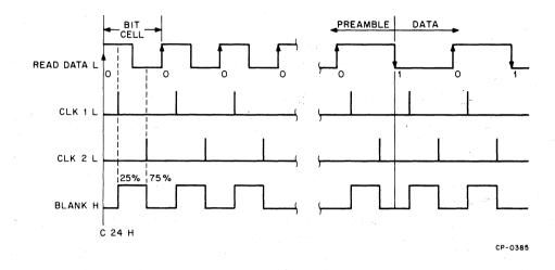
Figure 4-9 Simplified Blank H and Read Clock Timing
