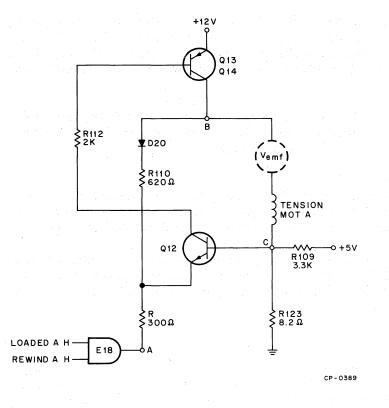
Figure 4-13 Rewind Control Circuit
