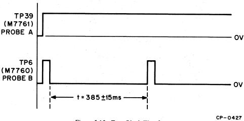
Figure 5-13 Tape Blank Waveform
