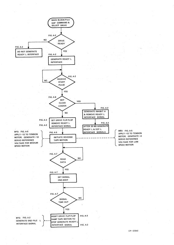
Figure 4-3 Back Block/File Gap Flow Chart
