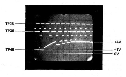
signal is then compared in the phase detector to the incoming PEAKS L pulses. Since the PEAKS L pulses occur at a higher frequency than the initial reference frequency, the PEAKS L pulses lead the reference signal. This condition causes pin 13 of the phase detector to go low, causing pin 5 to also go low for the duration of the time difference between signals (see figure).
