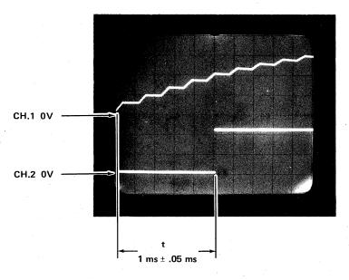
Figure 5-11 Threshold Waveform
