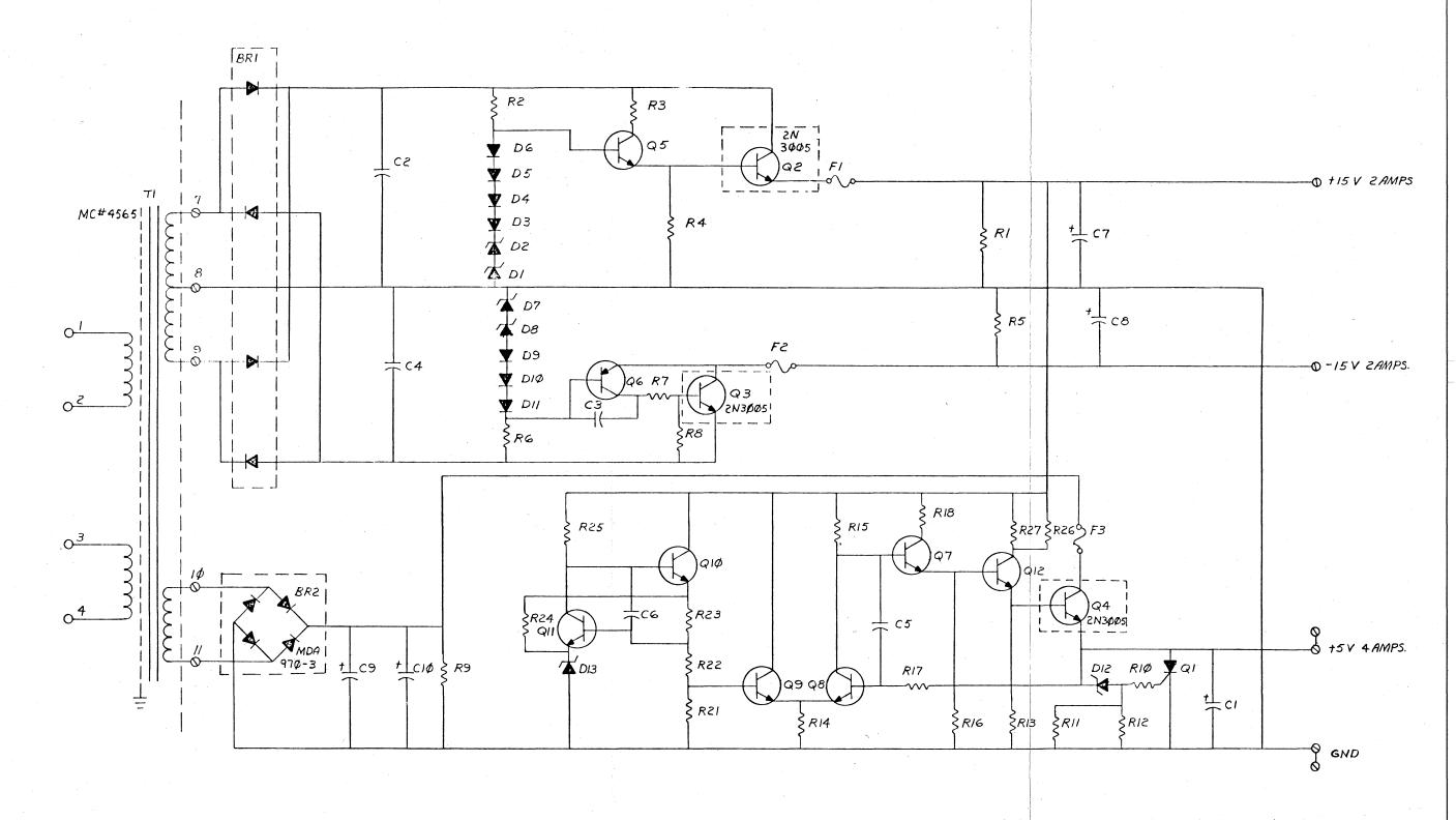
O INDICATES HOLES FOR DIODE BRIDGE Q2,Q3,Q4,BR24 TI ARE MOUNTED ON CHASSIS/HEAT SINK
