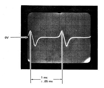
Figure 5-5 Fine Speed Adjustment
