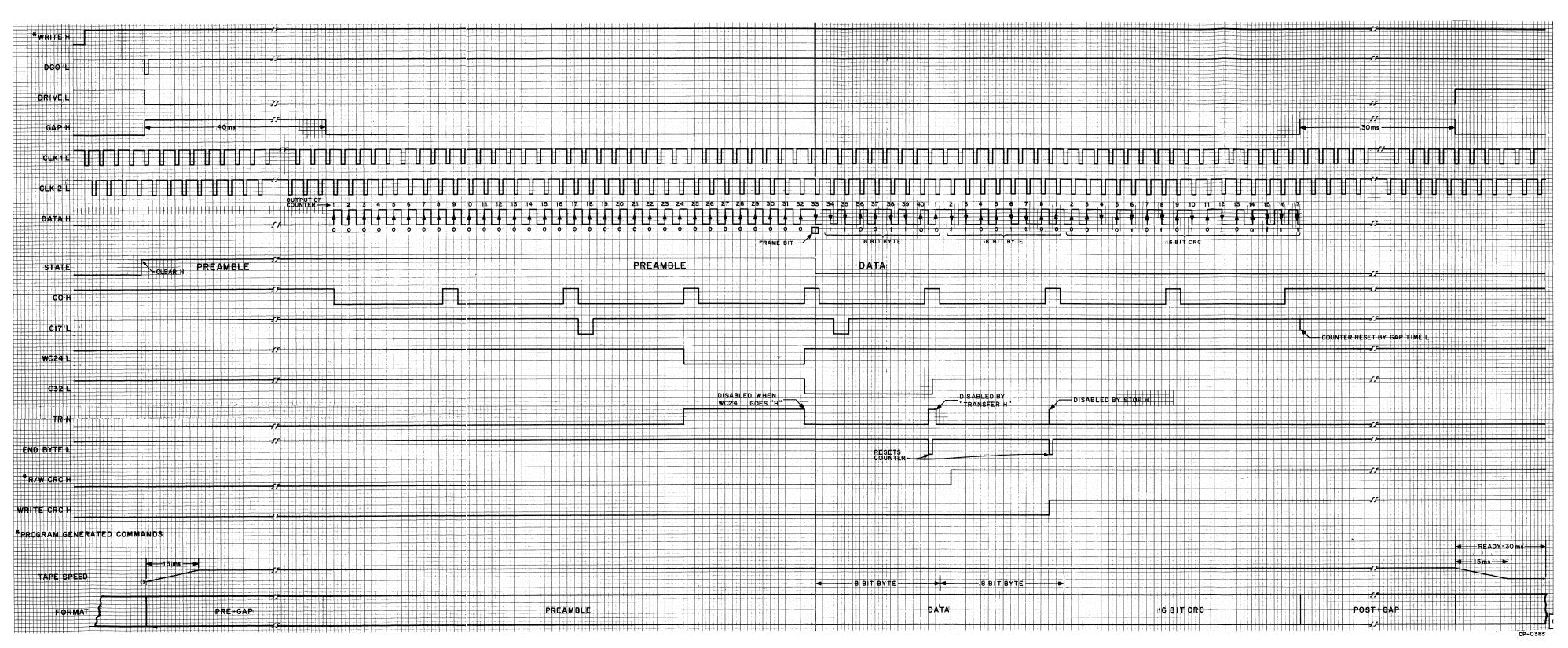
Figure 4-8 Write Timing
