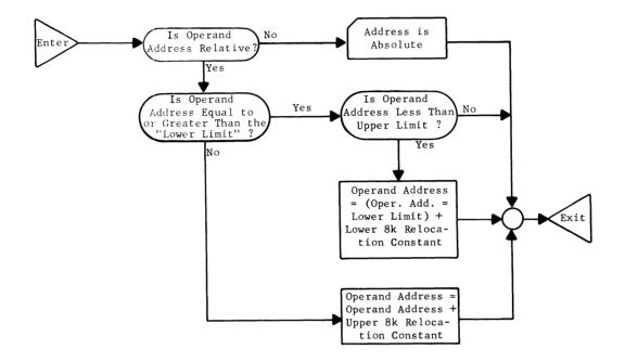
This same logic is used to convert relocatable program word location addresses into the absolute locations in which the program words are stored.
