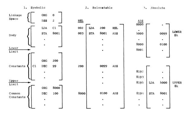
Note that the program constant C1 is loaded into the lower bank absolute location 4000 and the operation address of the upper bank instruction (LDA C1) is changed by the loader to absolute address 4000. The Common Storage constant (DEC 100) is loaded into the absolute address indicated by the ORG 8000 card in the symbolic program since this address is greater than the "upper limit" given on the header card.
