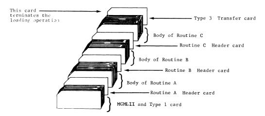
The Type-3 transfer card was produced by General Assembly Program II when Routine A was assembled in relocatable form. It is the last output card from the assembly. The Type-3 card has a 2, 3 punch in column 1. (A Type-5 transfer card was also produced and must be discarded. A Type-5 card has a 1, 3 punch in column 1.)
