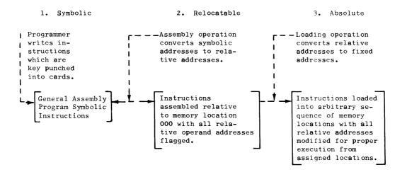
In the illustration below, addresses are modified from symbolic, to relocatable, to absolute in a specific set of GE-200 Series instructions. It is assumed that the loading routine has been instructed to store the relocatable instructions in memory starting at location 200. For ease of reading, operation codes are shown as mnemonics, addresses are shown as decimal numbers, and indexed instructions are indicated by , 2.
