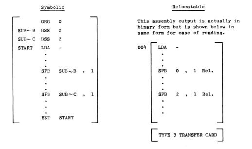
Before Routine A is leaded, a header card is prepared for A, giving the Loading Routine information needed to supply branch instructions connecting Routine A to B and C. The Loading Routine assigns absolute memory addresses to the instructions in Routine A, and supplies the missing Linkage between A and Routines B and C. Routines B and C are then loaded with Routine A.
