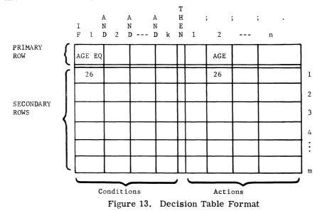
A condition is a relation between a variable appearing in a primary block and an operand appearing in a corresponding secondary block. For example, AGE may be written in primary block 1 and EQ 26 may be written in secondary block 1. In this way a condition is stated and the question "if age equals 26" is asked.
