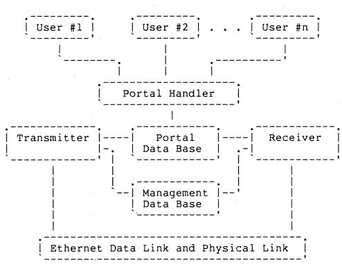
The Portal Handler maintains the Portal Data Base according to user requests through the User Interface. The Portal Handler communicates with the Transmitter and Receiver through the Portal Data Base. The Transmitter and Receiver send and receive frames through the DNA Ethernet Data Link User Interface and maintain counter and event information in the Management Data Base.
