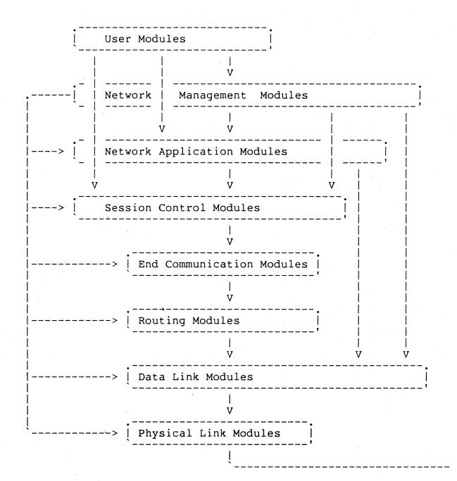
The DNA Ethernet Data Link resides within the DNA Data Link layer. It can be co-resident with other DNA Data Link modules such as DDCMP or X.25.
