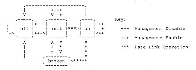
Network management can enable the channel. From the "off" or "broken" states, this enable causes a transition to "init". From the "on" state, enable has no effect.
