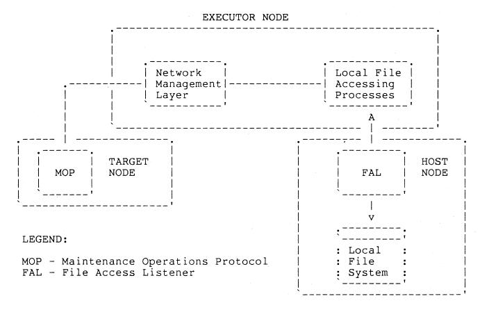
Figure 7B. Down-Line Load Remote File Access Operation
