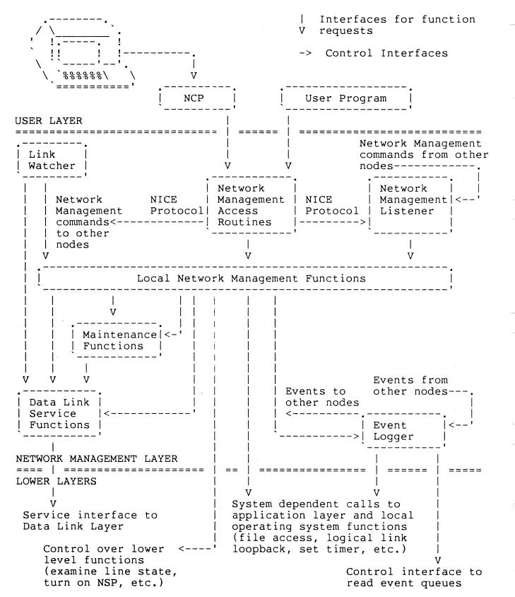
Figure 2. Network Management Layer Modules and Interfaces in a Single Node.
