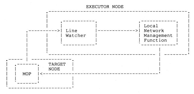
Figure 8A. Target-Initiated Down-Line Load Request Operation
