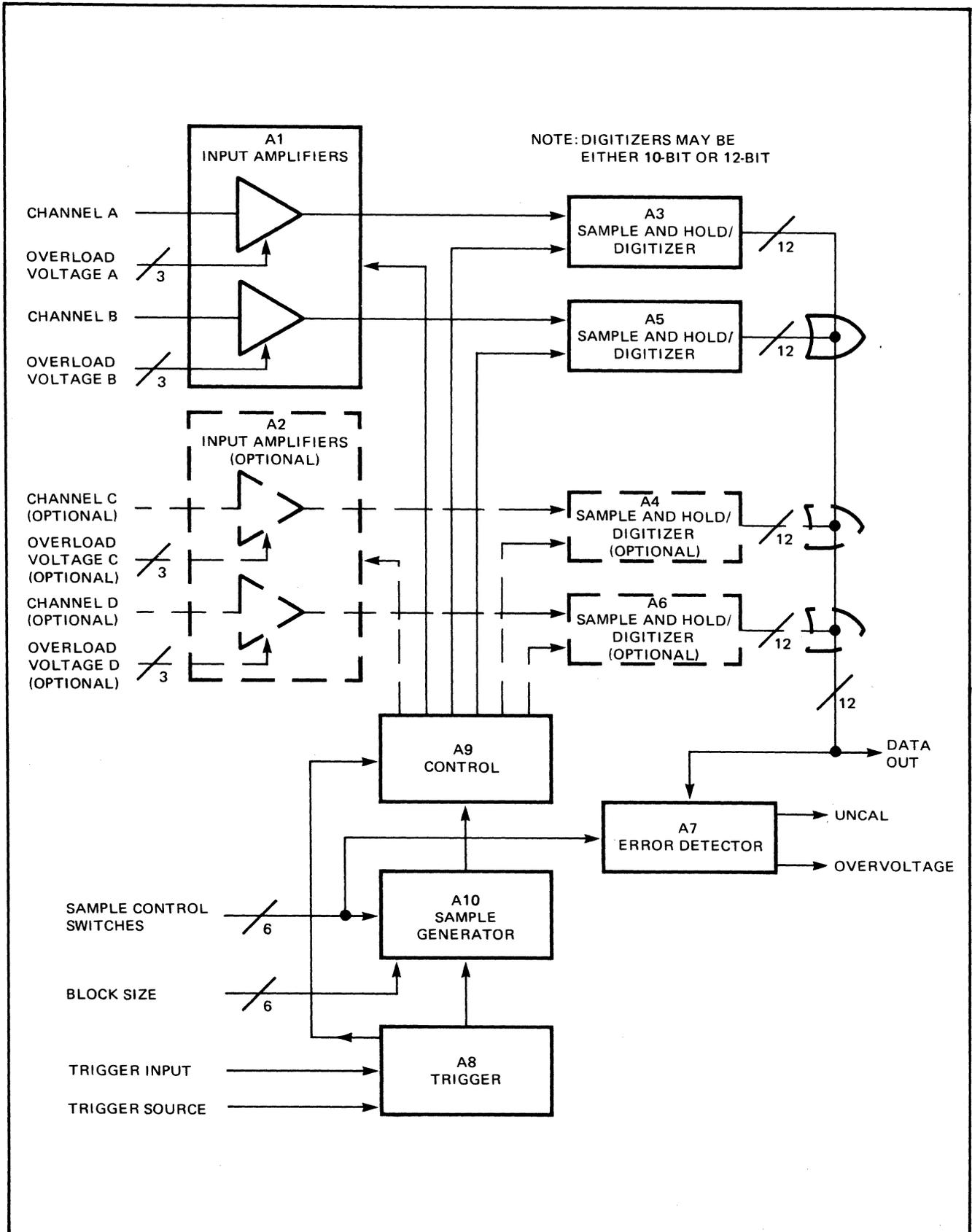
Figure 2-2. ADC Input/Output Signals
