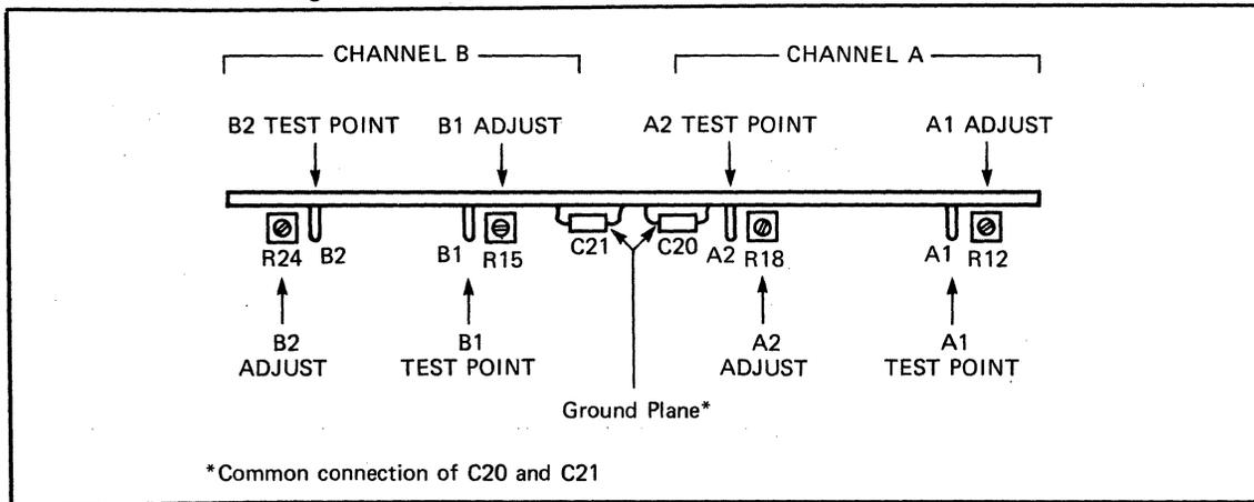
2. Connect the Voltmeter's Ground lead to ground on the board under test. (The best way to do this is to connect it to any component lead that is connected to the board's ground plane.)
