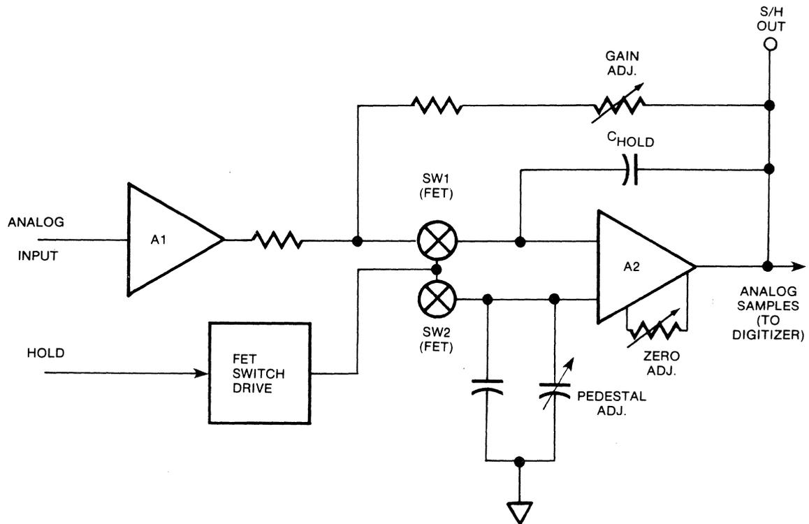
Figure 2-5c. ADC Circuit Block Diagram (05466-60014)
