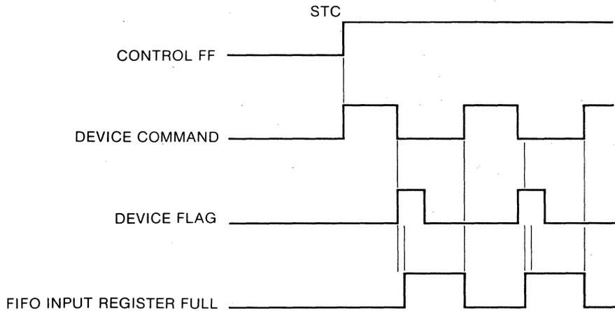
Since device command is not under direct control of STC instruction as is common, if the input operation is under the control of DMA it is possible to have more device commands issued to the device than the number of words required to satisfy the DMA transfer request. This can occur since DMA can not issue a CLC to clear the Control FF until it has taken out of the FIFO the required number of words.
