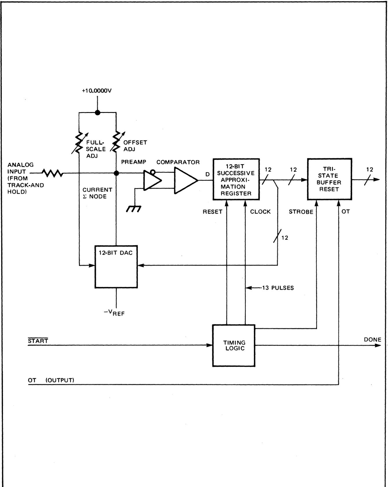
Figure 2-5d. DAC — Block Diagram (05466-60014)
