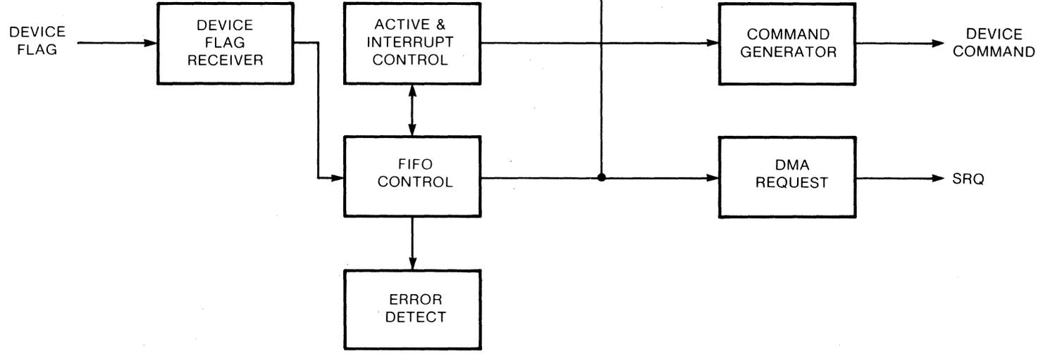
Figure 2-9a. High Speed ADC Interface Block Diagram
