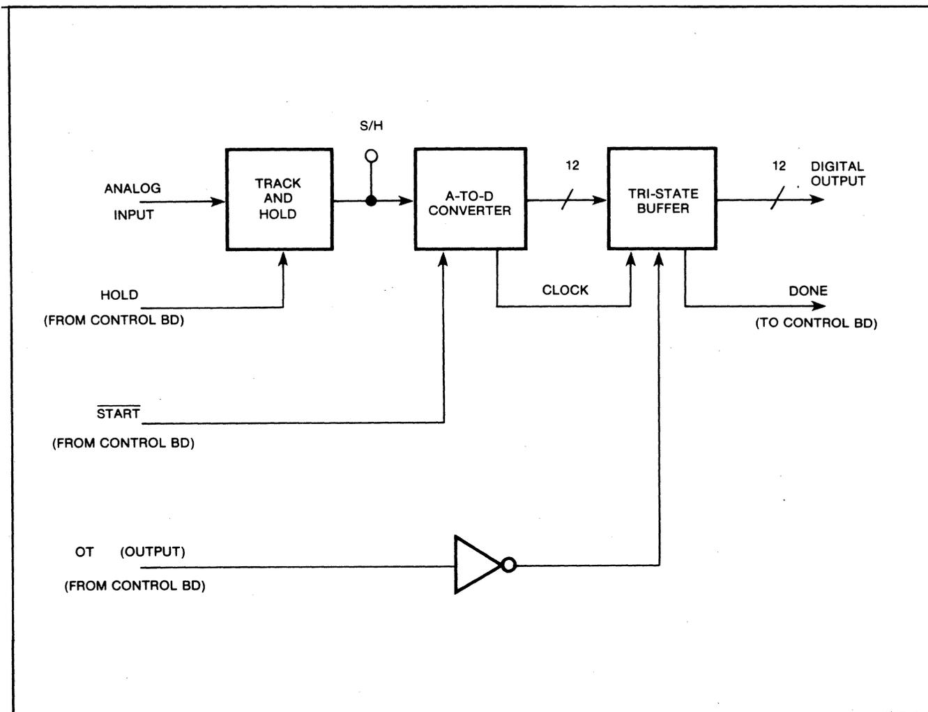
Figure 2-5b. Track-and-Hold Circuit—Block Diagram (05466-60014)
