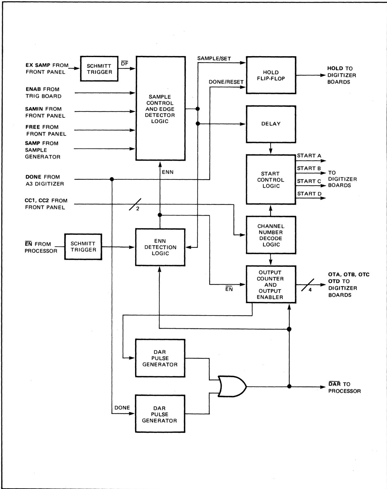
The sample pulses, after passing through the Sample Control and Edge Detector Logic, set the HOLD flip-flop. The HOLD command is sent to all digitizer boards. The sample pulses are delayed and used to send the START command to the appropriate digitizer board. Depending on the “number of input channels” information encoded on the lines “CC1” and “CC2”, the START command is sent to 1, 2, 3, or 4 boards, as indicated in Table 2-5.
