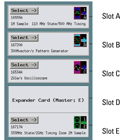
If a module is in Slot A, then its pods begin with "A", such as "A1".
