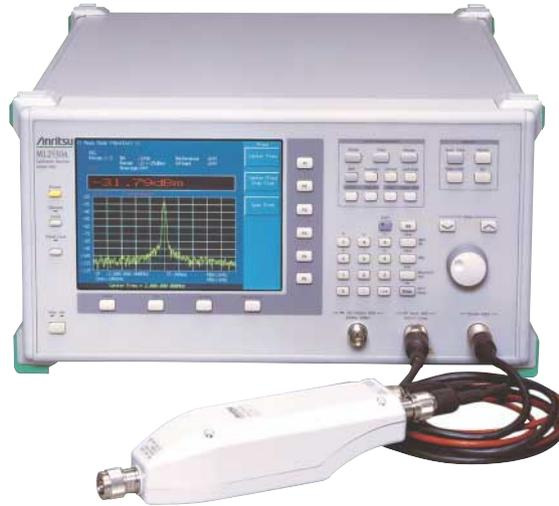
The ML2530A is a receiver for calibrating the output power level of such devices as signal generators and attenuators, covering the range of 100 kHz to 3 GHz. It is suitable for use as a reference level meter for the RF communications bands used by the world's mobile communications markets. High linearity is achieved by using a level detector that uses DSP technology. The level can be measured while observing the signal waveform to be measured by using the spectrum monitor function.
