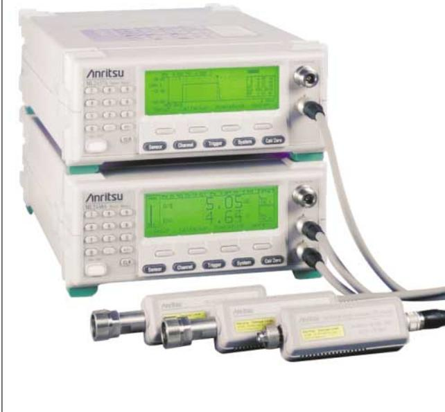
The ML2430A series Power Meters combine the advantages of thermal meter accuracy, diode meter speed, and peak power meter display graphics. The result is a single instrument that achieves 90 dB dynamic range with a single sensor. The ML2430A series includes graphics display capability as a standard feature. The ruggedized housing and optional high-capacity NiMH battery bring convenience and accuracy to field service applications.
