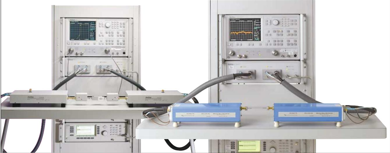
The ME7808B Broadband Vector Network Analyzer (VNA) is a high performance measurement solution that covers 40 MHz to 110 GHz in a single fast sweep. Built on the advanced technology of the Lightning 65 GHz VNA, the ME7808B is ideal for making accurate S-parameter measurements of components and devices to 110 GHz. The flexible system architecture of the ME7808B makes it easy to adapt to multiple measurement applications.
