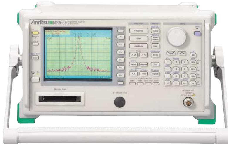
The MS2663C covers a frequency range of 9 kHz to 8.1 GHz. This allows measurement of spurious frequencies of up to three times greater than the frequency bands used worldwide for mobile communications. The MS2663C has superior basic performance such as high C/N ratio, low distortion, and high frequency/level accuracies and is easy to operate.
