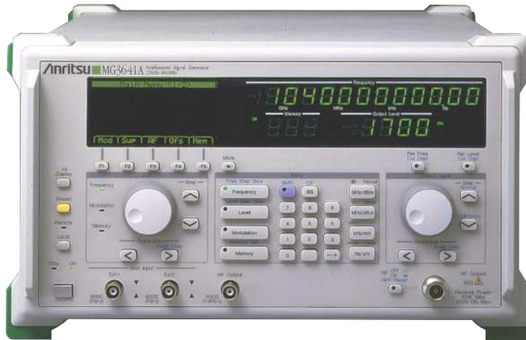
The frequency of MG3641A/3642A is set with a resolution of 0.01 Hz across the full frequency ranges, and the non-harmonic spurious is better than  $-100$  dBc for reliable measurement at any frequency. A low-noise YIG oscillator produces a high-purity signal with SSB phase noise of better than  $-130$  dBc/Hz (1 GHz, 20 kHz offset) making these signal generators ideal for interference testing of radio receivers and as sources for various local and reference signals.
