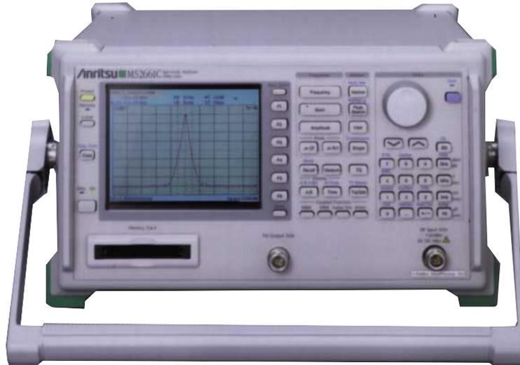
The MS2661C Portable Spectrum Analyzer is for signal analysis of radio and other equipment related to improving frequency usage efficiency, higher modulation, and digitalization. The MS2661C is a synthesized spectrum analyzer covering a wide frequency range from 9 kHz to 3 GHz and it has superior basic performance such as high C/N ratio, low distortion, and a high frequency/level accuracies.
