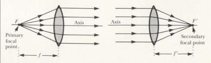
Figure 1. Two views of a thin lens with rays from and to F and F', respectively.
