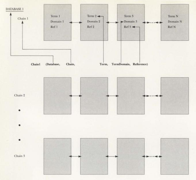
Figure 1. Structure of chains in the external database.
