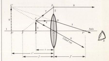
Figure 3. Placement of an object between the focal point and the lens, creating a virtual image.
