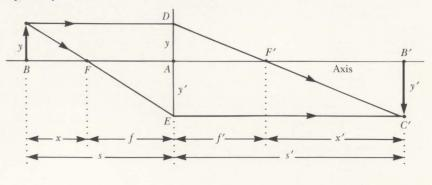
to the image of height y'. Let *s* represent the object distance from the center of the lens and let s' represent the image distance from the center of the lens. *x* represents the object distance from the focal point *F*, and *x'* represents the image distance from focal point *F'*.
