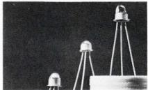
Type QS-507 is for general purpose computer and industrial applications that require light sensitivities 10 to 20 times those of normal photo transistors. It provides light current of 5.0 mA with irradiance of only 2.0 mW/cm<sup>2</sup>. Is sensitive to both visible and near I-R illumination. 45c (1,000 quan.). Quantum Sensing, Inc., 1650 Locust Ave., Bohemia, N.Y. 11716.
