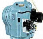
Stripper/crimper machine strips wire and attaches open barrel terminal during each machine cycle. Capacity: 1500 terminations per hour.
