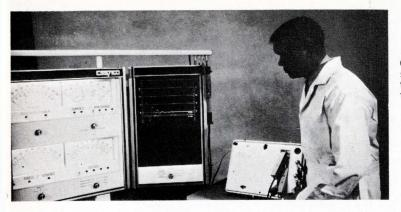
**Clayton's dynamometer** includes electronic instrumentation amplifiers for the panel meters. The electronic circuitry is packaged in rugged modules to withstand the service shop environment and to simplify service.
