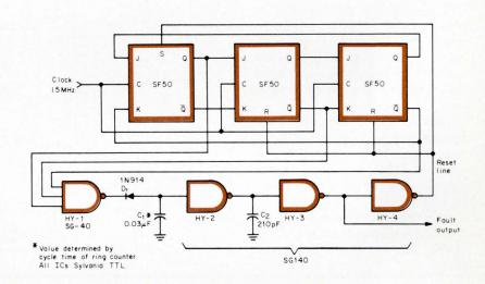
reaches the logic threshold level, HY-2 sends a logic  $\theta$  through HY-3 and HY-4 to reset the counter. This, in turn, forces HY-1's output to drop to a  $\theta$  and discharge  $C_1$  through  $D_1$ . The input to HY-2 thus drops below threshold, removing the reset pulse.
