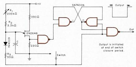
first gate which, in turn, SETs the flip-flop with a negative signal. The output is again HIGH.
