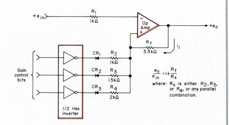
(about 5 or 6 V), then the diode in series with that output is reverse biased, and the associated resistor is not in the gain control loop.
