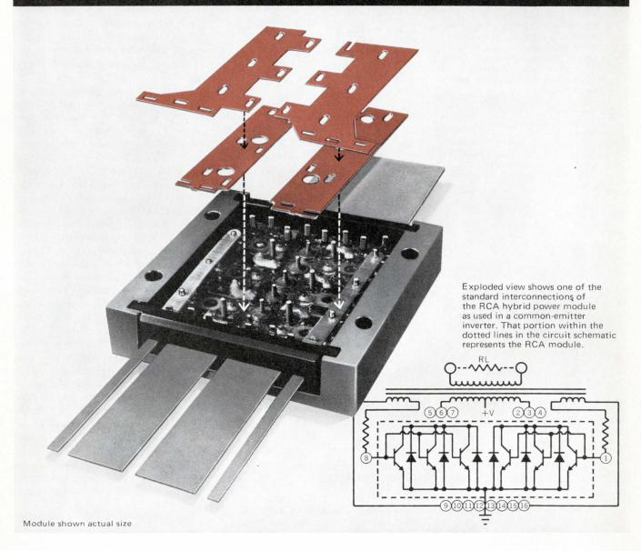
Take RCA transistor chips with current capabilities up to 80 A, rectifiers with peak currents to 80 A, and resistors to 10 watts. Interconnect them — in any number of ways. What do you get? A power capability up to 800 W, current capability up to 300 A!
