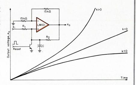
ous powers by adjusting the ratio of  $R_1$  to  $R_2$ .
