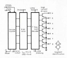
MC4050 Counter-Latch-Decoder. Resetting the input suppresses the leading zeroes in a display. The lamp blanking input allows control of display brightness through control of the duty cycle, and a lamp test input permits verification of all diode integrity.
