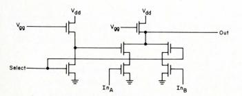
Fig. 9. Data selection structure for static shift registers. This circuit produces an inversion of the desired information which it must be corrected later in the register. The circuit shown is for static registers, but it can be used in slower dynamic registers also. Other variations can be constructed for modifications of inverters shown in the dynamic shift register section.
