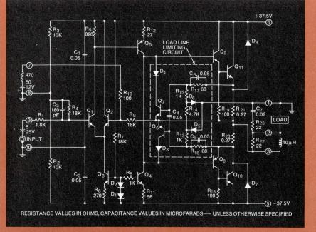
Schematic diagram of unencapsulated TA7625
