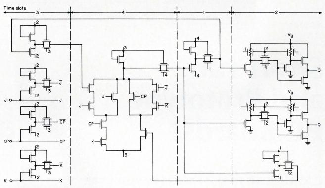
Fig. 10. Schematic diagram of JK flip-flop.
