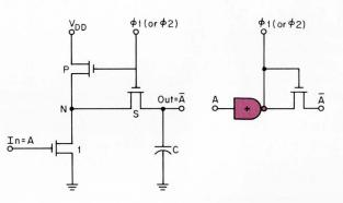
Fig. 4. The ac inverter. This logic gate shows the standard application of the three basic functions of MOS devices; the pull-up and coupling (series) devices are clocked at the same instant by a common phase, while the pull-down device is activated by the data (input).
