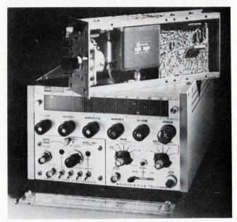
The Gunn Effect diode, operating from 8 to 12.4 GHz, is used by Kruse Electronics in their new microwave sweeper. Oscillator by Varian can be seen in the unit above.
