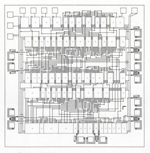
Computer generated interconnection layout for a four-bit counter.
