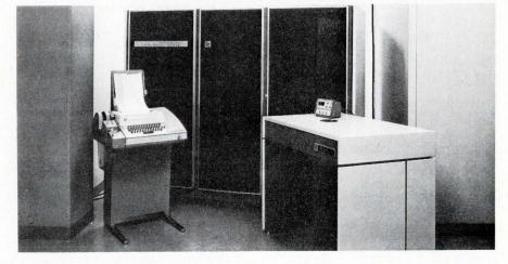
test station during the test sequence. Each lead of the IC may be independently connected to power supplies (three voltage supplies and one current source), signal sources (two pulse generators), load networks or buffer drive circuits (48 total), and measurement probes (16 sampling heads) as required. Voltage and current forcing capabilities (dc) are 0 to  $\pm 100$  V, and  $\pm 1$  mA to  $\pm 200$  mA, respectively.
