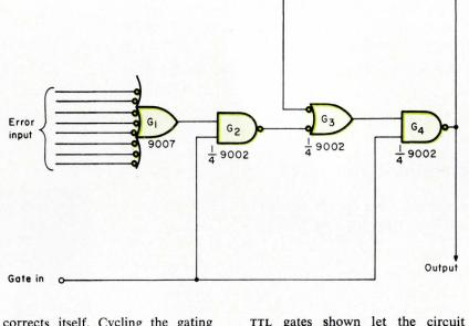
corrects itself. Cycling the gating signal to a logic 0 and back to logic 1 resets the circuit. The Fairchild TTL gates shown let the circuit latch on any error signal of 50 ns or longer.
