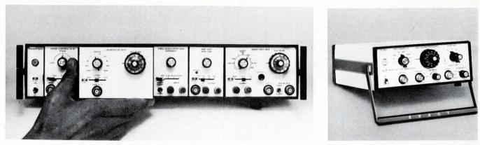
**Building-block waveform generator system** (Exact's 5000 Series) starts with a simple cabinet and power supply and lets you select its components. You can add, subtract or change functions to meet your needs. One square/triangle generator (G5210) and two ramp generators (G5212 and the second sec
