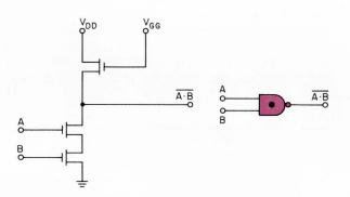
Fig. 3. The MOS NAND gate (dc) has two pull-down devices connected in series.
