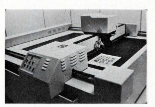
Computer-controlled drafting machine produces artwork at 100 times actual size.
