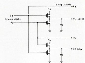
Fig. 6. This circuit located on the chip may be used to generate the two slow overlapping clocks, thus reducing the number of external clocks required.
