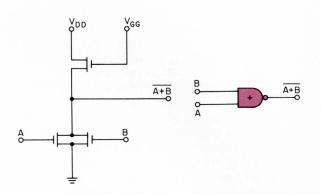
Fig. 2. The MOS NOR gate (dc) is similar to the inverter except that it has two pull-down devices in parallel.
