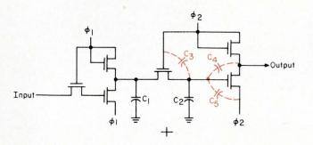
Fig. 11. This two-phase shift register shows the effect of parasitic coupling. A capacitor ratio of  $C_1 = 6C_2$  is commonly used and  $C_2 = 6(C_3 + C_4 + C_5)$  is a reasonably good approximation. First  $\phi_1$  precharges  $C_1$ , to a logic 1 (15 V) and then  $\phi_2$  shorts  $C_1$  and  $C_2$  together. Using the above capacitance values, when  $\phi_2$  returns to ground, the voltage left on  $C_2$  is about 10 V, which in many systems is the minimum input level.
