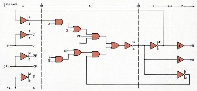
Fig. 9. Detailed logic and timing diagram for JK flip-flop.
