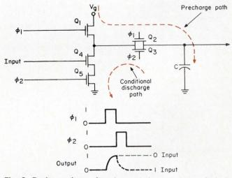
Fig. 2. Basic precharge inverter and the sequence of clock charging and conditionally discharging the output holding capacitor, depending on the input signal is shown.
