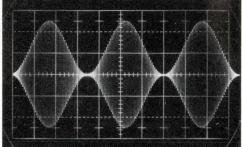
Sine wave amplitude modulation
