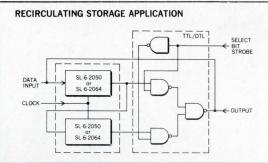
Among their various and marked advantages over bipolar and delay line serial storage systems, General Instrument's GIANT Dual 50-bit and Dual 64-bit DC shift registers operate with the lowest power dissipation available for static registers . . . a mere 7 milliamps typical.
