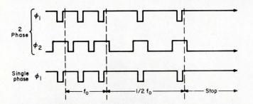
Fig. 8. Relative timing in single- and two-phase static systems. In the two-phase system,  $\phi_2$  must be a 1 while  $\phi_1$  must simply be returned to 0 to stop the register. In the two-phase system, the gap between  $\phi_1$  and  $\phi_2$  must be controlled. As the frequency changes, the pulse width of  $\phi_2$  must be changed. The single-phase system does this changing of  $\phi_2$  pulse width internally.
