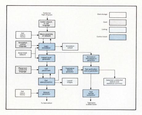
Flowchart for CAD subsystem design, test generation, simulation and artwork generation.
