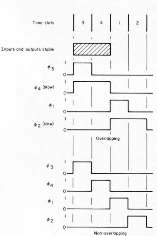
Fig. 5. The overlapping and non-overlapping four phase clocks are shown related to the four time slots. Note that the inputs and outputs of both types are stable during time slots 3 and 4. Thus, systems may have both types of clocks.
