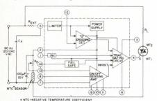
Functional block diagram of IC zerovoltage switch.
