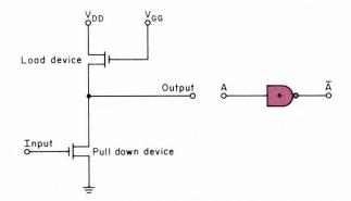
Fig. 1. The MOS inverter shown in schematic and logic diagram form. The node N is at or close to  $V_{\rm DD}$  if the pull-down device is off and is close to ground if the pull-down device is on.
