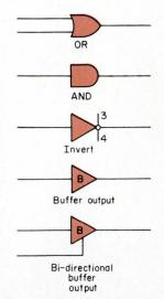
Fig. 8. The five basic logic elements are shown. The AND and OR gates are normally combined and fed into an inverter. The number 3 denotes the time slot in which the inverter precharge occurs and the number 4 at the bottom indicates that the conditional discharge occurs during the fourth time slot. The output is stable in time slots three and four.
