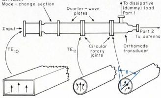
The proposed divider has four elements: a modechange section; two quarter-wave, rotatable plates; and an orthomode transducer. Input energy arrives at the divider via rectangular waveguide in the  $TE_{10}$  mode, which the circular mode-change section changes to  $TE_{11}$  mode. The first quarter-wave plate completes the change to  $TE_{11}$  circular polarization.
