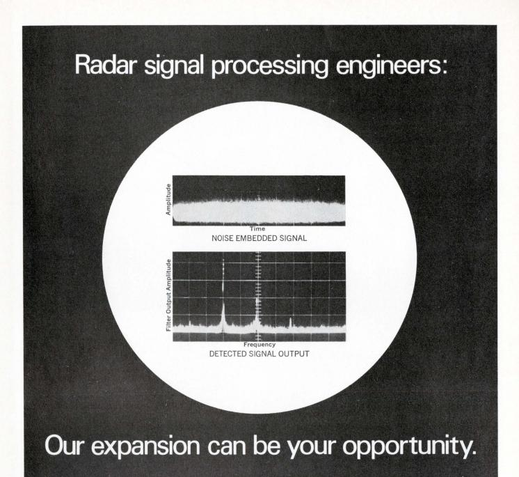
Today at Hughes, we're developing digital radar signal processors for a variety of important airborne applications. An engineering model of one of these processors has been developed for real-time operation. It uses the Cooley Tukey, or fast Fourier transform algorithm, to form a bank of 512 narrowband doppler filters, together with their associated detectors and threshold circuits.
