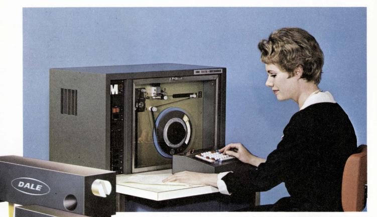
Mohawk Data-Recorders speed input preparation by transferring data direct from source document to computer-compatible magnetic tape. Dale Econo-Trims are used here to control gain in a number of amplifier circuits.
