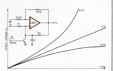
ous powers by adjusting the ratio of  $R_1$  to  $R_2$ . If  $R_1 = R_2$ , then k = 0 and the equation for  $e_0$  reduces (by l'Hospital's rule) to that of a linear sawtooth waveform:  $e_0 = 2e_i t/CR_1$ .
