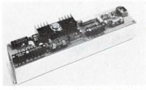
The PM796 consists of a 4.8 V to 6.3 V at 3 A logic power supply and a 180 V at 40 mA display power supply. Line and load reg. is  $\pm 0.05\%$  on the 5 V sub-assembly and  $\pm 0.5\%$  on the 180 V sub-assembly. Operating temp. range is 0° to 65°C and TC is 0.05% / °C. Computer Products, Inc., 2709 N. Dixie Hwy, Box 23849, Ft. Lauderdale, Fla. 33308.
