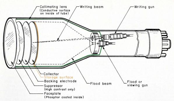
Fig. 1. Internal structure of a high-contrast display storage tube. By changing the voltage on the backing electrode you can control the number of electrons (from the flood gun) that reach the phosphor-coated faceplate. With a negative voltage level, the backing electrode prevents any electrons from passing through (cutoff), and the face of the tube is dark.
