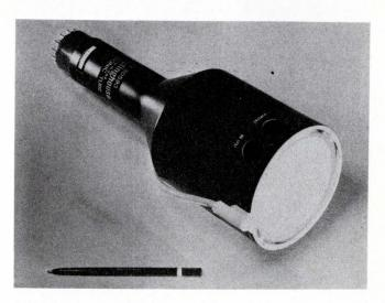
Fig. 6. The WX-30593 storage tube, made by Westinghouse Electronic Tube Div., Elmira, N. Y., can display both stored and nonstored information. Representative of the high contrast type described in the article, this tube has a writing speed of  $5 \times 10^5$  in./s and a resolution of 60 lines/in.
