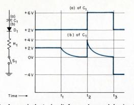
Fig. 2. An equivalent circuit for a storage tube is shown on the left. Plate (a) of  $C_1$  is the wire mesh of the backing electrode; the storage surface is the dielectric of  $C_1$ . Plate (b) represents flood electrons striking the storage surface.  $D_1$  shows that the electrons travel in one direction only and  $R_1$  is the impedance of the flood beam.
