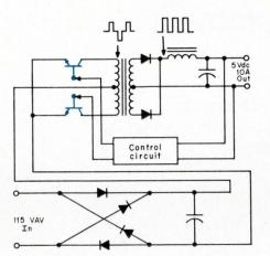
that would handle 300 V peak-to-peak and operate at these frequencies were not available. The electronically controlled transistors produce a pulse width corresponding to the desired output of the transformer. Loop response is faster than 1 ms.
