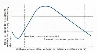
Fig. 3. A typical secondary emission curve for a dielectric material used in storage tubes. The curve shows that by bombarding the material with primary electrons at energies above first crossover you can raise the potential of the dielectric.
