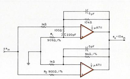
with dc levels, the circuit operates to beyond 5 MHz. Because the compensation circuit introduces a 1- $\mu$ s delay, waveform-area accuracy is 0.1% at 1 kHz, improving as the frequency decreases. The circuit as shown has a 10X gain. At gains lower than this, instability can develope because of phase shift in the amplifier. Capacitive loading should eliminate this difficulty, however.
