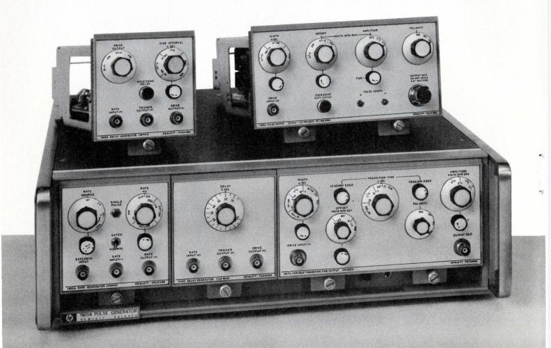
You can get 2- to 16-bit word lengths at a 0 to 50 MHz clock rate. A pseudo-random noise output and RZ and NRZ formats at the flick of a switch add to its capabilities. And, you are compatible with ECL, TTL, DTL, MOS, core memories or any other type of circuit you are testing.
