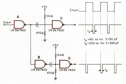
This causes a narrow output pulse. To drop enough voltage across the grounded resistors and thus guarantee threshold crossing, gates A and B should be TTL or similar low output-impedance devices.
