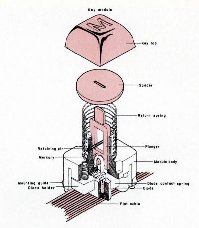
**Plug-in key modules** are the secret of the Mercutronic Coding Keyboard's versatility. Encoding diodes are built-in, and mercury switches give bounce-free switching. Standard typewriter keyboard configurations are available.
