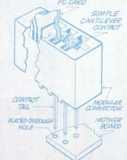
And, no, you don't give up a bit of connector reliability. The exclusive swaged single-beam design of the dual-readout contact provides optimum spring rate and deflection characteristics. A preload applied
