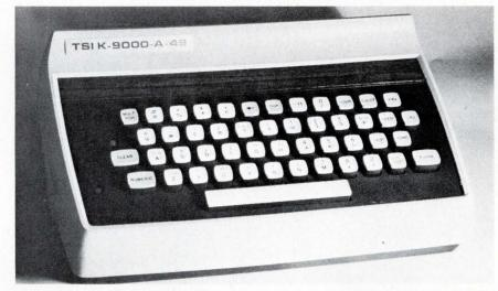
TSI's alphanumeric keyboards are solid state throughout, and offer bounce-free operation via the manufacturer's proximity key switch for data entry. Individually moveable and replaceable keys give you flexibility in use, and easy maintenance.
