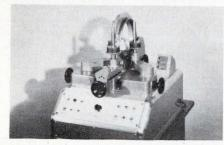
Open shuttle principle makes it possible to wind several toroids from a single load. The loading cycle, which on normal machines may require more time than the winding itself, is spread over several cores. Thus, it is practical to machine wind coils having relatively few turns. Coil Winding Equipment Co., Railroad Plaza, Oyster Bay, N.Y. 11771. Booths 3001 & 3101.
