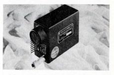
These modules provide high voltages for crt displays including storage tube and projection systems. Units are available with outputs from 1 kV to 30 kV. They are resin encapsulated which gives rugged construction and prevents voltage breakdown. Units can tolerate brief overloads and flashovers. Ekco Electronics Ltd., Southend-on-Sea, Essex, England. Booths 4614-15.
