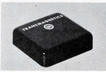
This SS converter can replace gear train servos in many applications. Model 1637 converts a three wire synchro input to a linear dc output proportional to the synchro angle. It is 2.6 in.<sup>3</sup> and sells for under \$100 in quantities of 1000 or more. Transmagnetics, Inc., 134-25 Northern Blvd., Flushing, N. Y. 11354. Booth 4180.
