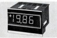
Model 4304, with four digits for a display to 1999, features small size and large up-front display. A to D conversion is done by dual slope in-tegration. Display can be read from 40 ft at angles to 140° without parallax or tunnel effects. Accuracy is 0.1% and res. 1 part in 4000. API Instruments Co., Chesterland, Ohio 44026. Booths 1404-05.
