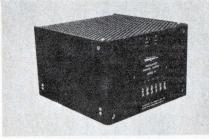
"N" Series modules with IC regulation system provide an effective system for minimizing load and line in-duced thermal drift. It has 0.005% reg., adj. current limiting, convection cooling to 71°C and electrostatically shielded transformers. Deltron Inc., Wissahickon Ave., North Wales, Pa. 19454. Booth 1508.
