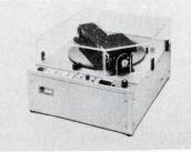
IDR 100 instrumentation recorder uses a 12 in. disc rotating at 1800 rpm to record analog signals from 400 Hz to 2 MHz. Primarily for recording and analyzing transient signals, it has a spiral 0.004 in. track with 0.001 in. guardband and 20 s of cont. record/ playback. Data Memory, Inc., 1255 Terra Bella Ave., Mt. View, Calif. 94040. Booths 5306-07.
