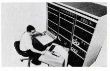
Medium scale PDP-15/20 is one of four configurations in which the 18bit computer is being offered. Some features included are 8,192 words of core memory; a KSR35 teletype; two mag tape units; a high speed paper tape reader and punch; and advanced monitor software. Digital Equipment Corp., Maynard, Mass. 01754. Booths 5620, 21, 22, 23.
