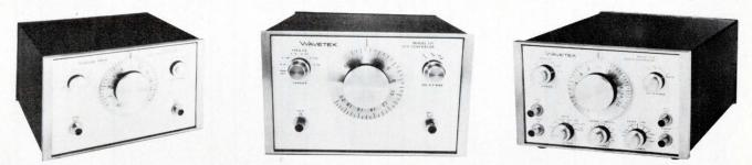
Wavetek's new line of function generators. Basic Model 130 (left) has six frequency ranges covering from 0.2 Hz to 2 MHz; output voltage of 20 V pk-pk into an open circuit, 10 V pk-pk into a 50 $\Omega$  load; dial accuracy of  $\pm 2\%$  of full scale; maximum sinusoidal distortion of 5% (26 dB down from fundamental). Price: \$295. Model 131VCG (center) can be driven by an external ramp to sweep its frequency range,
