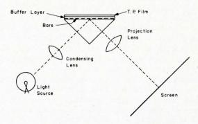
Fig. 4: The GE thermoplastic film projection system is similar in idea to the Eidophor system.
