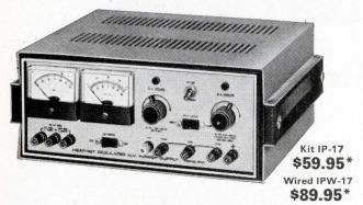
Heathkit IP-17 Variable Regulated High Voltage Power Supply will deliver 0 to 400 VDC with better than 1% regulation at current loads up to 100 mA, 0 to -100 V bias at 1 mA max., and both 6 and 12 VAC at 4 A and 2 A respectively or any combination to a maximum of 25 VA load. Separate panel meters monitor B+ output voltage and current. High voltage and bias may be switched "off" with heater voltage still "on" for maximum efficiency in testing and for safety. Ripple is less than 10 mV.
