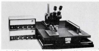
A visible tooling template gives fast positioning of the circuit board (to 8 x 8 in.) under the soldering head. There is a magnetic transfer system for placement. Dual power supplies. \$4900. Development Associates Controls, 725 Reddick Ave., Santa Barbara, Calif. 93103.
