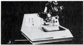
Model 8-151-01 has manual search control for multilevel bonding, adjustable wire looping, and a micromanipulator (x, y, and rotation). Patented bonding mechanism assures flat tool delivery. \$3400 fob. Unitek, Weldmatic Div., 950 Royal Oaks Dr., Monrovia, Calif. 91016. Circle 202 on Inquiry Card
