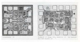
These ICs have active elements protected by a "tub" of silicon dioxide, and interconnected with tantalum thin-film resistors. The five DTL circuits are the 930, 932, 944, 945, and 962. Philco-Ford Corp., Microelectronics Div., Blue Bell, Pa. 19422.
