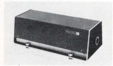
Model 610 is for use where a highpower, cw, 1.06-micrometer source is needed. It emits >1 W in the TEM<sub>oo</sub> mode and >5 W in multi-transverse mode operation. Optical length of the cavity is about 38 cm. Output beam dia. is 3 mm. Sylvania Electronic Systems-Western Div., Electro-Optics Orgn., Box 188, Mountain View, Calif. 94040. (415) 966-2312
