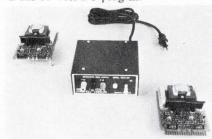
Model SEI-15/15-100 is an all silicon SS device. Basic unit provides 100 mA on each output; is short circuit proof; has 1-mV pk-pk ripple voltage; and is regulated to  $\pm 0.01\%$  line, 105 to 125 Vac 60 Hz, and  $\pm 0.02\%$  load, no load to full load. Salient Electronics, Inc., Blue Barns Rd., Rexford. N. Y. 12148. (518) 393-4590.
