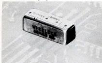
Series 442S 5-V relays require about 60 mW per pole to operate. They occupy only 0.05 in<sup>3</sup>/pole, and are only 0.258 in. high. Available in 1- to 4pole models with contacts rated at a full 7 W, they weigh 1.9 g/pole. Operating temp. range is  $-65^{\circ}$  to  $+85^{\circ}$ C. Wheelock Signals, Inc., 273 Branchport Ave., Long Branch, N. J. 07740. (201) 222-6880. Circle 237 on Inquiry Card
