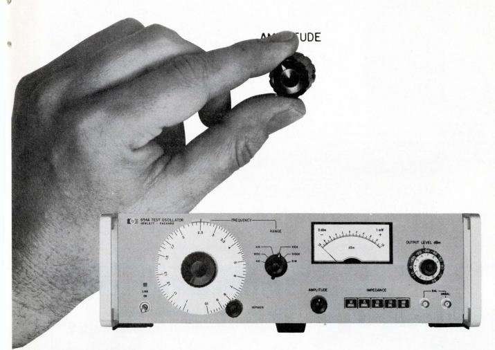
With the HP 654A Test Oscillator you don't have to adjust the output when you change frequencies. The automatically controlled 0.5% level flatness across the entire frequency range of 10 Hz to 10 MHz eliminates repetitive output level adjustments. And, with your system input automatically controlled, you are free to concentrate on system performance measurements.
