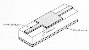
Fig. 3: Stripline method for achieving the rf short. The center conductor's width is increased and the rf short is essentially the capacitance between the center conductor and the outer conductor (ground plane). In this approach, due to the large separation between plates (typically 0.0625 or 0.125 in.) and the dielectric material's low dielectric constant (2.5-3.0), the capacitance attainable is small.
