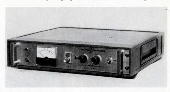
Model PR-101 analyzer measures dielectric constant and loss factor of sample materials that have an E of 26 or less. Accuracies are better than 2% absolute and 0.2% relative. Direct-reading output. Pacific Radionics, 581 Division St., Campbell, Calif. 95008.
