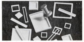
For packaging ICs, resistor networks, etc. frame portions can be as narrow as 0.02 in., with 0.01 in.-thick material. High strength. Pre-glassed edges available. Can be silk-screened. Custom manufactured (2-3 wks.). Cermetron Corp., 10475 Roselle, San Diego, Calif. 92121.
