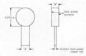
Fig. 5: Discrete rf termination electrically and mechanically matches the stripline. Typical dimensions are A=0.080 in. and B=0.125 in.
