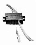
Weight and volume savings rendered by terminal junctions (when compared with terminal strips) become appreciable as the wire becomes finer. The protective grommet's sealing action on the terminal junction (right) eliminates the contamination and shorting hazards of the exposed terminals. Terminal junctions on relay offer fast connection and environmental protection. It is the first step towards an integrated termination system. (Photo courtesy of Deutsch-Filtors.)
