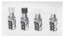
Snap-action switches have DPDT action enclosed in a miniature case, but separate connections to the lamp can still be made. Standard T-13/4 grooved lamps are replaceable from the front without tools. Alco Electronic Products, Inc., Box 1348, Lawrence, Mass. 01845 (617) 686-3887.
