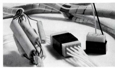
Terminal junction modules provide feedback or a feedthru capability for terminating wires; splices are also available. (Photo courtesy of AMP, Inc.)
