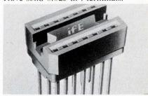
These 14-lead sockets have large tapered entry channels for quick lead insertion into dual leaf contacts. Polysulfone body provides anti-rotate pockets for hex nuts for easy assembly to the chassis. Contacts are beryllium copper with std. gold and tin contact plating. Plastic Mold and Engineering Co., 265 Wampanoag Trail, Box 4265, East Providence, R. I. 02914.
