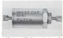
Miniature CF filter series is available in the working voltage range of 50 to 200 Vdc and 0.06 to 15 A. Hermetically sealed steel case is 0.560 x 0.375 in. Operating temp. is  $-55^{\circ}$  to  $+125^{\circ}$ C. Plating is gold, silver, or tin with various mounting styles available. San Fernando Electric Mfg. Co., 1501 First St., San Fernando, Calif. 91341. (213) 365-9411.
