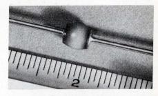
This is one of the new 3-A rectifiers showing the "Metoxilite" encapsulation prior to painting and marking. It is 0.165 in. long and 0.180 in. at the widest point.
