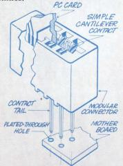
And, no, you don't give up a bit of connector reliability. The exclusive swaged single-beam design of the dual-readout contact provides optimum spring rate and deflection characteristics. A preload applied
