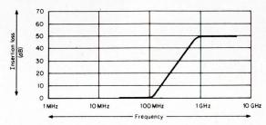
Fig. 10: Typical insertion loss curve of filter/bias capacitor network.
