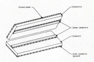
termed "microstrip"—essentially one-half of the stripline. Microstrip is the basic building block for what is often referred to as "MIC's" or Microwave Integrated Circuits (thin-film hybrids, thick-film hybrids, or monolithic integrated circuits).
