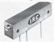
Type 60 has many features of the more expensive MIL types. It meets MIL Std. 202 tests for load life, humidity, shock, and vibration. It has a res. range from 10  $\Omega$  to 50 k $\Omega$ ; tol. is  $\pm 10\%$  with a power rating of 1 W at 70°C, derated to 0 at 125°C; temp. range is -55° to +125°C. IRC Div., TRW Inc., 2801 72nd St., N., St. Petersburg, Fla. 33733.
