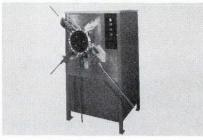
Type 852 sorter, operating with suitable test equipment, automatically tests and sorts over 5000 DIL ICs/h, magazine to magazine. Devices fed from the magazine are transferred to an index table, then advanced to a probe station for dc or dynamic testing. Daymarc Corp., 40 Bear Hill Rd., Waltham, Mass. 02154. (617) 894-2105.
