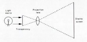
Fig. 2: A very basic display technique is the projection of a photographic transparency. This is a 2D system for non-real-time data.
