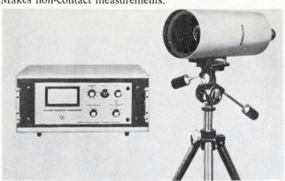
This infrared thermometer can measure the temperature of objects both near and far. It will also monitor fast-moving objects, or transient heat phenomena as short as 3 ms (55 Hz). Total temperature range is from  $-20^{\circ}$  to  $3200^{\circ}$ C, in four overlapping ranges. Sensitivity at  $20^{\circ}$ C is  $0.5^{\circ}$ C; absolue accuracy is  $\pm 1\%$  o.f.s.
