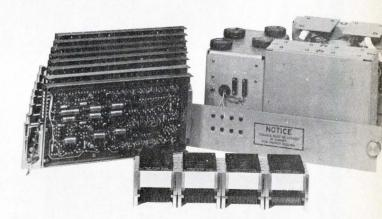
Fig. 5. Packaging evolution of an electronic subsystem. At the upper right is the initial design, while at the upper left it's seen redesigned into transistor page-card modules. The foreground unit shows its final repackaging into Standard Hardware Program modules by NAFI engineers.
