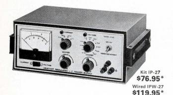
Heathkit IP-27 Solid-State Regulated Low Voltage Power Supply features Zener reference voltage, immunity to transients and protection against short circuit and overload. The IP-27 will supply 0.5 to 50 V with better than 15 mV regulation under current loads ranging from 0 to 1.5 A. Current can be limited from 30 to 100% on each of four ranges from 50 mA to 1.5 A as a safety factor. Panel meter shows output voltage or current. Ripple is less than 150 microvolts.
