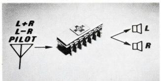
The monolithic MC1304 separates left and right audio, activates a stereo-indicator lamp, mutes interstation hiss, and automatically converts weak stereo to monaural signals. \$4.80, 100-up. Technical Information Center, Motorola Semiconductor, Box 20924, Phoenix, Ariz. 85036.
