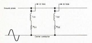
Fig. 7: Diodes D1 and D2 are represented by the series inductance and series resistance. The inductive reactance ( $X_{\rm LD1}$  and  $X_{\rm LD2}$ ) increase with increasing frequency and result in a high impedance path to ground, rather than in a short circuit. The circuit which overcomes this problem is shown in Fig. 8.
