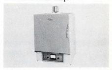
New LST (Low Skin Temperature) ovens have a safe ext. temp. of  $<50^{\circ}$ C even when operating at 300°C. The ovens provide over 5 ft³ of load area in a stainless steel chamber. The Temp. range is from 40° to 350°C. Electronic control is accurate to within  $\pm 0.15\%$ . Hotpack Corp., 5137 Cottman Ave., Philadelphia Pa. 19135. (215) 333-1700.
