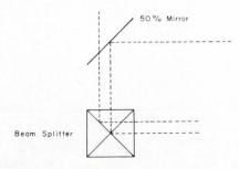
Fig. 9: With the addition of 50% mirrors the arrangement in Fig. 8 can be used to project six overlay images.
