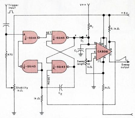
If you set the stability control so that input A is above the gate threshold, the circuit free-runs. It gives you a continuous train of sweep pulses, each with a period equal to the sweep time plus the hold-off interval.
