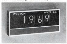
DPM 1290 specs include threedigit plus 100% overrange display, 0.1% ±1 digit accuracy, 1-2-4-8 BCD positive output logic, and plug-in readouts. Less than \$200, 100-pc. lots. Weston Instr., 614 Frelinghuysen Ave., Newark, N. J. 07114.
