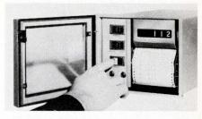
Input voltages, 0-1, 0-10, 0-50 mV. Three-digit print-out, plus two spaces for channel call-out, four for time, three more for external data. Options available. Model DL-1210, \$1575. Entex, Box 770, Friendswood, Tex. 77546.
