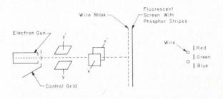
Fig. 12: The Lawrence color tube uses a single gun and deflection system. A potential on the wires in the grid determine which color is activated.
