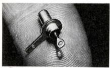
Metal diodes protect elements in applications where fast firing, low leakage current, and relatively low firing voltage are needed. Inherent firing voltage is 80 to 89 V. While the puncture voltage of Mos-Fets is generally lower than 85 V, this 85-V diode protects lower puncture voltages by appropriate biasing of the diodes. Victoreen Instrument Div., 10101 Woodland Ave., Cleveland, Ohio 44104.
