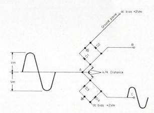
Fig. 6: Simple parallel diode switch. D1 and D2 in leg AB are forward biased and will conduct. Ideally, in this state, they will short any signal in leg AB to ground. D3 and D4, on the other hand, are reverse biased and, as such, will not conduct. In this state D3 and D4 are ideally an open circuit, and the signal will be transmitted through leg AC.
