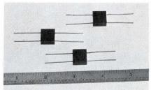
New 2-A single phase, full wave rectifier bridge features controlled avalanche and reverse recoveries from 50 to 400 ns. Each leg of the bridge has a double glass seal for hermeticity. Available in mechanical form factors for PC boards, cordwood, and other mountings. MicroSemiconductor Corp., 11250 Playa Court, Culver City, Calif. 90230. (213) 391-8271. Circle 280 on Inquiry Card
