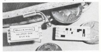
Series 809 (positive output), Series 859 (neg.) have fixed outputs from 5-28 V. Load regulation, 0.003%/mA. Ripple attenuation, 34 dB. I/O differential, 2 V min. \$13.50 ea. Tech. Info. Sect., Helipot Div., Beckman Instr., 2500 Harbor Blvd., Fullerton, Calif. 92634.
