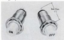
New line of miniature switches are 11/2 in. from the front of the panel to the rear of the contacts. They come in momentary action up to SPDT and operate with either 115 Vac or 30 Vdc at 1 A res. or ½ A ind. Lens take either a std. T1¾ or ALC-100 neon bulb. Electro-Mech Components Inc., 1039 East Valley Blvd., San Gabriel, Calif. 91776. (213) 283-9213.
