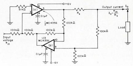
current and governs the output voltage of amplifier (a) for regulation. Output-current linearity vs input control voltage is good, with errors of less than 1%. Frequency response is limited to that of the open-
