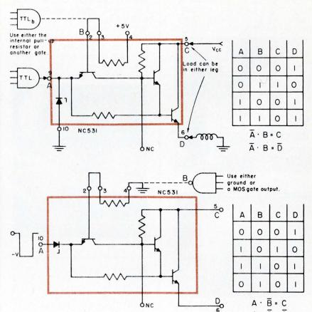
the zener provides the necessary logic levels (noise immunity): logic  $0, \le 6 \text{ V}$ ; logic  $1, \ge 6.5 \text{ V}$ .
