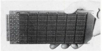
Socket cards hold 24 (4.5 in. sq. unit) or 64 IC sockets 4.5 x 9.25 in.). \$46.50 to \$100.40 ea., 10-24 pcs. Card files are assembled for automatic or hand wiring. The 19-in. file holds 728 ICs. \$48.80 to \$177 ea., 10-24 pcs. CTC, 445 Concord Ave., Cambridge, Mass. 02138.
