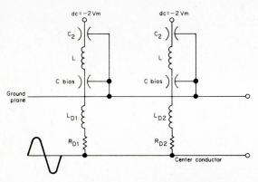
Fig. 8: This circuit overcomes the problems found in the circuit of Fig. 7. The capacitor ( $C_{\rm Blas}$ ) resonates with the self-inductance of the diode at the transmitting frequency, resulting in an effective rf resistance. A low impedance path now exists between the center conductor and ground.
