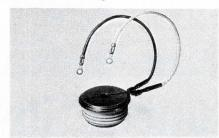
Type 282, "Full Capacity" thyristor is to replace parallel SCRS. Because of the all-diffused design, the thyristor's full inherent capacity is realized. Characteristics include a guaranteed dv/dt, low thermal imp., high surge current capability (to 7000 A), and high transient voltage capability. Westinghouse Semiconductor Div., Youngwood, Pa. 15697. (412) 255-3693.
