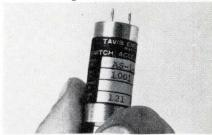
Model AS-1 instantaneous acceleration switch is for use with 12- to 40-Vdc supplies. It combines a basic inertial element with integral SS logic circuitry. Circuits are opened or closed within 1 ms, when peak acceleration exceeds the set point. Tavis Engineering Co., Bootjack Rd., Mariposa, Calif. 95338.
