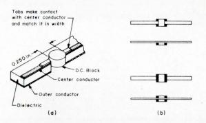
Fig. 2: Discrete passive device (dc block) mounted on stripline (left). This type device has soft copper tabs which match the stripline's center conductor. The tabs can be either soldered or spot welded. Low inductance is inherent in the design and the insertion loss is typically 0.25 dB max. from 0.5 to 4 GHz. VSWR is typically 1.1:1 up to 4 GHz. Discrete devices for microstrip dc blocks (right).
