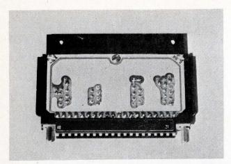
Fig. 1. The basic module configuration in the Navy's Standard Hardware Program is the single-span, single-thickness (1A) module. The functions of the 225 modules in the SHP span both linear and digital applications. Of this number, 87 are Standard modules of which 60 are already documented, qualified (or in process of being qualified), and multi-sourced. The remaining 138 modules are Specials, carried temporarily for information purposes, and aren't representative of the program's objectives.
