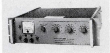
Model 1579 furnishes stable, low noise corona-free voltages between 10 kV and 30 kV. Specs include: Max. out. curr. of 1 mA; 0.0025% reg. for line or load variations;  $< 250$  mV ripple pk-to-pk; output volt. drift  $< 100$  ppm/h and 300 ppm/24 h; and repeatability of 100 ppm. Power Design, Inc., 1700 Shames Dr., Westbury, N. Y. 11590. (516) ED 3-6200. Booths 2G10-11.
