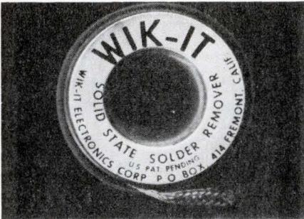
Wik-It desoldering tool is specially-treated (with Mil Spec chemicals) tinned braid that quickly draws up solder when heat is applied with an ordinary soldering iron. It acts as a heat sink to protect delicate components, and leaves the joint resolder-ready. It cuts costs of equipment down-time, rework, trouble shooting, quality control and prototype building. It is sold as service kit or spool rolls; a sample is available on request. Wik-It Electronics Corp., Box 414, Fremont, Calif. 94537.
