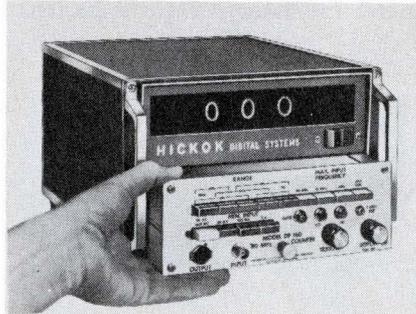
Here are five more plug-ins for the DMS 3200 digital measuring system. The DP 110 and DP 130 measure, respectively, dc and ac microvolts to kilovolts. The D 310, when used with the DP 110, measures nanoamperes to amperes. The DP 160 is an 80-MHz frequency counter, and the DP 210 shows interval/period from 10  $\mu$ s to 999 s. Hickok Electrical Instr. Booths 2C18-20, 2C25-27.
