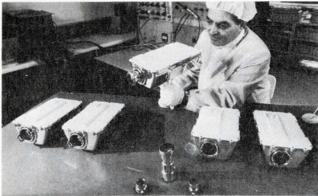
rendition without breakup at the slow speeds at which the astronauts will move. This scan rate can be easily converted to 60 fps for viewing on home TV receivers. A 320-line scan was chosen to obtain nearly equal vertical and horizontal resolution. The 10 fps mode will provide about 250 discernible lines on a home TV set, good enough for viewing.
