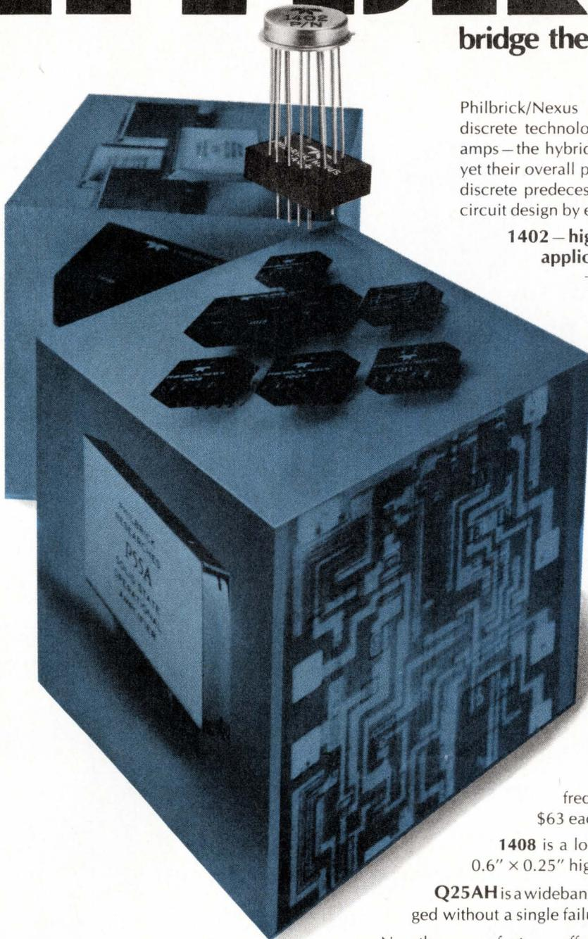
Philbrick/Nexus combines the best of monolithic and discrete technologies to create the now generation of op amps—the hybrids. They're micro-miniature and low cost, yet their overall performance is equal to or better than their discrete predecessors. And, built-in stabilization simplifies circuit design by eliminating external components.
