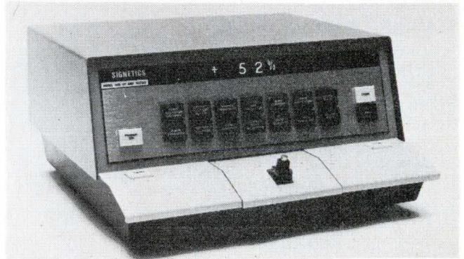
Model 1410 is primarily an op amp tester for pre-production testing: it is automatic and simple to program and operate. Its three modes of operation tell the operator what tests are programmed for pass/fail indication, whether a unit passed or failed, and how well that unit passed or failed as a percentage relative to the programmed limit for that test.
