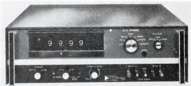
This automatic-ranging digital voltmeter has a sample rate of 10 samples/s, 10  $\mu$ V sensitivity, with a readout accuracy of 0.01% over its five dc ranges. The display neither blinks nor has running numbers.
