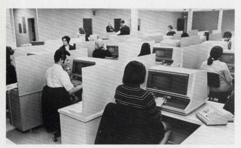
Operators of UNISCOPE terminals at National Data Corp.'s Cherry Hill, N.J., center receive telephone calls to verify credit cards from gasoline stations and department stores throughout the Northeast United States. Normally, an answer verifying if the card is "good" is received within 20 seconds from the computer.
