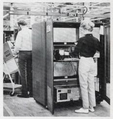
General Electric's new DATANET-500<sup>tm</sup> data communication processors undergo final tests prior to shipment. The new system combines all technological breakthroughs in communications and computer design over the past several years. GE computer experts predict the new processor can save up to 70 percent in communication line costs for large nationwide computer networks. It can serve up to 250 communications lines at the same time and can accommodate 500 to 1,500 users.
