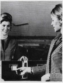
Help for Jet-Age Joe . . . Automatic computer-aided passenger check-in devices for air travelers are being developed by Sperry Rand Corporation's Univac Division to ease crowded conditions at terminals as air travel triples in the 1970's. The self-service devices include credit card verifier, left, and ticket encoder, right. Automatic passenger processing systems may also include talking computers, which would provide flight schedules, reservations service, and flight status reports.
