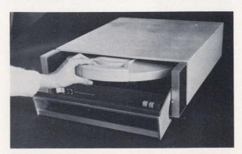
A Front Loader. Diablo's Model 31 with one 2315-type front loading cartridge.
