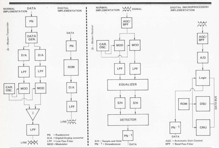
Fig. 3 – The Methods Compared. 3a shows block diagrams of a modem transmitter, nondigitally and digitally implemented. 3b shows block diagrams of a modem receiver, also nondigitally and digitally (with microprocessor) implemented. Programming the ROM for different modulation and filtering schemes gives the modems great flexibility.
