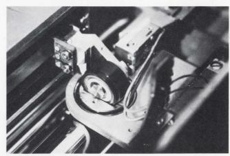
Diablo's head positioner. Shown is one of two head positioning mechanisms; one inertial actuator can independently move two head positioners per disk drive.
