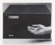
Four-Phase Systems' new NP/80 Network Processor. The heart of the NP/80 is a powerful 16-bit computer with 500 nanosecond cycle time and up to 256K bytes of MOS/LSI memory. The hand in the foreground contains all the 16K-bit RAM chips needed for a 256K byte memory including error correction. These devices, designed and manufactured by Four-Phase, will occupy a single printed circuit board when assembled.
