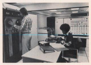
First Ryad Computer In U.S. ES 1040 computer system and East European peripheral devices are shown above in CDC's Capital Facility in Washington, DC. At left are two Robotron-built single-density 75-ips tape drives. At rear center are two Bulgarian built 7.25-Mbyte disk drives with German Democratic Republic controller. Operator's console of computer system manufactured in East Germany is at right.
