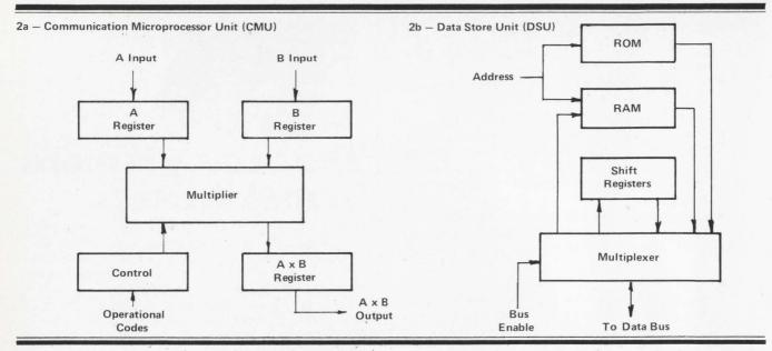
Fig. 2 - Block diagram (a) shows the CMU chip organized for fast multiplication, and (b), the DSU with its three types of data storage.
