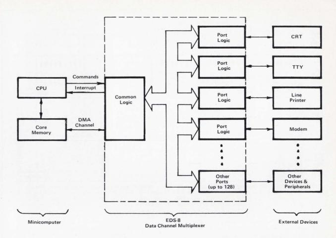
Fig. 2 - Block Diagram of EDS-8 Data Channel Multiplexer
