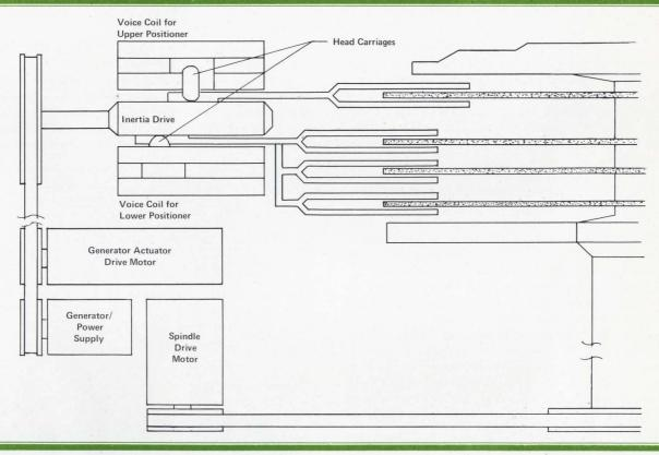
Two Independent Positioners. Both ride on the same driveshaft. One is used for the fixed disks; one is used for the removable disk.
