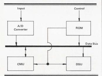
Fig. 1 — High-Speed Communication Microcomputer. The heart of the modem receiver is the CMU/DSU microprocessor with the control ROM as the brains. A small amount of additional logic routes data from data bus to customer's equipment.
