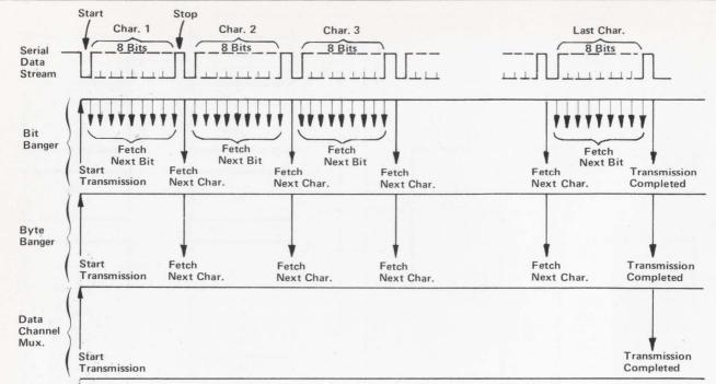
FROM BIT BANGER TO CHANNEL MUX. The Bit Banger was primarily, a software multiplexing technique, with the hardware limited to a flip-flop for each channel plus some common logic. This mechanization required an interrupt every bit time, at which time software routines determined whether the last bit output was the last bit of a byte. If not, the next bit would be fetched, the computer would again be interrupted, and the determination made again.
