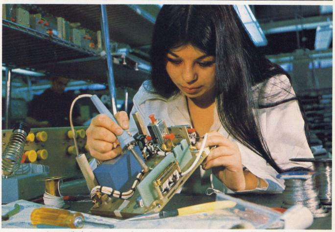
Technician Elizabeth Garcia wires the front panel of a chassis assembly produced by GTE Sylvania.
