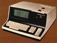
remote batch applications through utilization of card reader, magnetic tape, and printer peripherals. In software, Datapoint provides a CTOS operating system, Assembly Language, and the new DATAFORM language for sophisticated data entry and editing. Initial deliveries of the 1100, with a monthly lease price of \$138, will begin in January.
