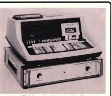
Fluidyne Instrumentation's 7200 series interface with Wang 600 series calculator.
