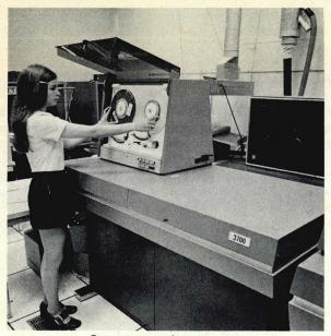
Operator mounting tape on a Pertec Model 3700 COM recorder.
