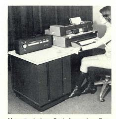
Magnetic Ledger Card Accounting Computer. The Litton/ABS Model 1281 can process letter-sized ledger cards containing 1199 digits per side. Data is maintained on a magnetic stripe positioned at the edge of each card side, with remaining space utilized for account or record printout.
