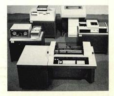
Accounting Computer/Small Business Computer. The NCR 399 straddles the dividing line separating an accounting computer from a disc-based small business computer. The unit record oriented 399 offers a complete range of magnetic ledger card, line printer, tape and card options, and can come with auxiliary disc ''platter'' storage.
