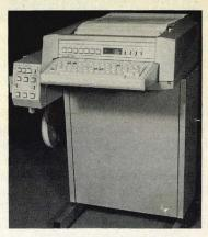
GE TermiNet 300 Teleprinter in pedestal mount
