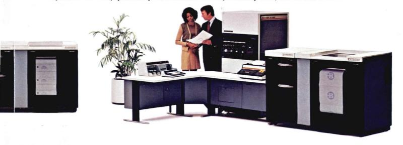
B 1700 SYSTEMS satisfy business management requirements and can serve engineering and production, as well. Like Burroughs larger scale computers, the B 1700 Systems operate on multiple data processing jobs at the same time. Their advanced features include "virtual memory" operation for high system efficiency, and a Master Control Program for system self-management.
