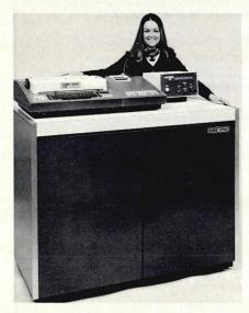
Fig. 3 — The Cope 4705, a communications controller marketed by Harris Communication Systems as a direct replacement for the IBM 270X and 370X transmission control units, which supports a variety of I/O devices and communications facilities.
