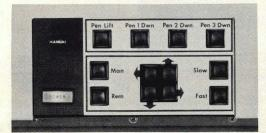
Simple push buttons control paper, pen and power; low paper supply and low vacuum shown by indicator lights.
