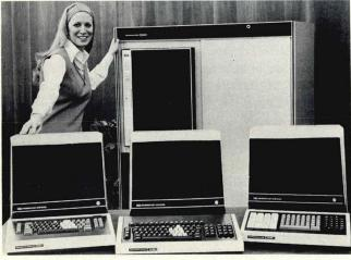
Fig. 1 — The GTE IS/7800 Series of intelligent CRT terminals, replacements, and enhancements for the IBM 3270 series, includes local and remote cluster units, stand-alone terminals, and terminal systems oriented to special inquiry/response applications (brokerage quotations, airlines reservations, etc.).
