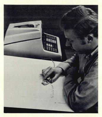
Figure 1 • Hand-held, manual cursor of Hewlett-Packard digitizer used to feed coordinates to H-P calculator for analysis.
