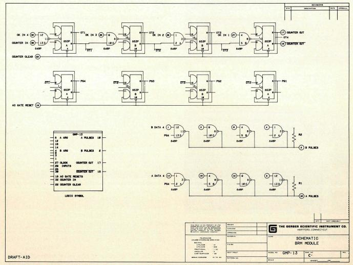
Figure 4 • A camera-ready logic drawing which took two hours to prepare using a digitizer and plotter, versus an estimated seven hours using manual methods (courtesy of Gerber Scientific).
