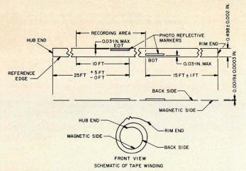
Figure 4 • Tape Markers, Recording Area, and Tape Wind (courtesy of USAI)
