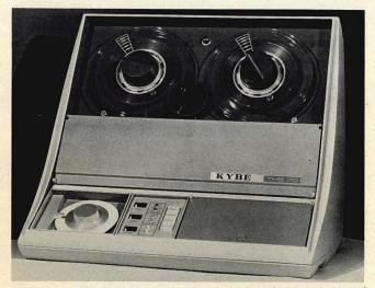
Figure 6 • The TMS-70 magnetic tape tester-cleaner, designed by Kybe for small- to medium-size tape-oriented computer installation.
