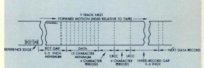
Figure 2 • 9-Track NRZI Format (courtesy of Peripheral Equipment)
