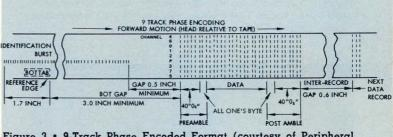
Figure 3 • 9-Track Phase Encoded Format (courtesy of Peripheral Equipment)
