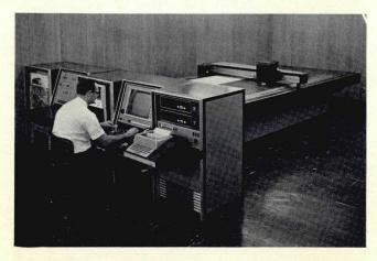
Figure 2 • Actron Industries/Tridea Products Division's ALTAPE/ALDRAFT Systems, an automatic line-following graphic digitizer/plotter system.
