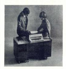
Teletype 4210 magnetic tape data terminal with 37 keyboard send-receive set.
