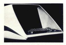
any point on the screen with only three commands. A built-in interface allows the DECterminal I to drive multiple TV monitors; it also has a video mixing capability allowing variable background pictures to be projected simultaneously on the screen. Price, in quantities of 100, is \$1,995, with first deliveries this summer. Digital Equipment, Maynard, Mass.
