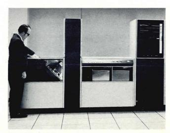
The 20/20 OCR System of Scan Optics, a page/document reader capable of reading a wide variety of fonts and handprint, and 30 lines of 60 characters at 50 pages per minute.
