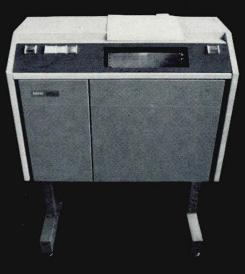
The Vogue/Shepard 880E Printer combination of ink roller reliability and patented, drum-impact, ballistic hammers to produce six clear copies of data. Five more copies than you get with non-impact printers. At no extra cost.
