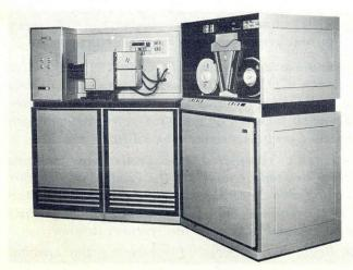
UCC-Graphic Systems Division Model 300-3 microfilm printer/plotter with companion tape drive.
