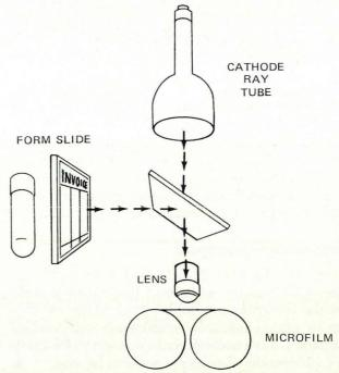
Fig. 1 CRT Recording on Microfilm
