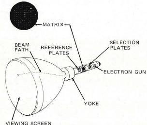
Fig. 4 Use of a Stencil-Type Wafer
