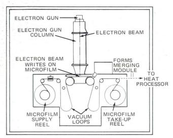
Fig. 2 Electron Beam Recording on Microfilm
