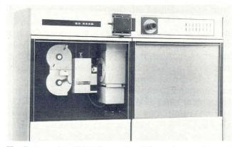
The Datagraphix 4440 Micromation Printer shown with the F230 Universal camera exposed.
