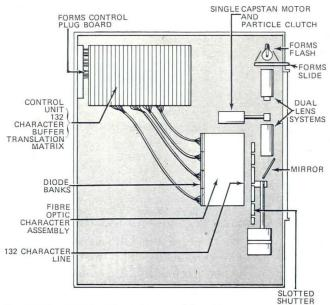
Fig. 3 Fiber Optics Recording on Microfilm
